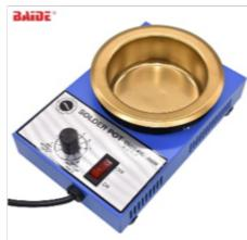
The ends of control cables will require a certain type of nipple to be soldered on. Because more than just capillary filling of solder is required, a soldering bath is a must have to ensure sufficient solder can attach to the cable end and nipple before it cools off too much.
