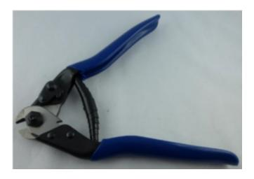
To cut the inner and outer cables you need a proper sit of shearing cutters specifically for steel cable. If you use a pair of nail pliers you will squash the inner cable and fray it; you'll simply crush the outer cable. Shearing cutters have a cutting area that encloses the to be cut item, so don't crush or squash. Here's an example:
