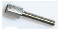
After measuring the brake hub, we find the required take on is quite small on the output side. The input side will take the M6 distancer.
