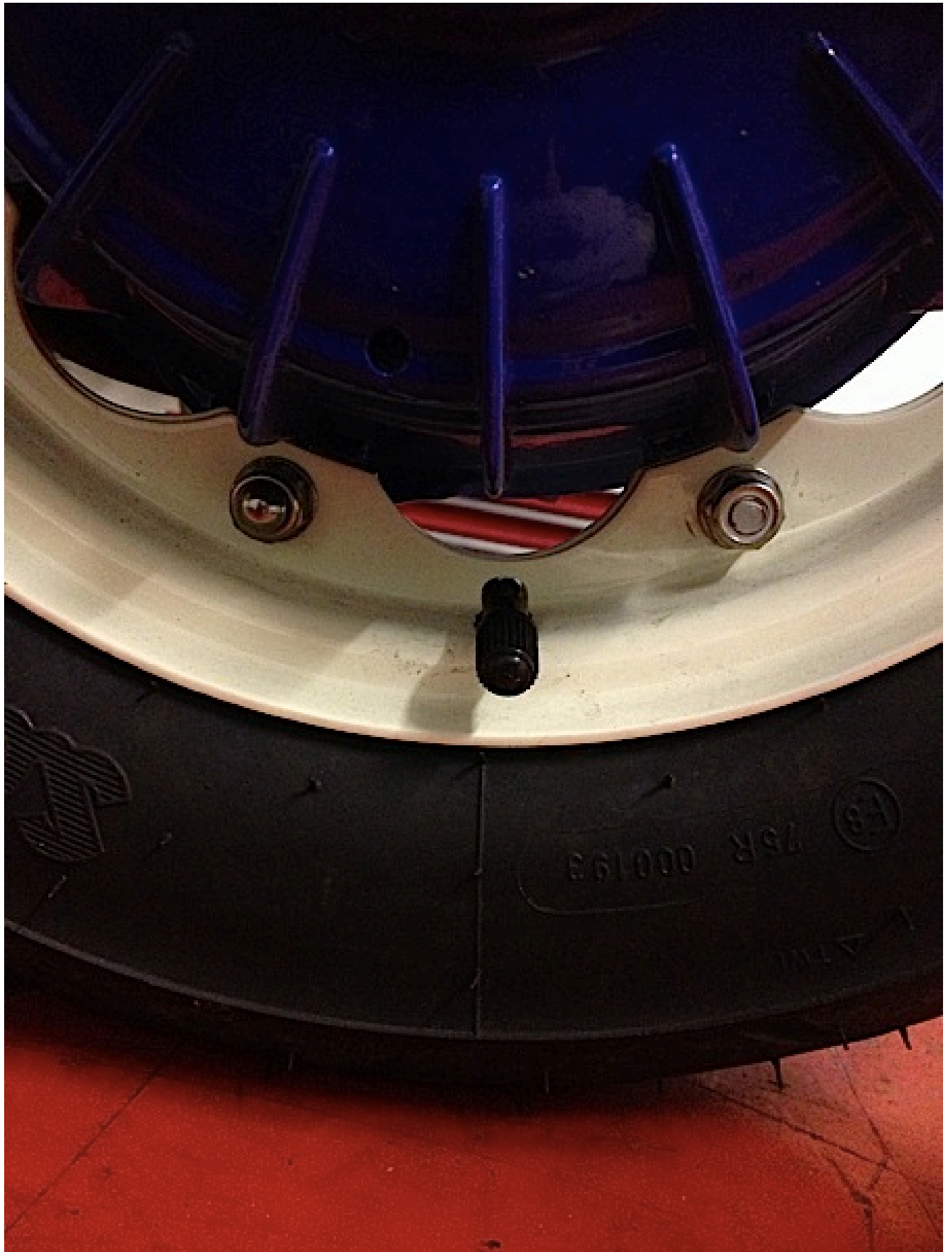
Holes in rims can effect valve positioning, this is center between the studs but is direct towards the rear hub fin, some valves can be touching the fin
