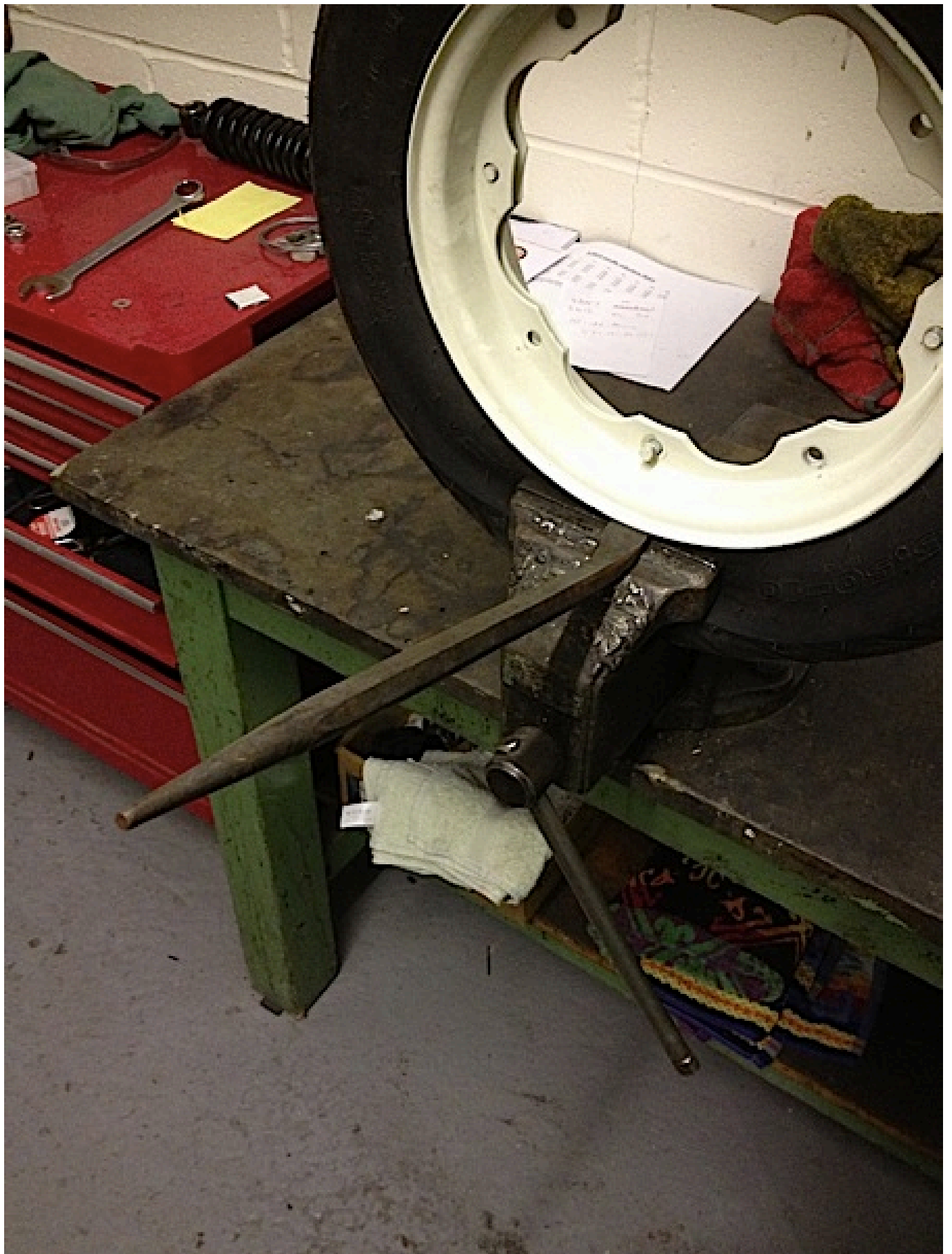
Hook a lever underneath to prize off the rim
