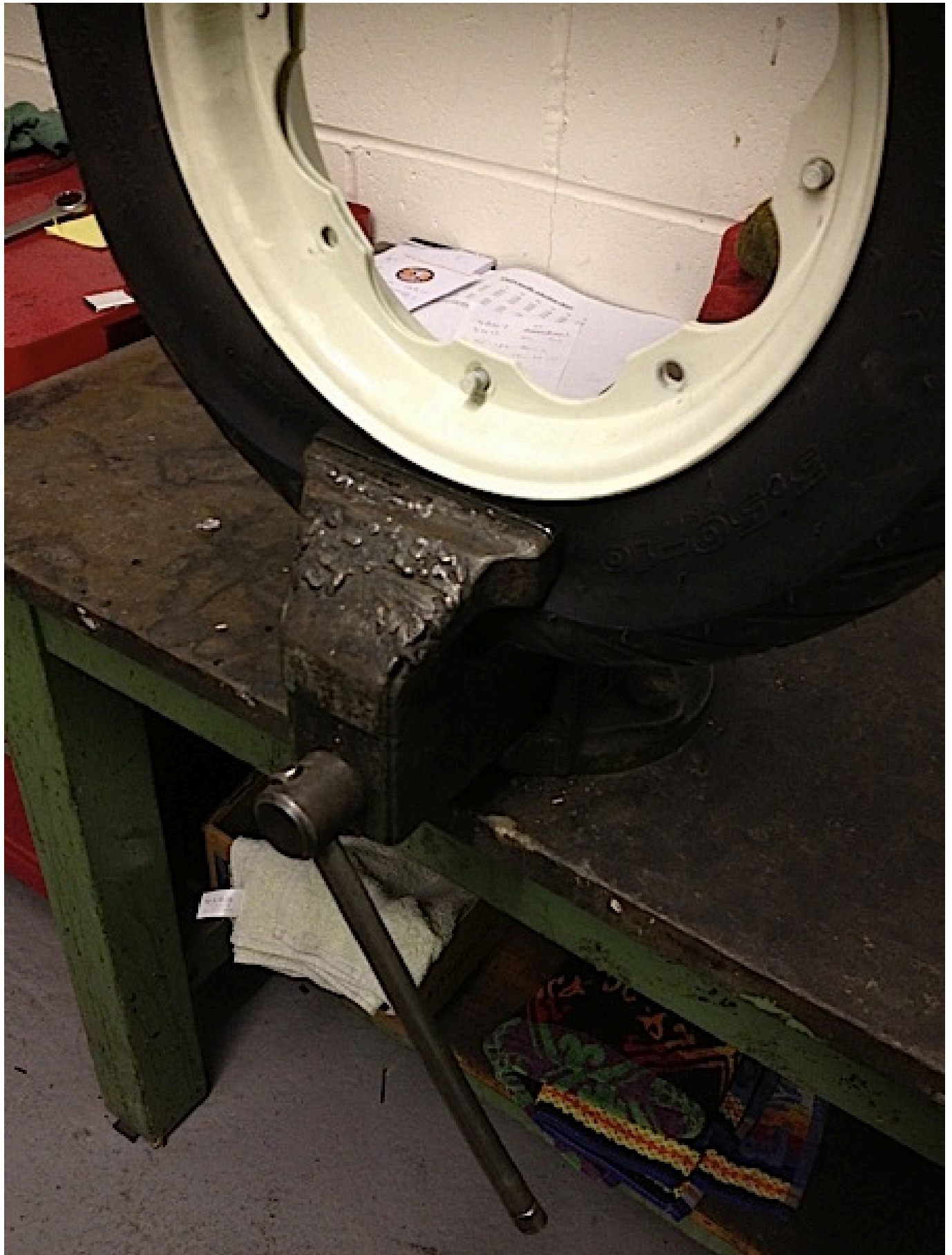
Really tight tyres can be gripped in a vice below the rim
