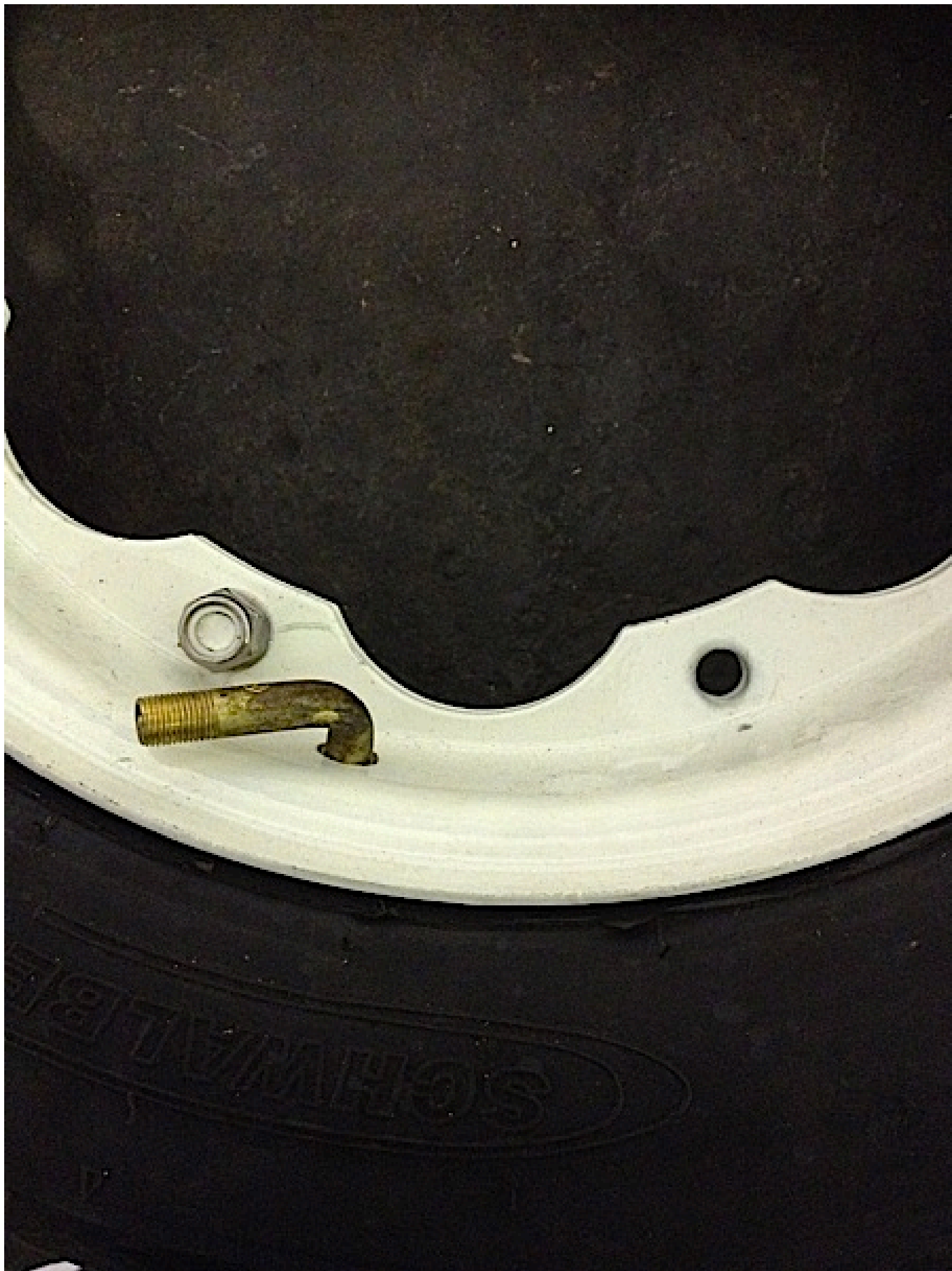
This rim has a valve hole offset to center of the studs which would clear the hub fin, but gets in the way of one stud
