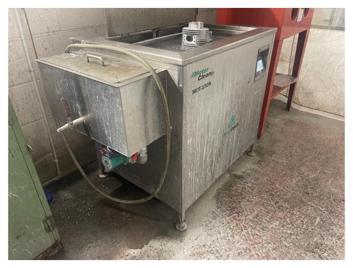
Our Ultra sonic cleaner is big, big enough for a full engine or the smallest part. The dirt on the outside is splashes off the floor when we wash off parts off. Its stainless steel throughout it just wipes off
