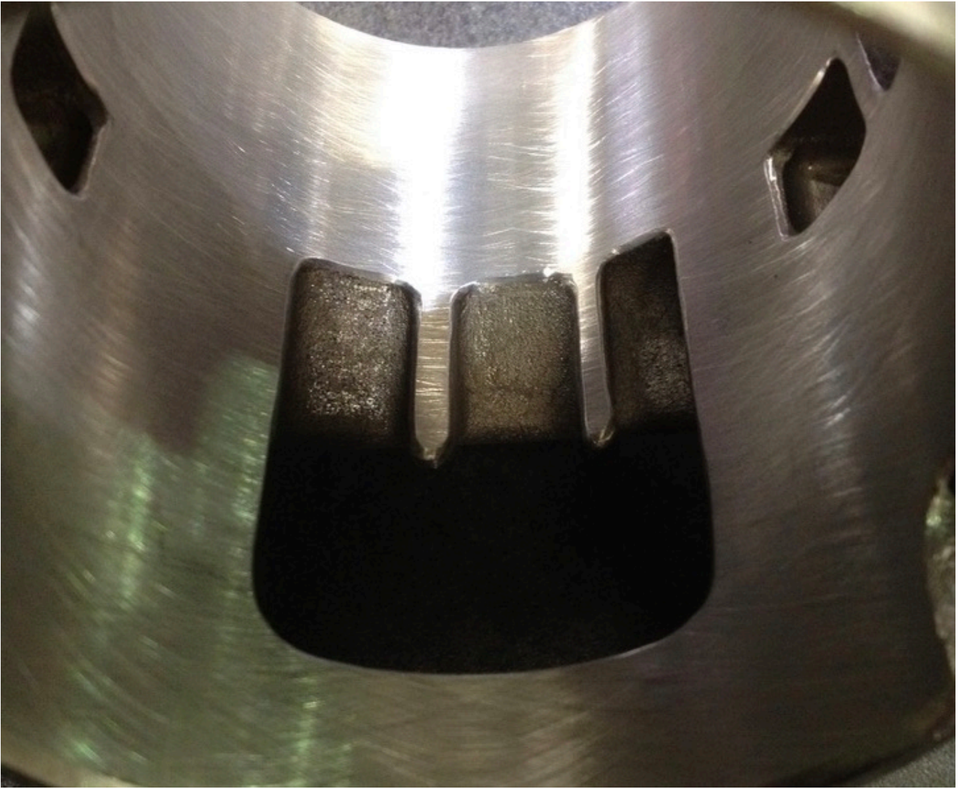
3 boost ports in the RB 250 cylinder
