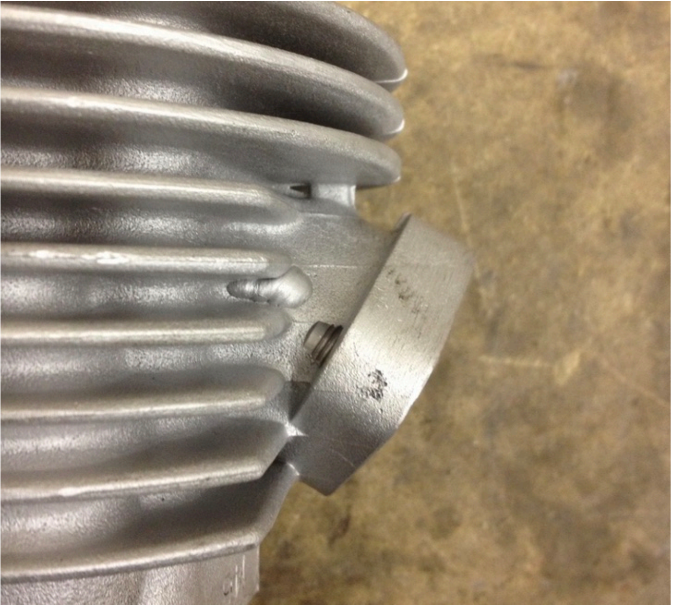
Same sloped exhaust port shape, needs a special exhaust
