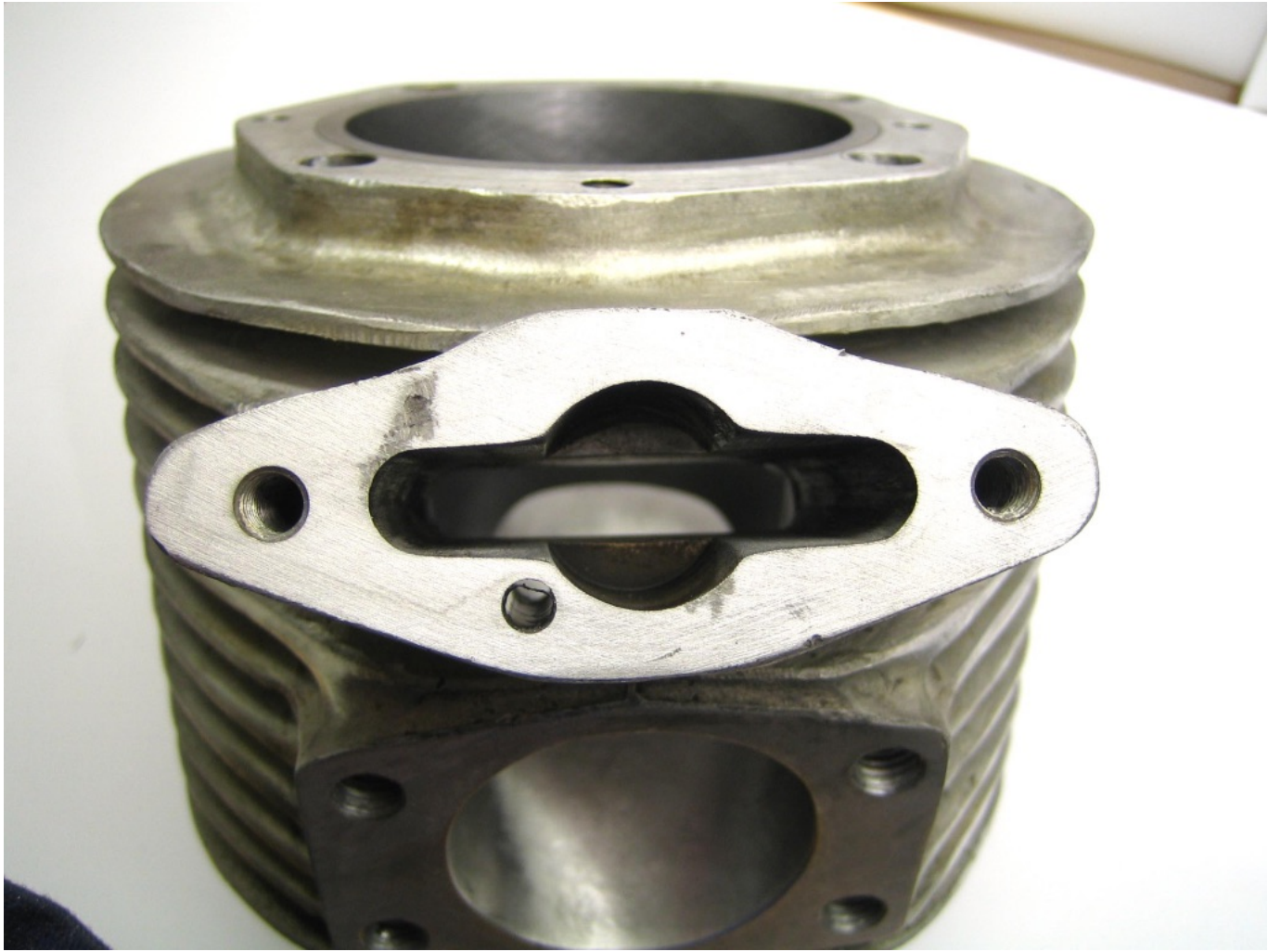
This shows the alloy casting removed from a Rotax cylinder and welded into position on a TS1 cylinder
