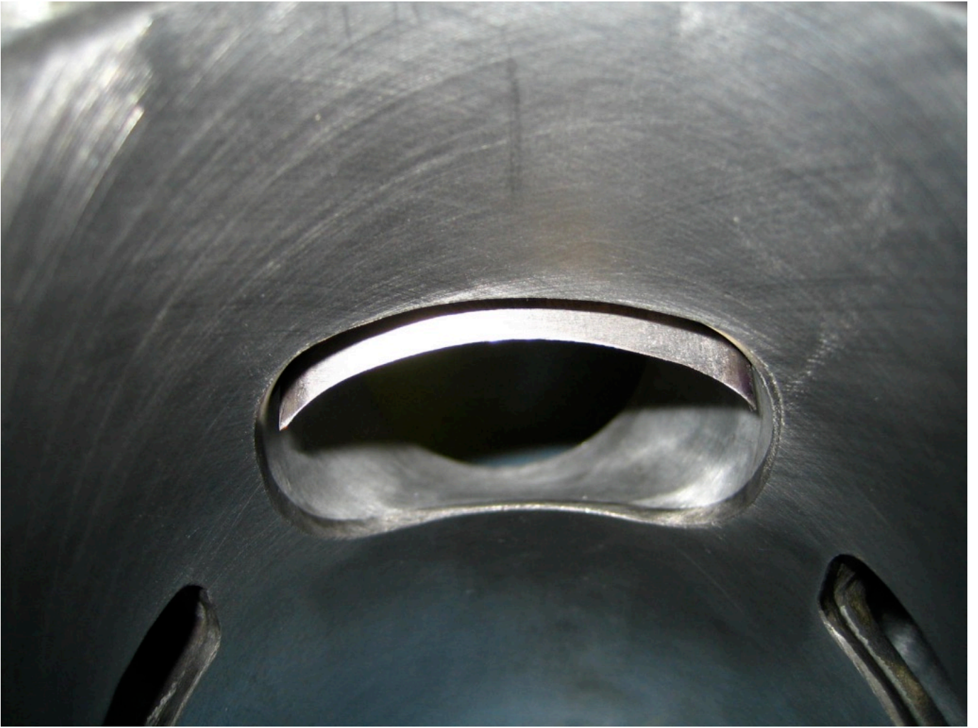
The Guillotine in the shut off position which the best pulling power
