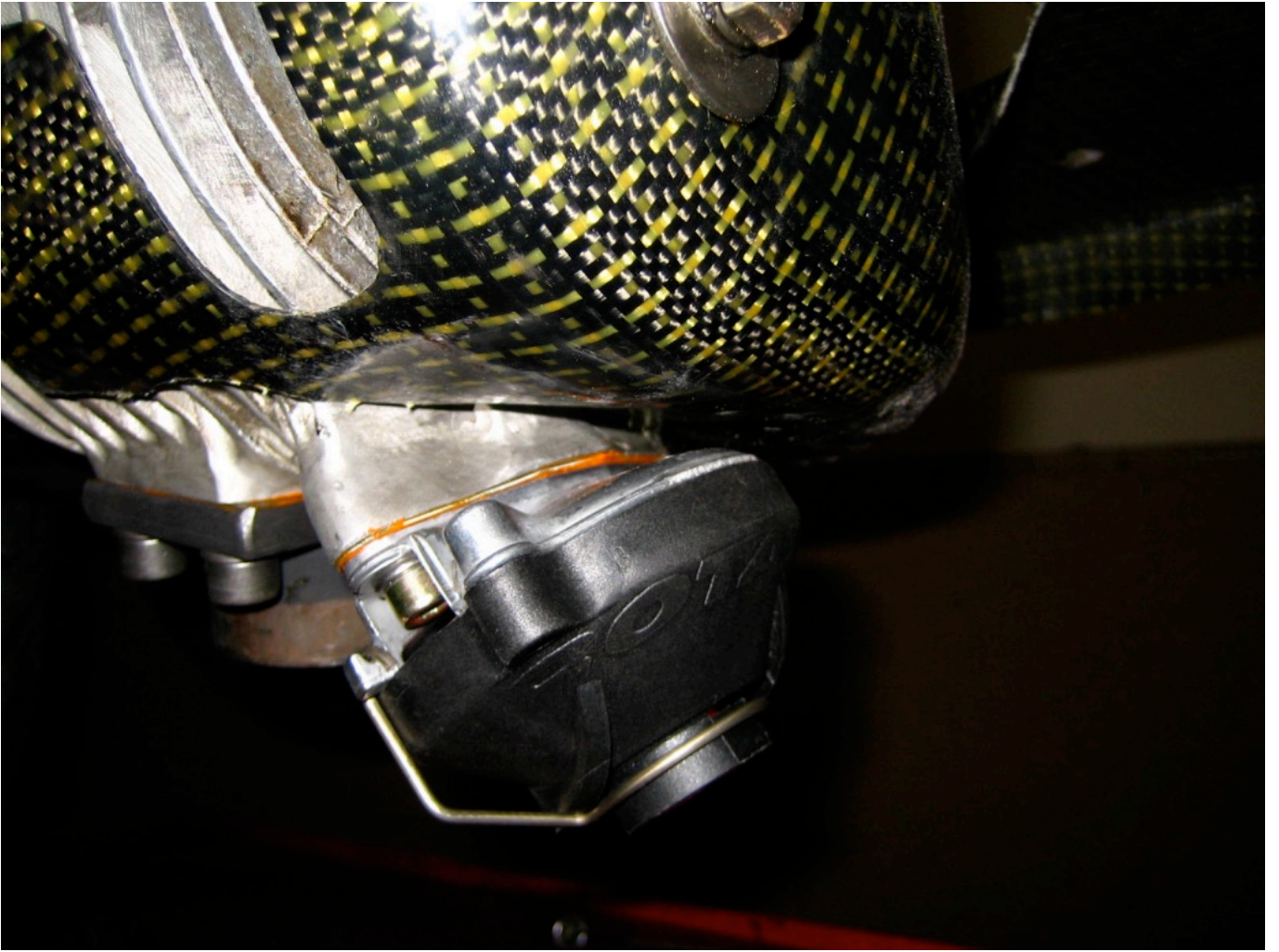
Power valve fitted above the exhaust port
