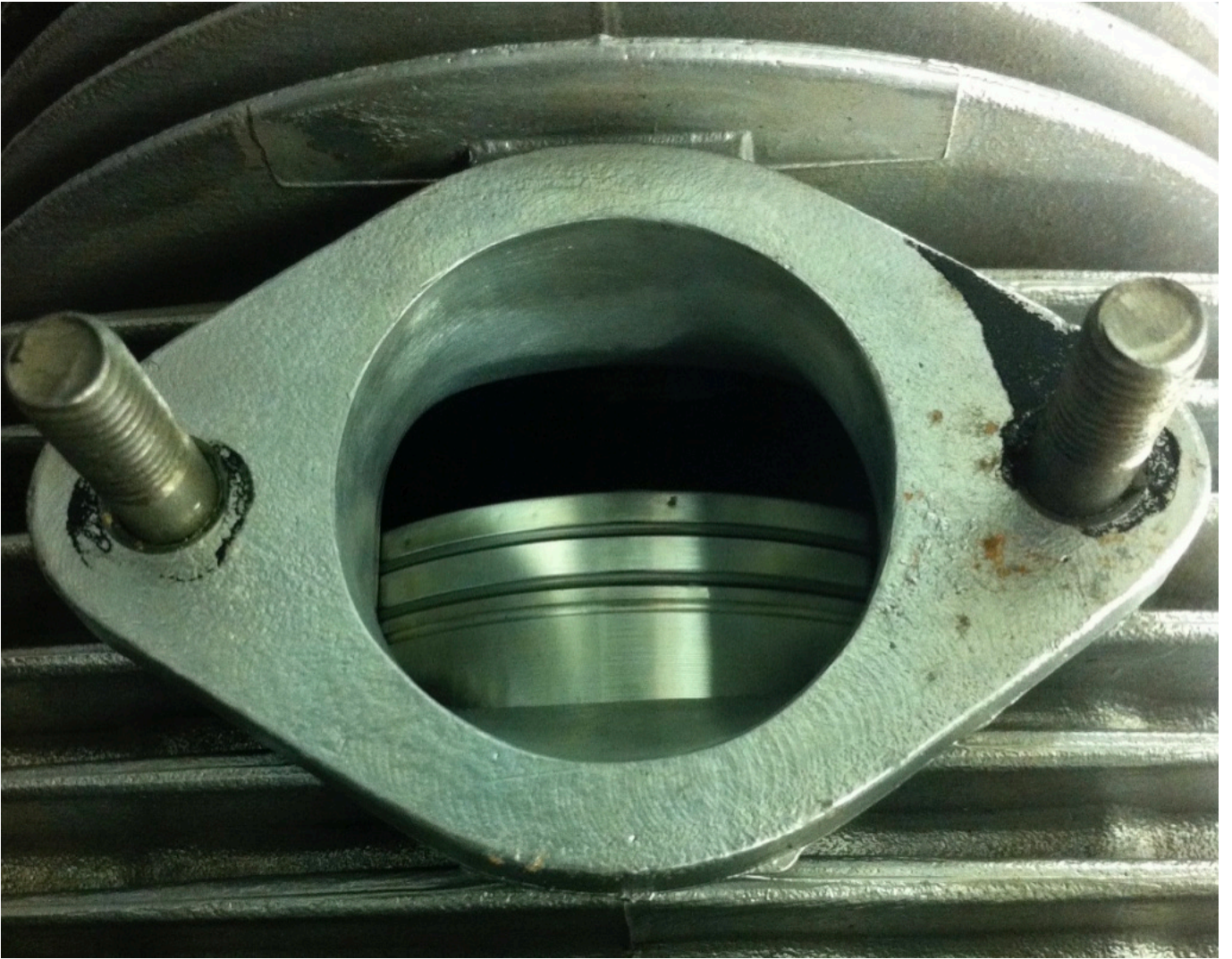
Road tuned exhaust port showing the MB forged piston
