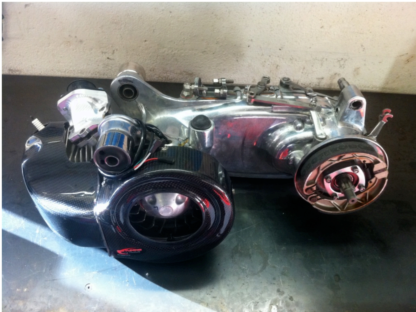
Completed MB5 TS1 rebuild
