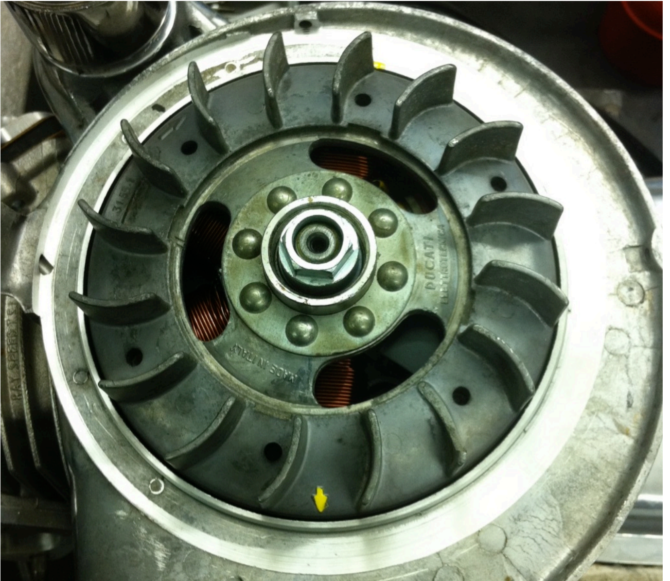
Old early AF Rayspeed flywheel, nice and light which gives power
