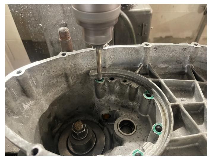
Once bolted in the jigs, centralise the drill and drill to the correct depth of the stud used
