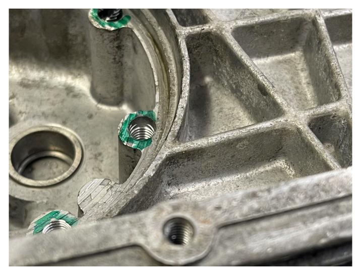
Even if the threads are not perfectly cut on the outer edge, our deeper studs lock onto new perfect metal lower down
