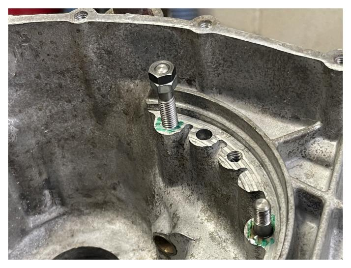
Double nut the stud, to screw in, check where it stops, tap a bit deeper until the larger thread is flush with the casing
