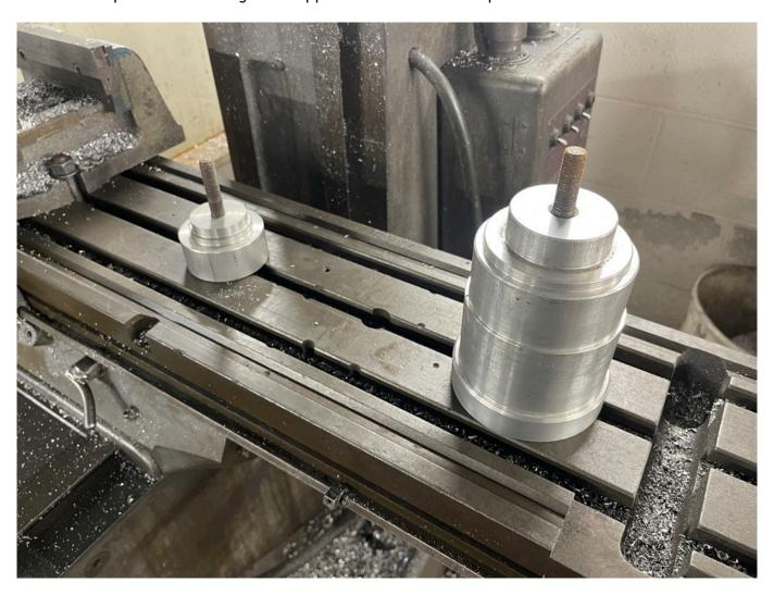
We mount engine casings on 2 special jigs mounting in the important bearing faces so the casings faces are true
