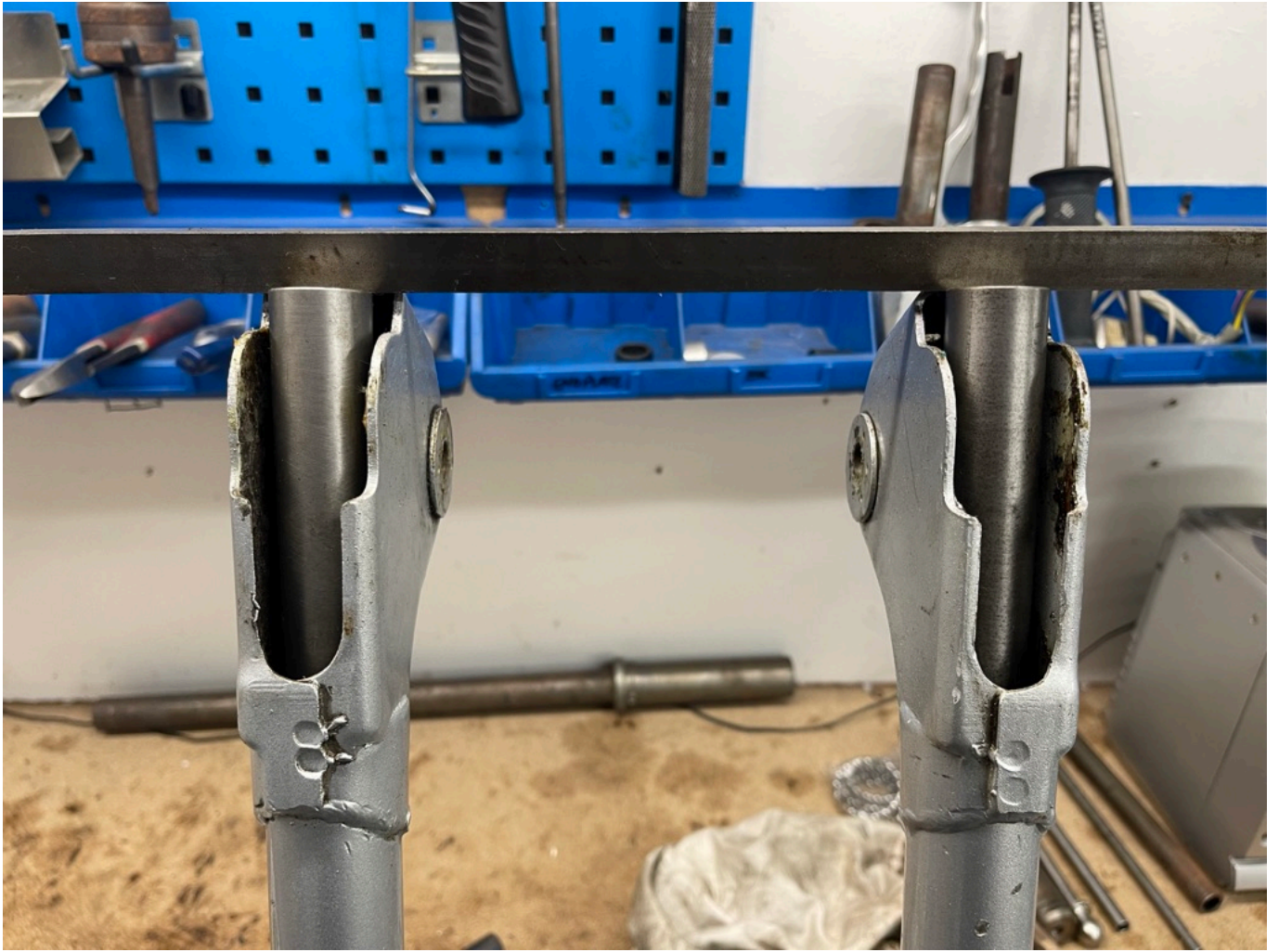
Laying the flat bar over the rods shows by eye how good the stops are
