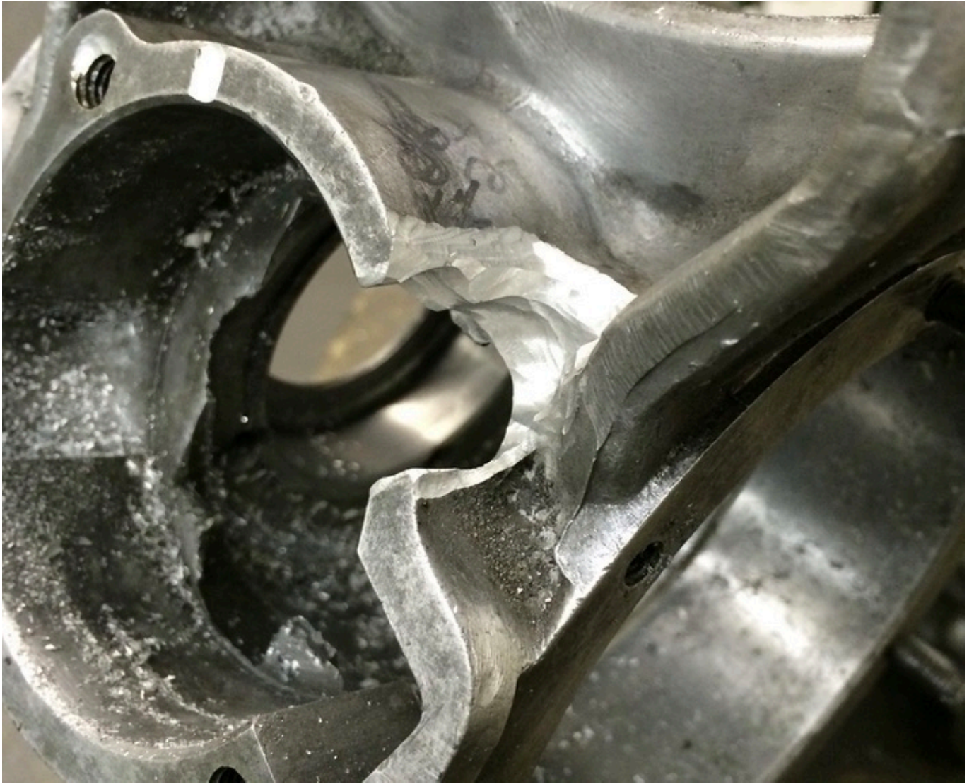
A regular job cylinder studs broken and cracked
