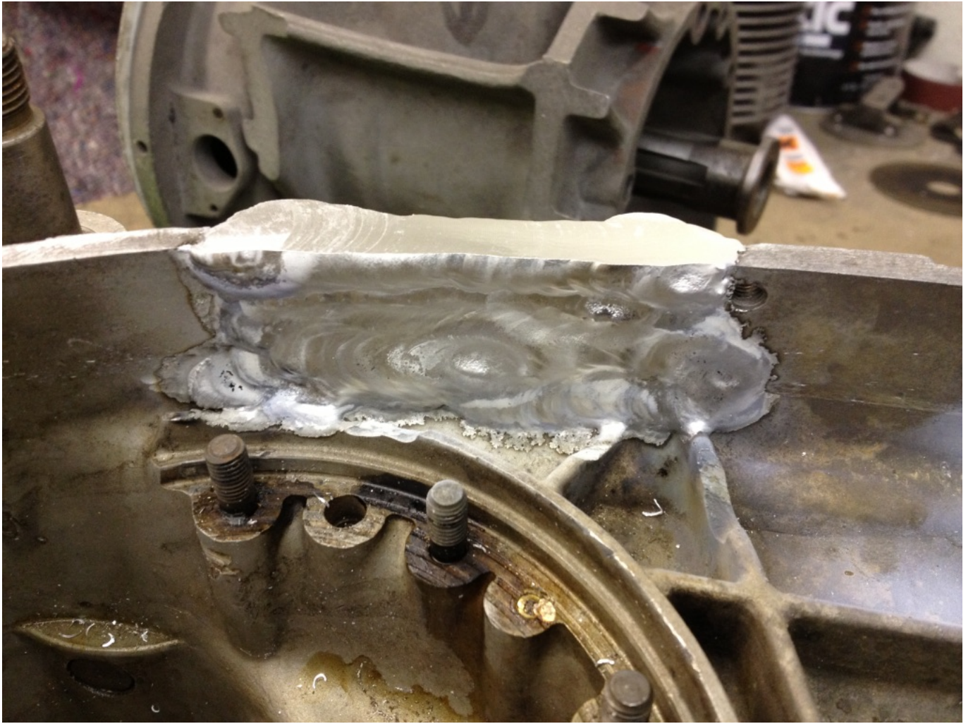
Welded and built up
