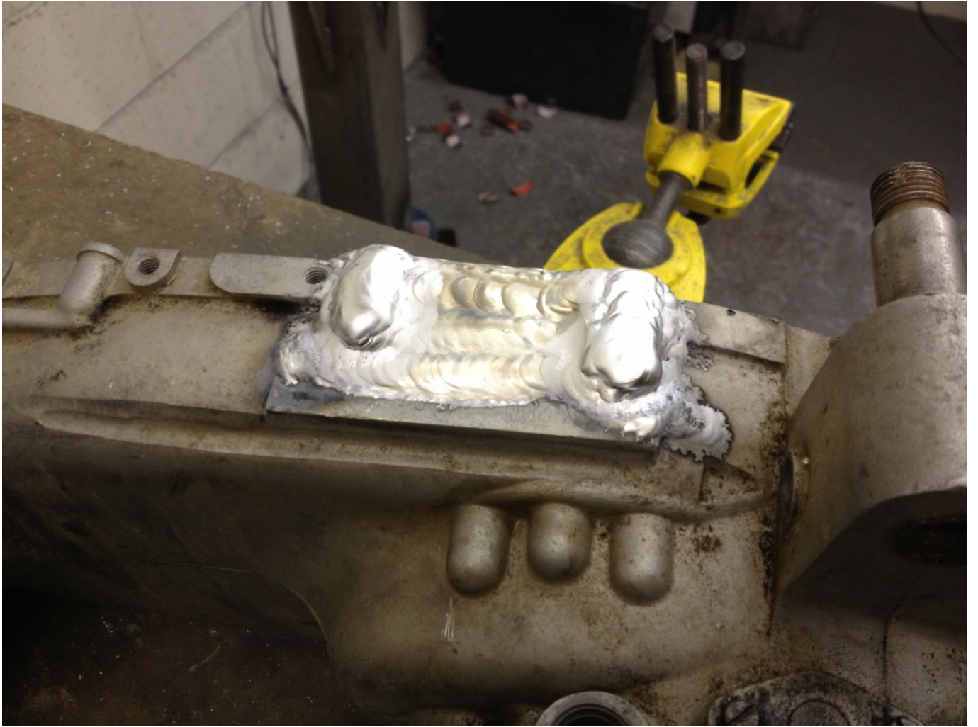
Built up and shaped to replace the stud holes
