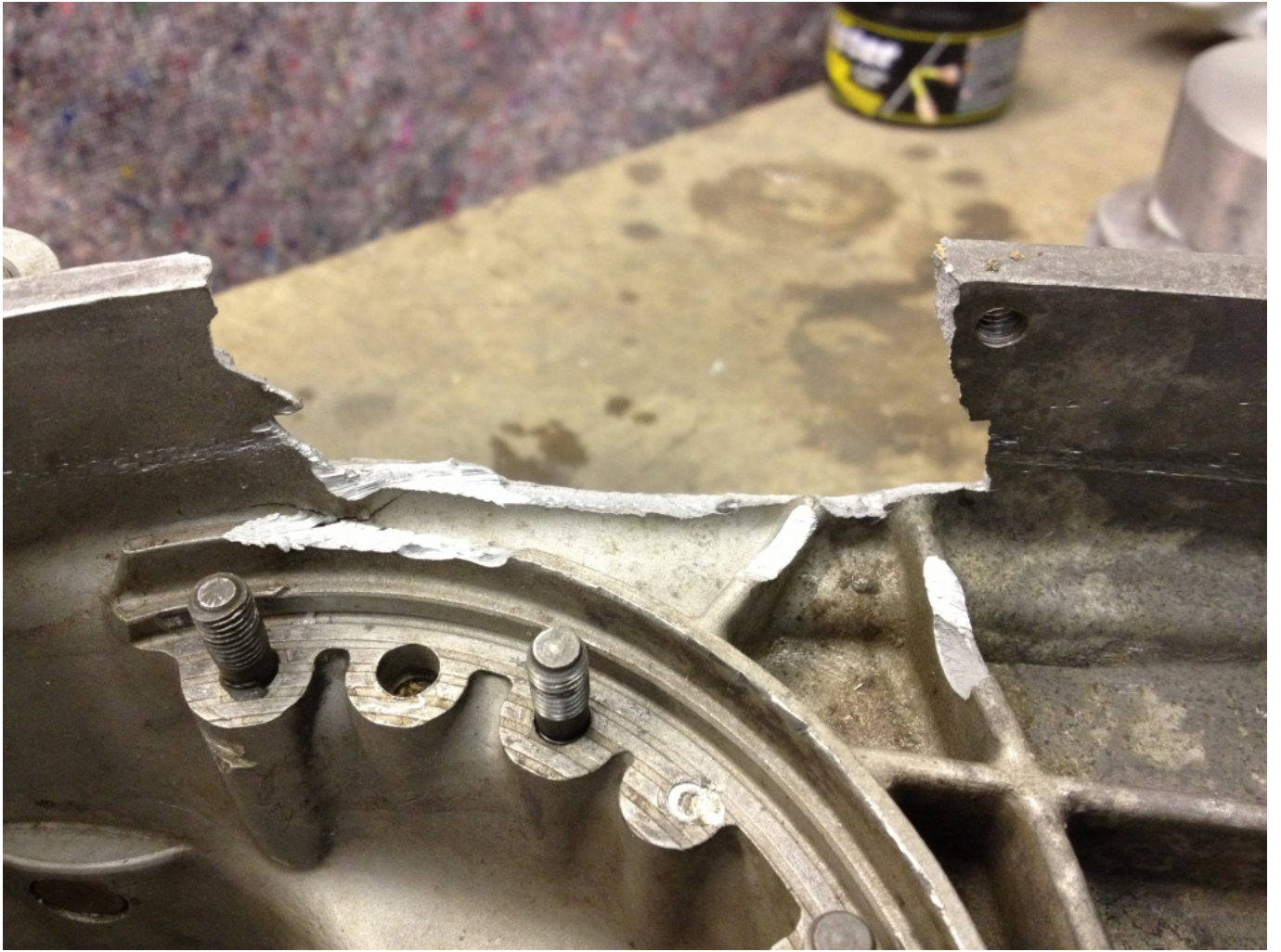
A bit of an explosion! Chain snapped!
