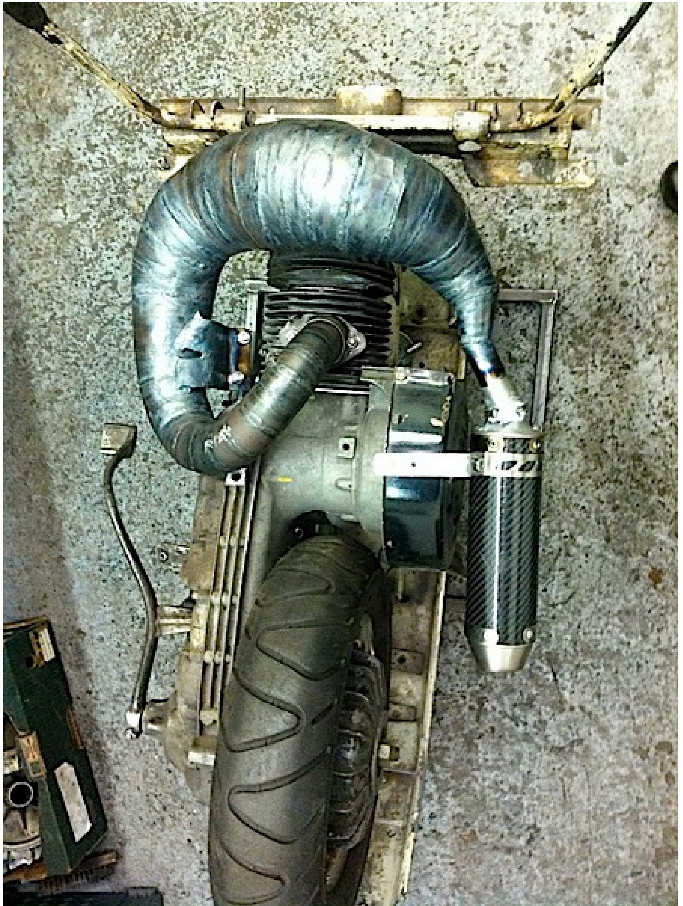
This was one of his race exhausts I had to modify to get better ground clearance
