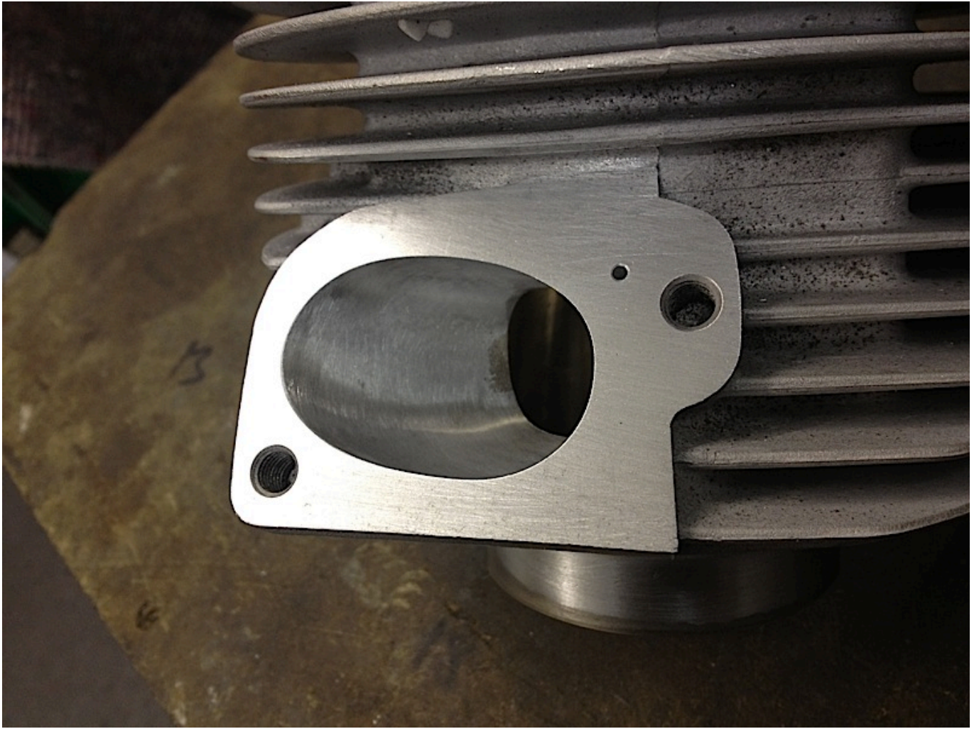
Note the little hole to pin the inlet manifold in perfect position
