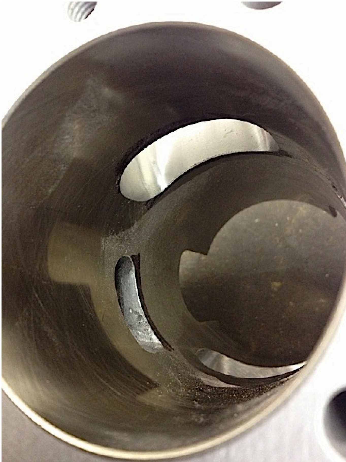
Transfers marked out and tuned to suit the 60mm crank
