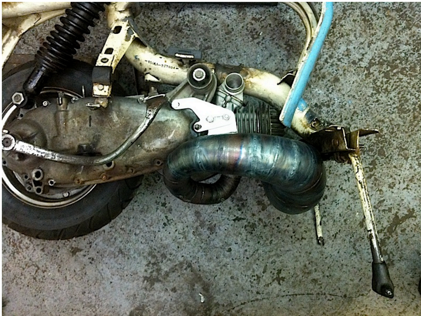
Set up on half a frame as a jig
