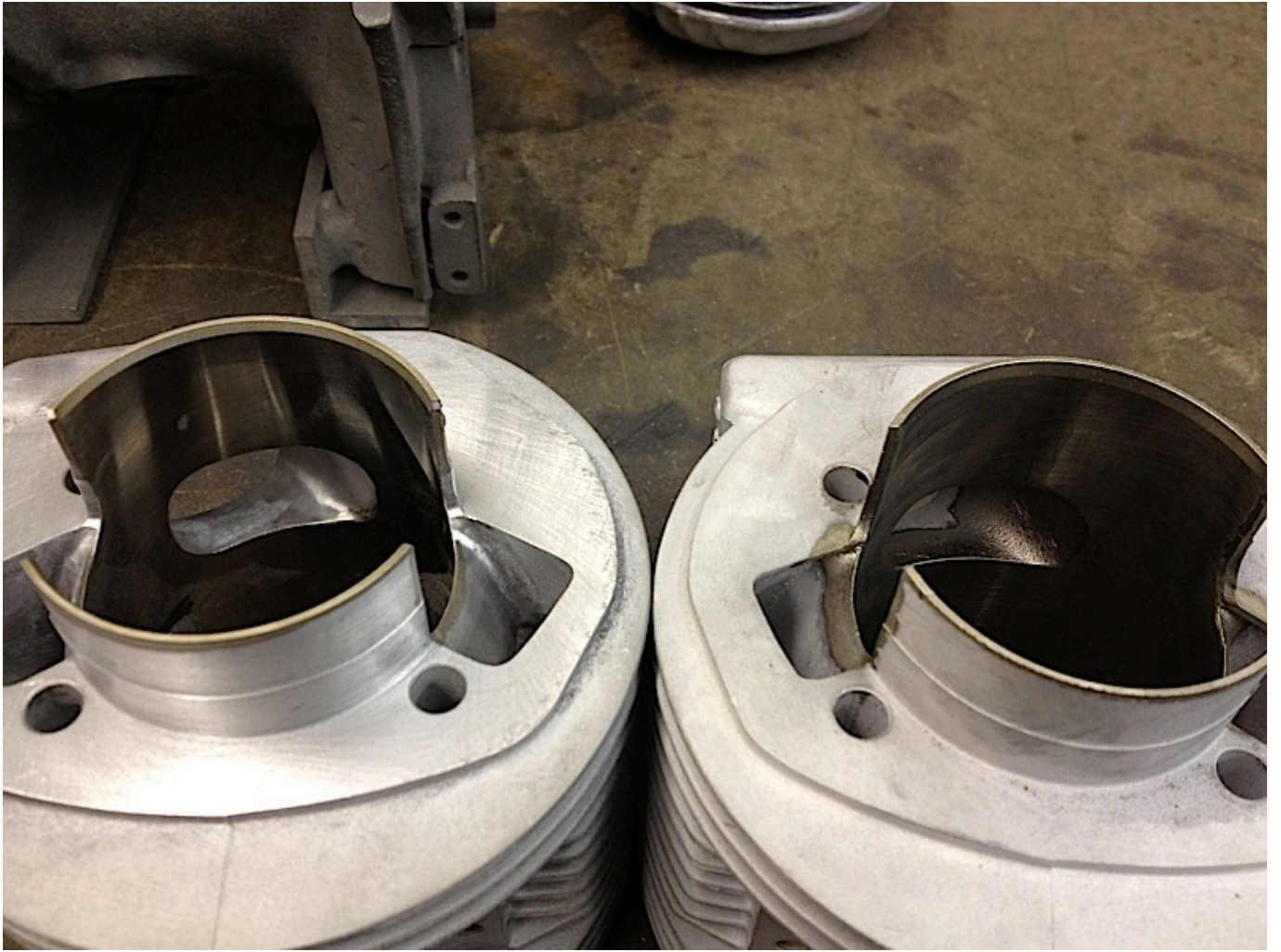
Flowed inlet port on the left and standard RT on the right
