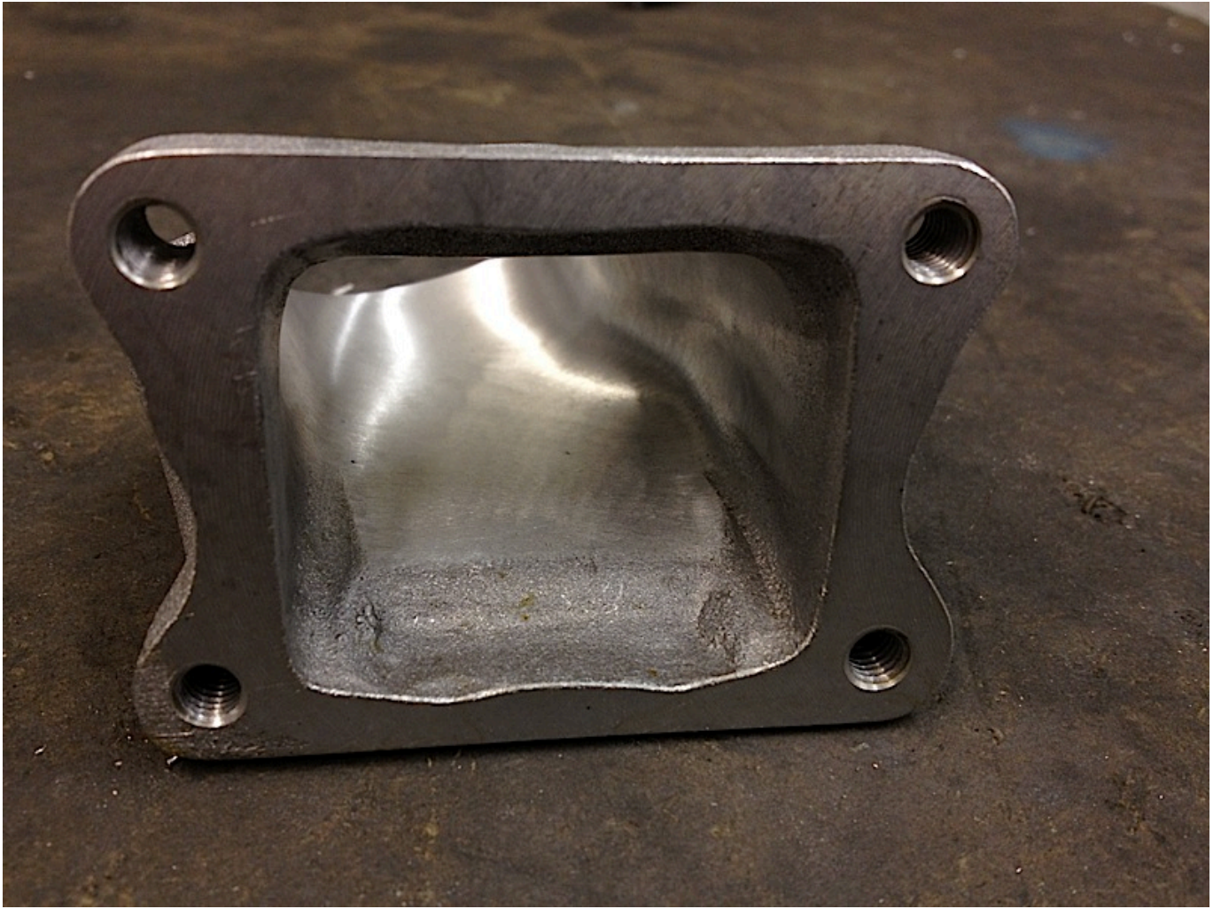
Sand casting surfaces cleaned and flowed where it's needed
