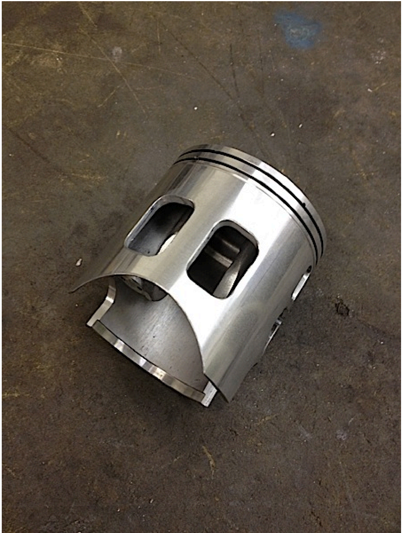
A MBgm full skirt piston modified for reed tuning
