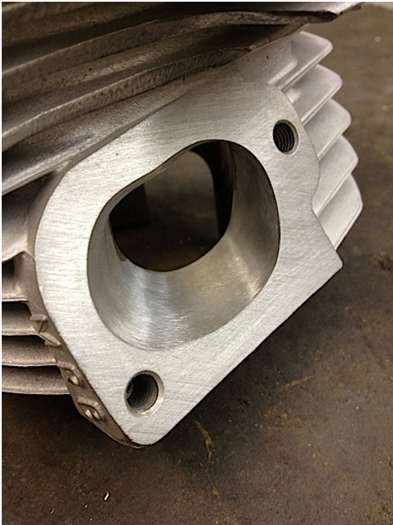
Inlet port lowered and shaped to the reed assembly
