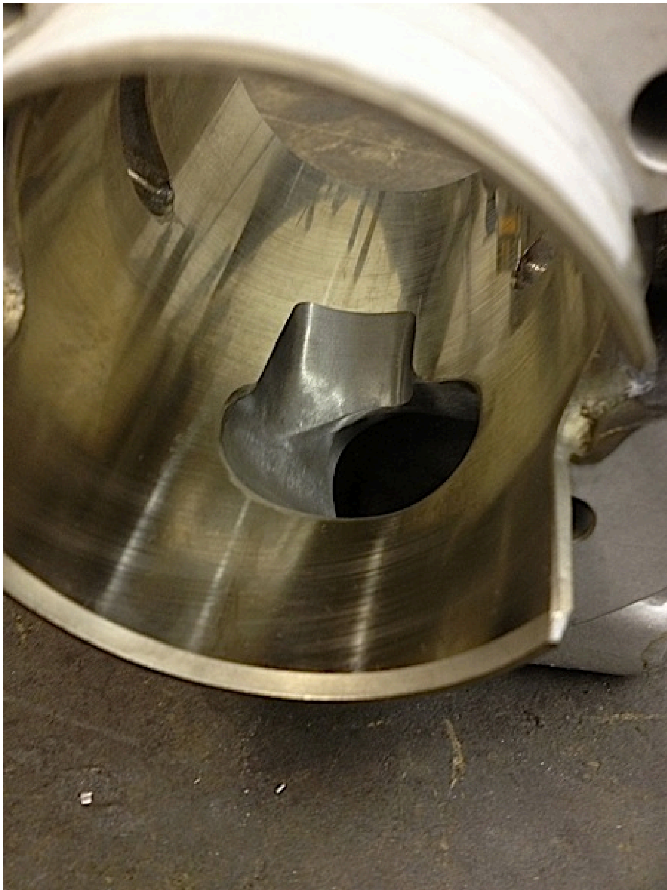
Rounded inlet shape for reliability
