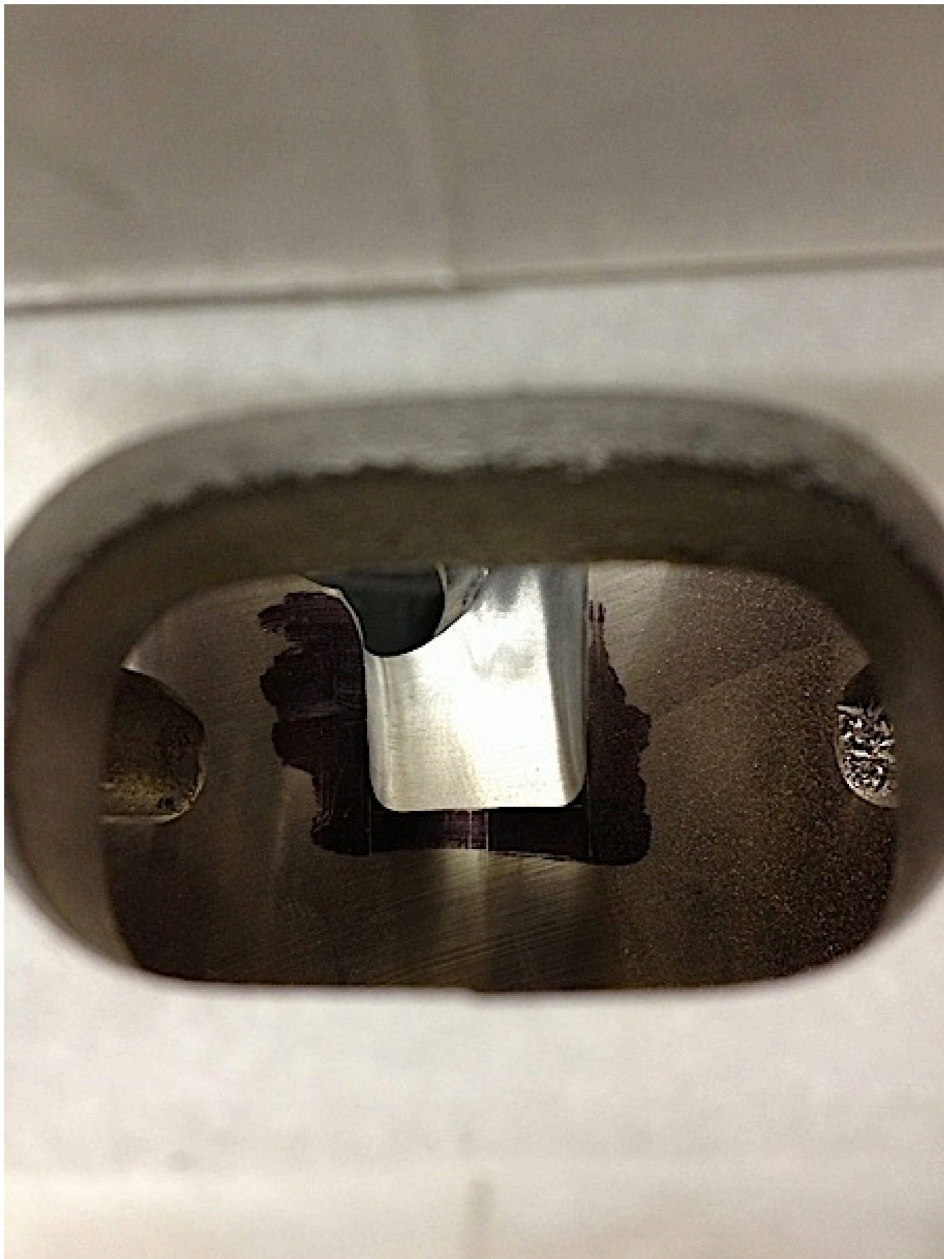
Finish tuned and flowed into the inlet port
