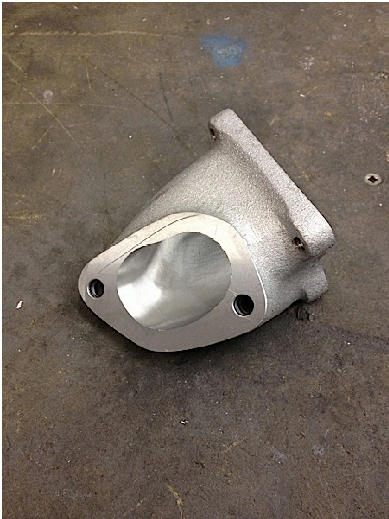
MB shorty Reed block, opened, matched and flowed to the inlet port
