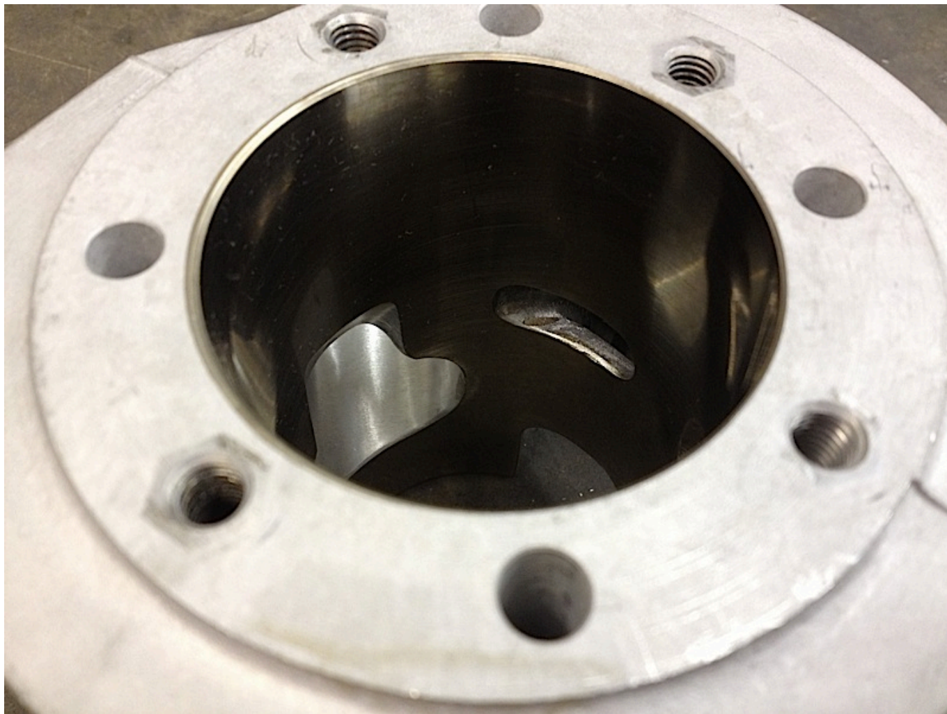
Reed boost port cut into the cylinder, which is very important, transfers cleaned up but not tuned
