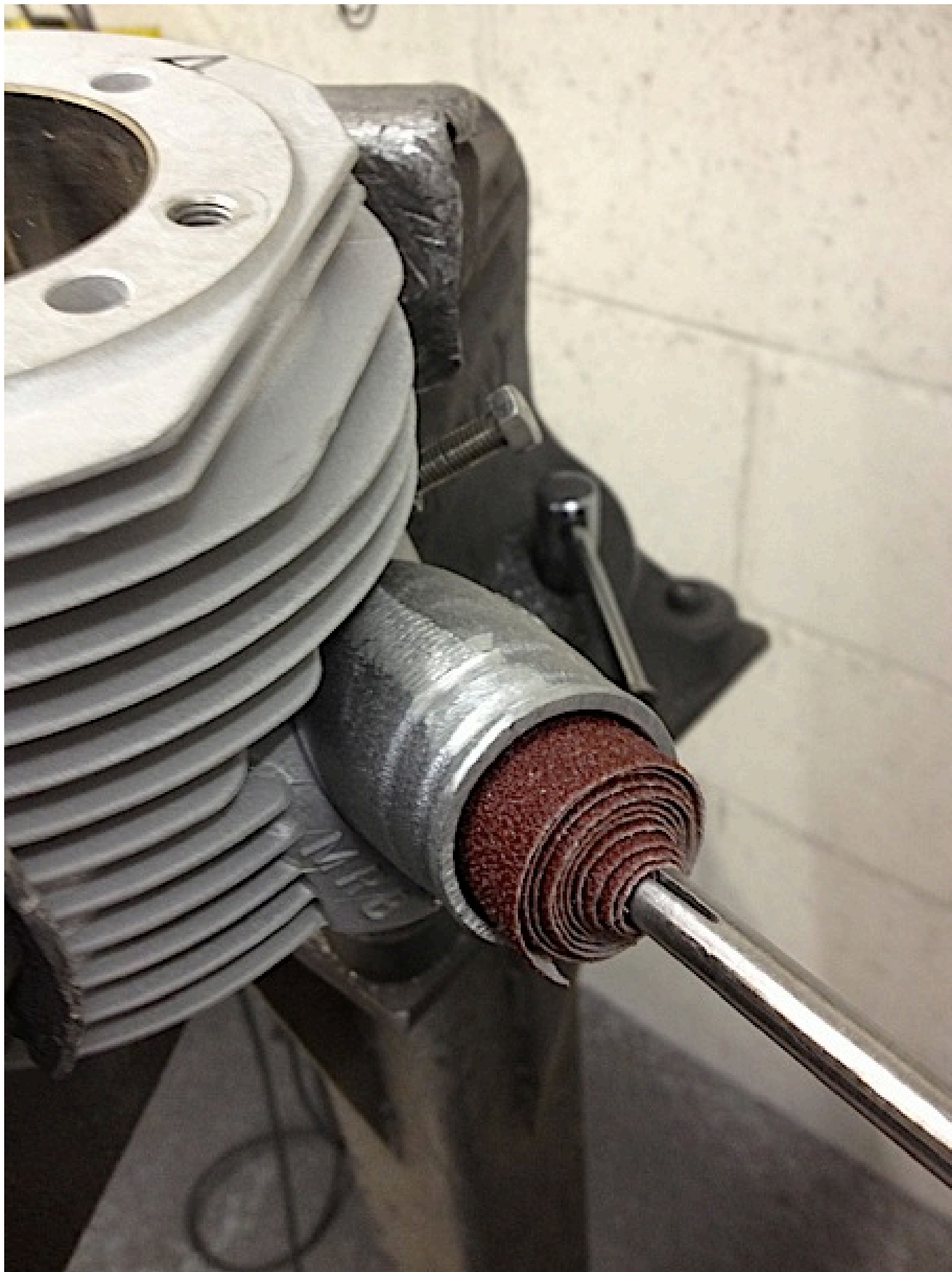
Flow the sand casting with rough 80 grit
