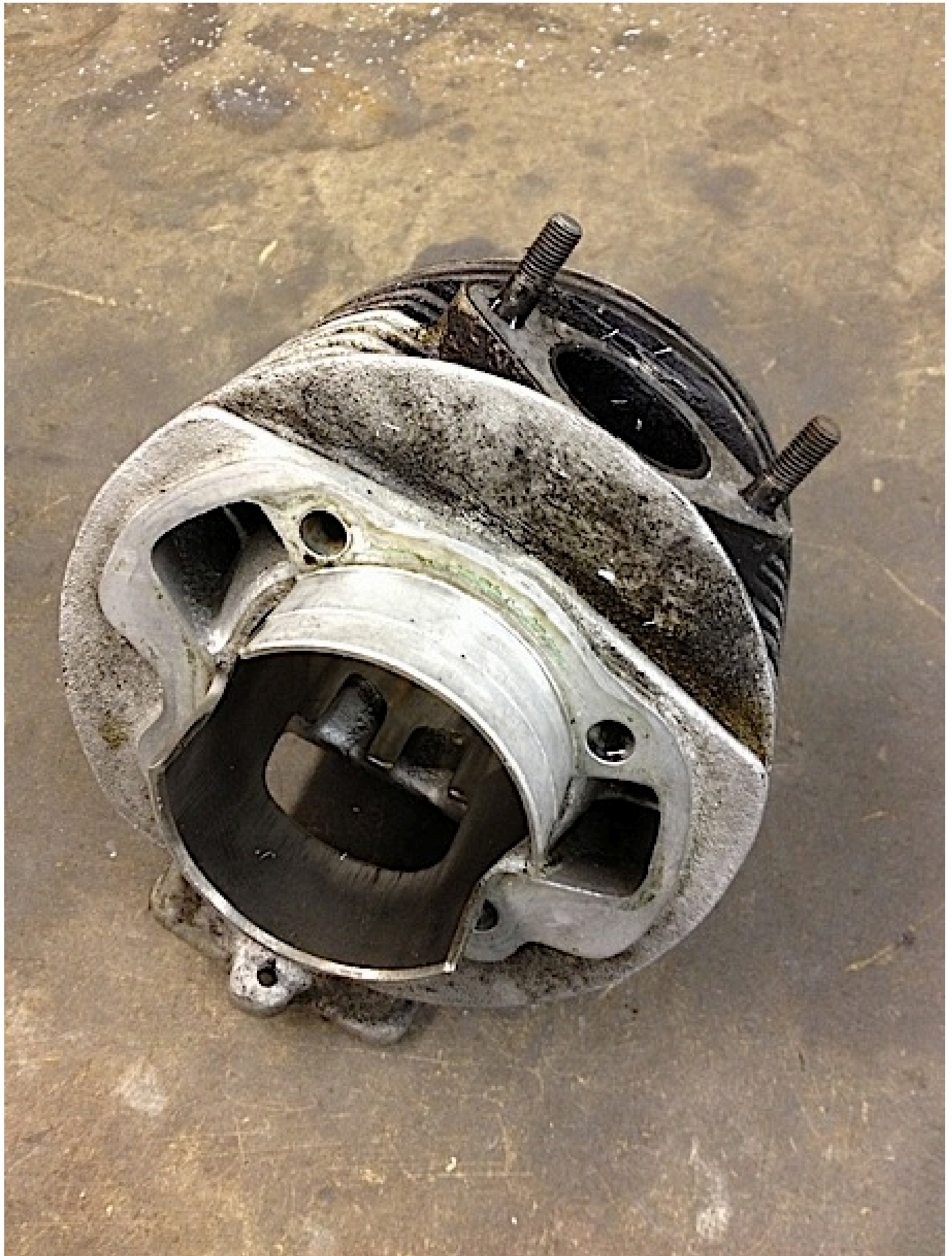
Standard Inlet port ports ready to modify
