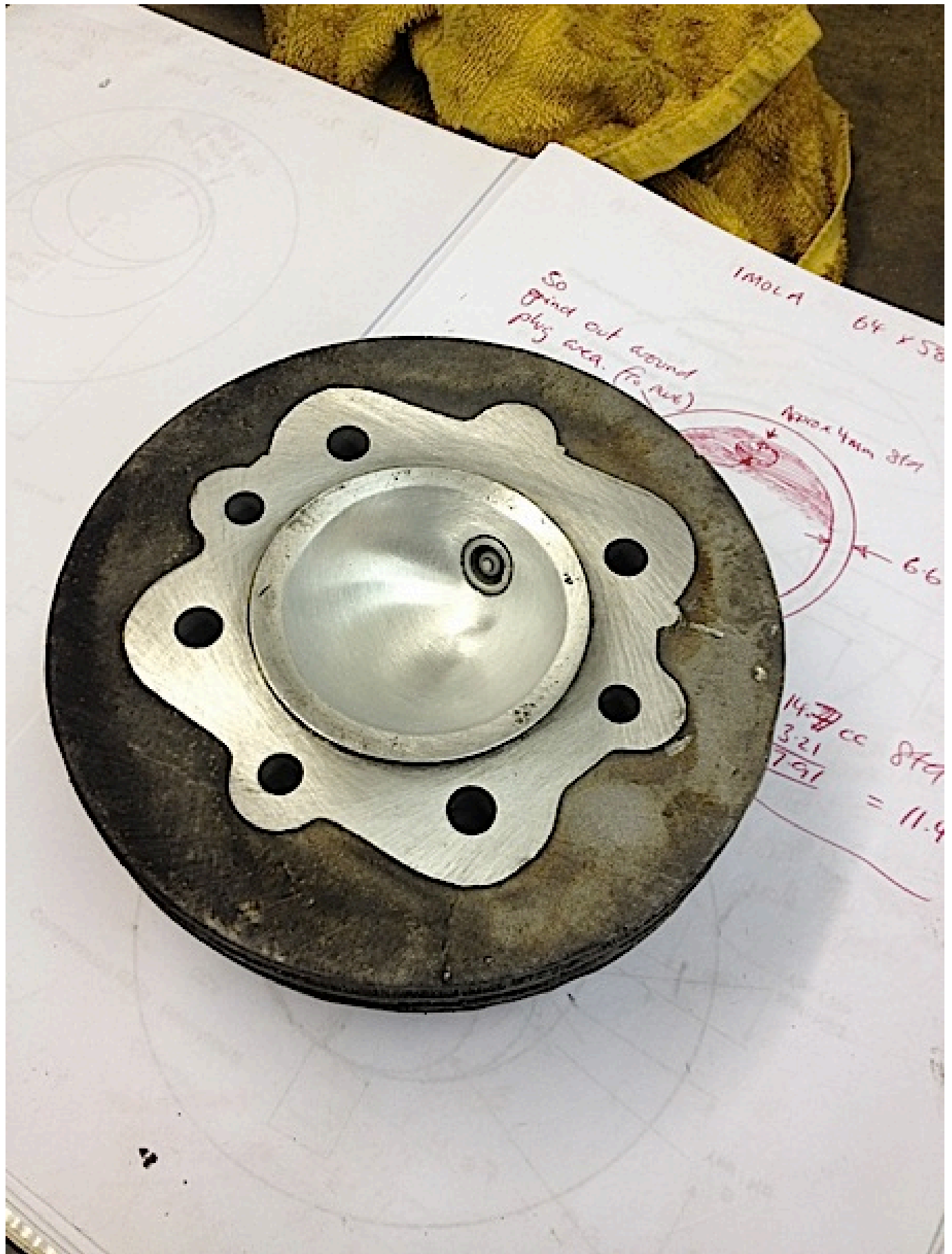
Modified lower compression head, the head standard is a little on the high side for todays fuel
