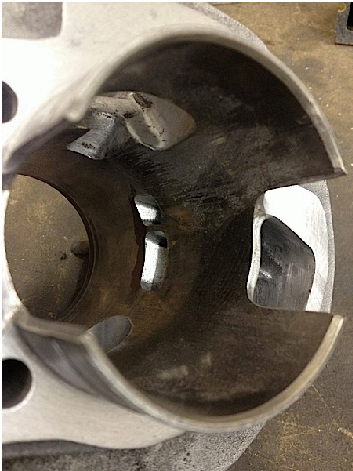
Transfers inside the cylinder are modified, leveled and widened
