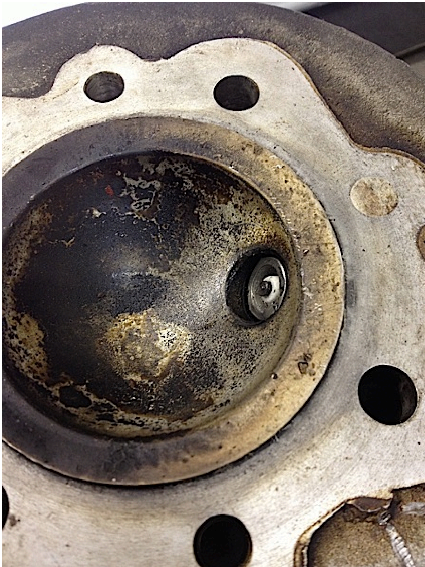
A standard center bowl head, check out how far away the plug is which needs altering
