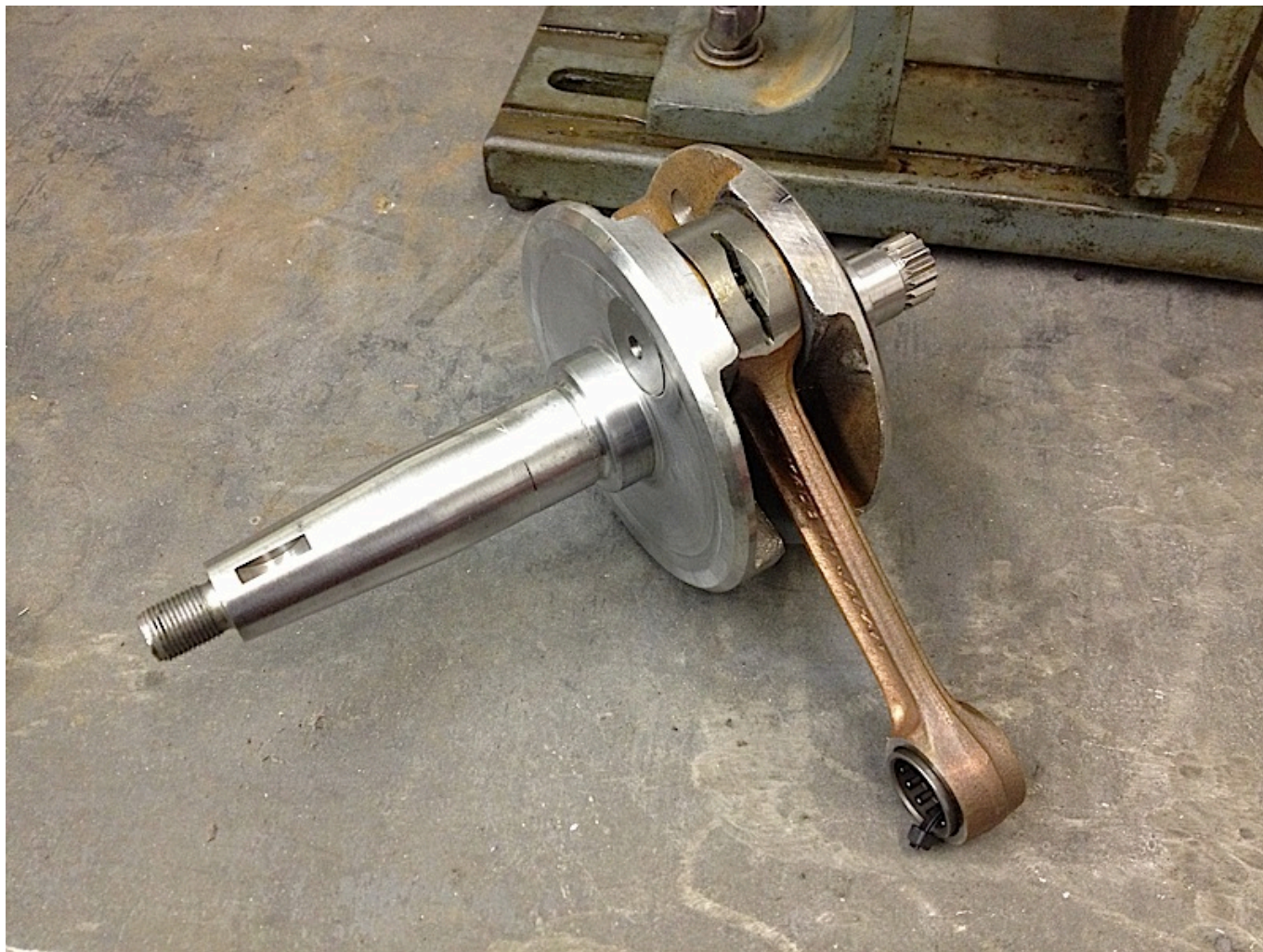
Crank webs machined, stronger rod and race bearings fitted
