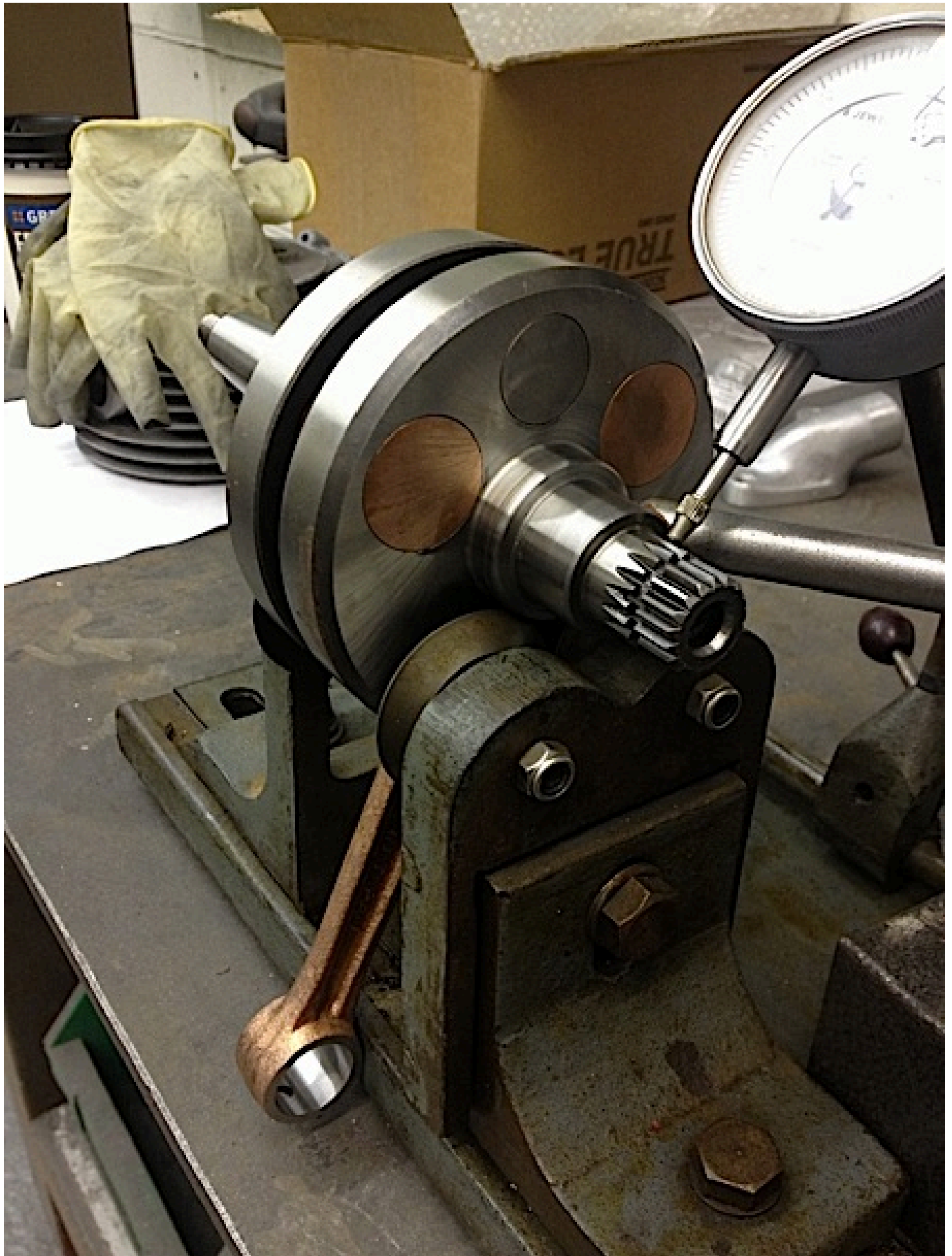
BGM crank on the jig after hand building one for a special engine
