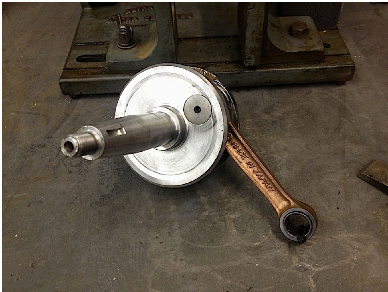
Indian crank modified with a Japanese Yamaha con rod conversion
