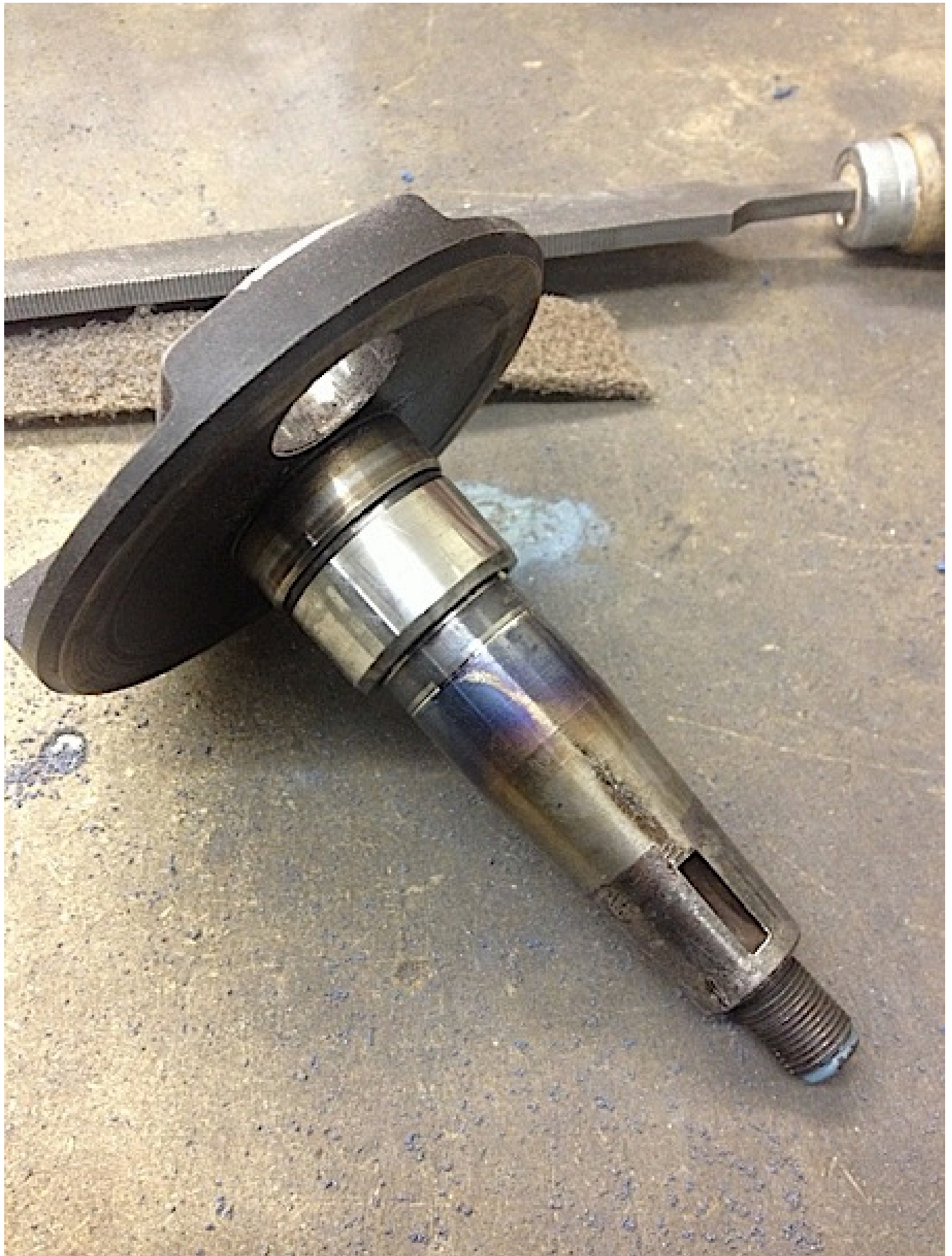
A rough old MEC Black crank, reworked to clean up the damage
