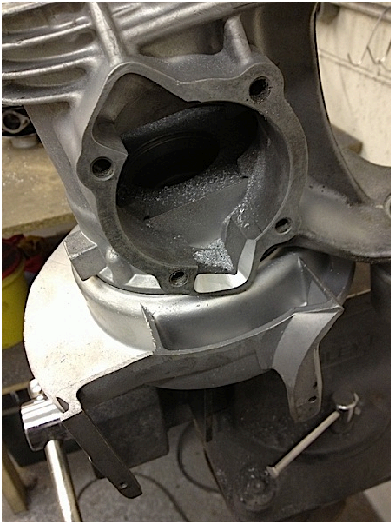
Casing get thin on most types of Imola without welding, if your lucky
