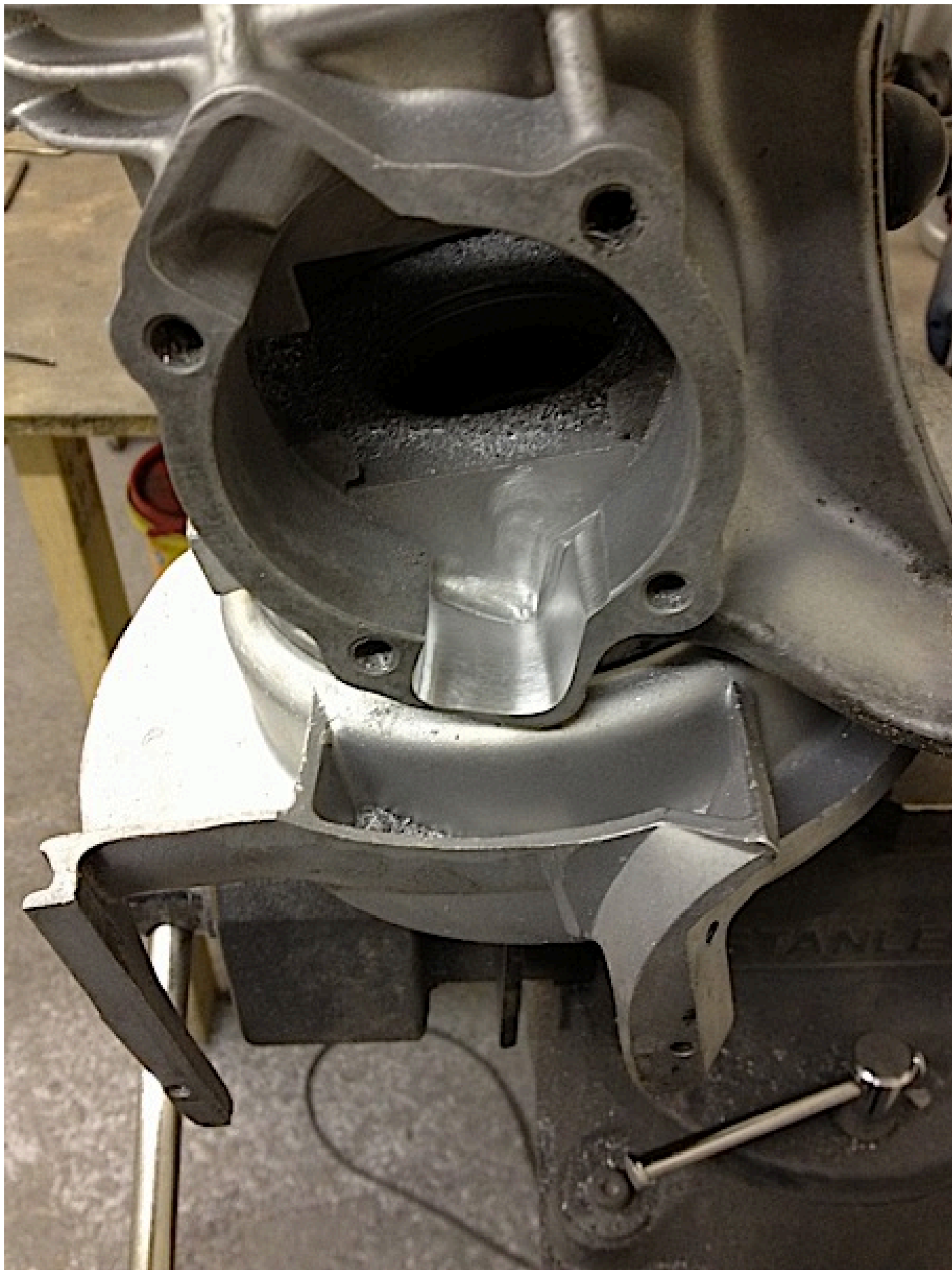
Mag housing matched and flowed with the transfer feed
