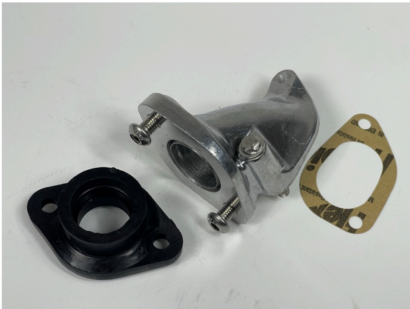
MB Flange inlet manifold showing the extra sealing ring cast into the manifold
