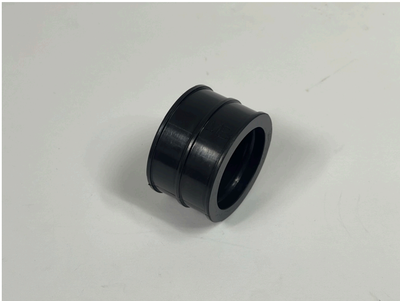
Tube type carb mounting rubber, same size both sides
