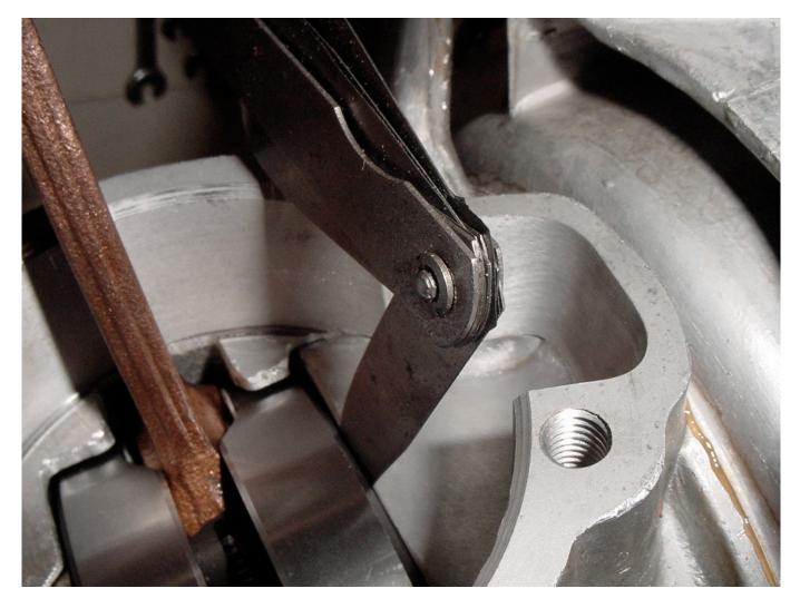
Use feeler gauges to check gaps between crank webs, drive plate and mag housing
