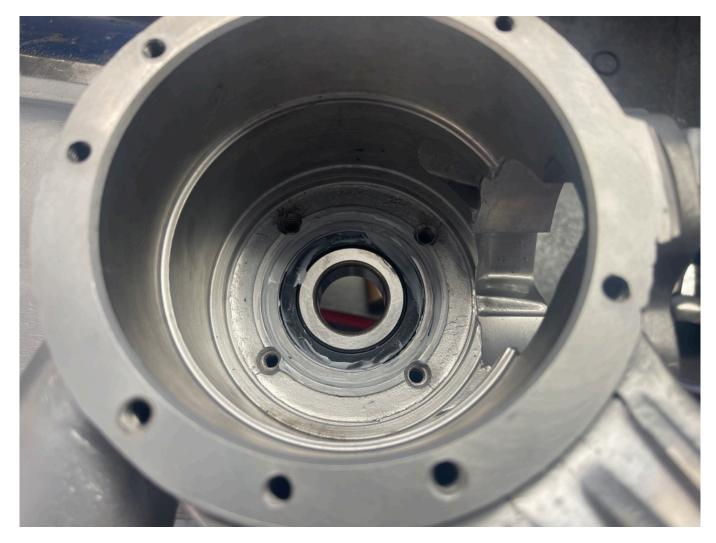
Once the bearing is fitted, wipe the sealer around the outside of the bearing, but keep it away from the inside of the bearing
