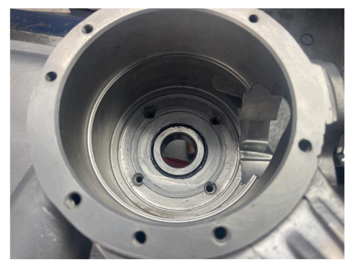
Smear the gasket on both sides and fit, wipe sealer into the outside of the gasket to help seal the outside of the bearing
