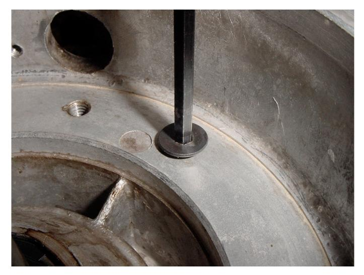
Use a counter sunk screw to centralise and locate the mag housing in the same place, do this every time and timing marks will always be the same on strip downs
