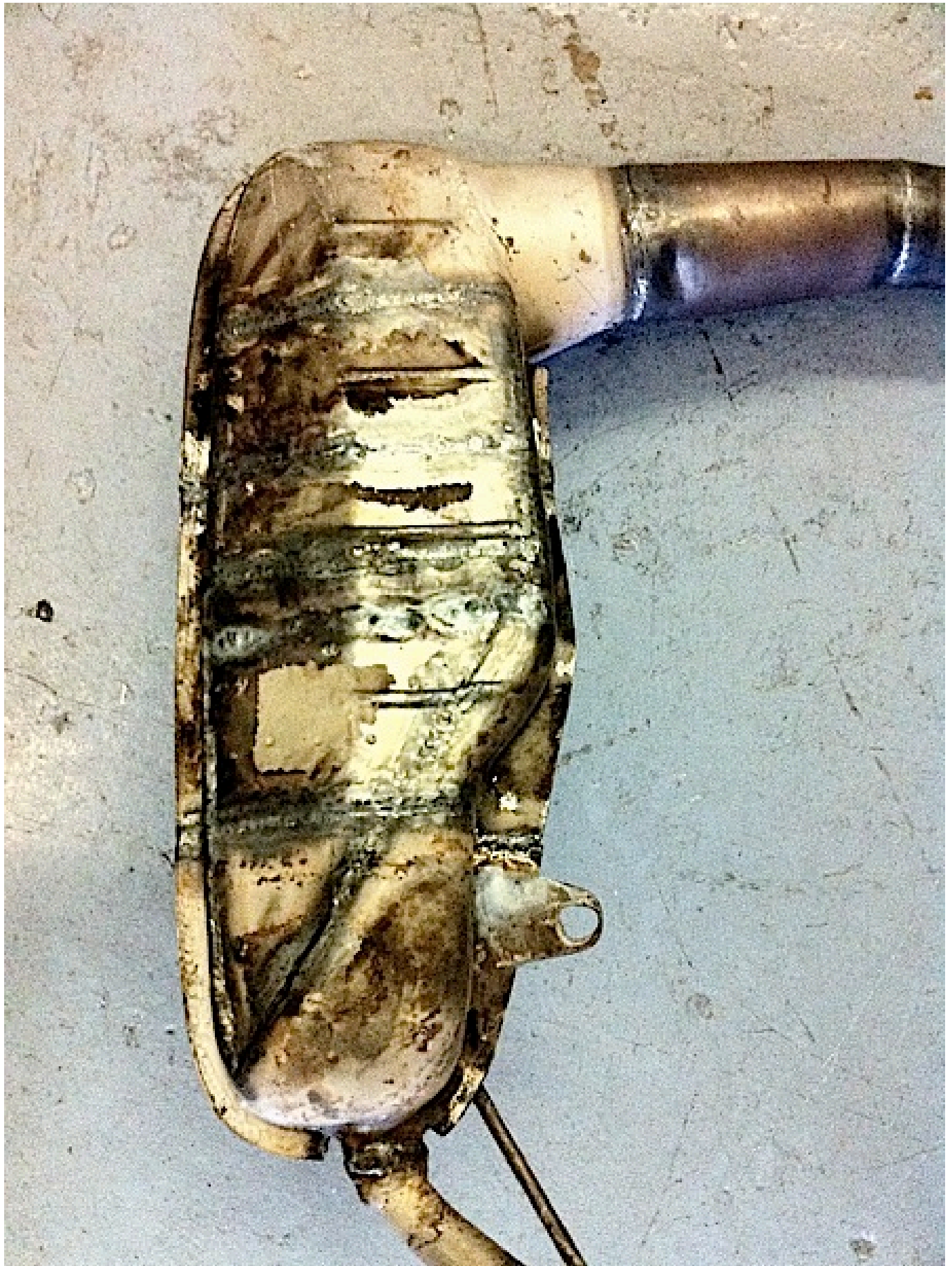
This shows the amount of times we have cut and modified the internals just on this one pipe
