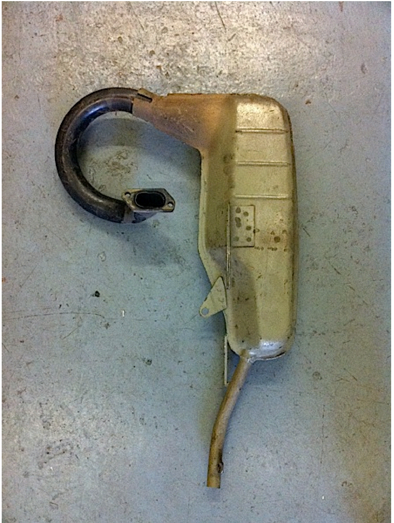
SIL Indian big bore exhaust, showing a small cone leading into the main exhaust box and a strange angled U bend which makes fitting the main exhaust difficult. These really worked nice on a mild tune.
