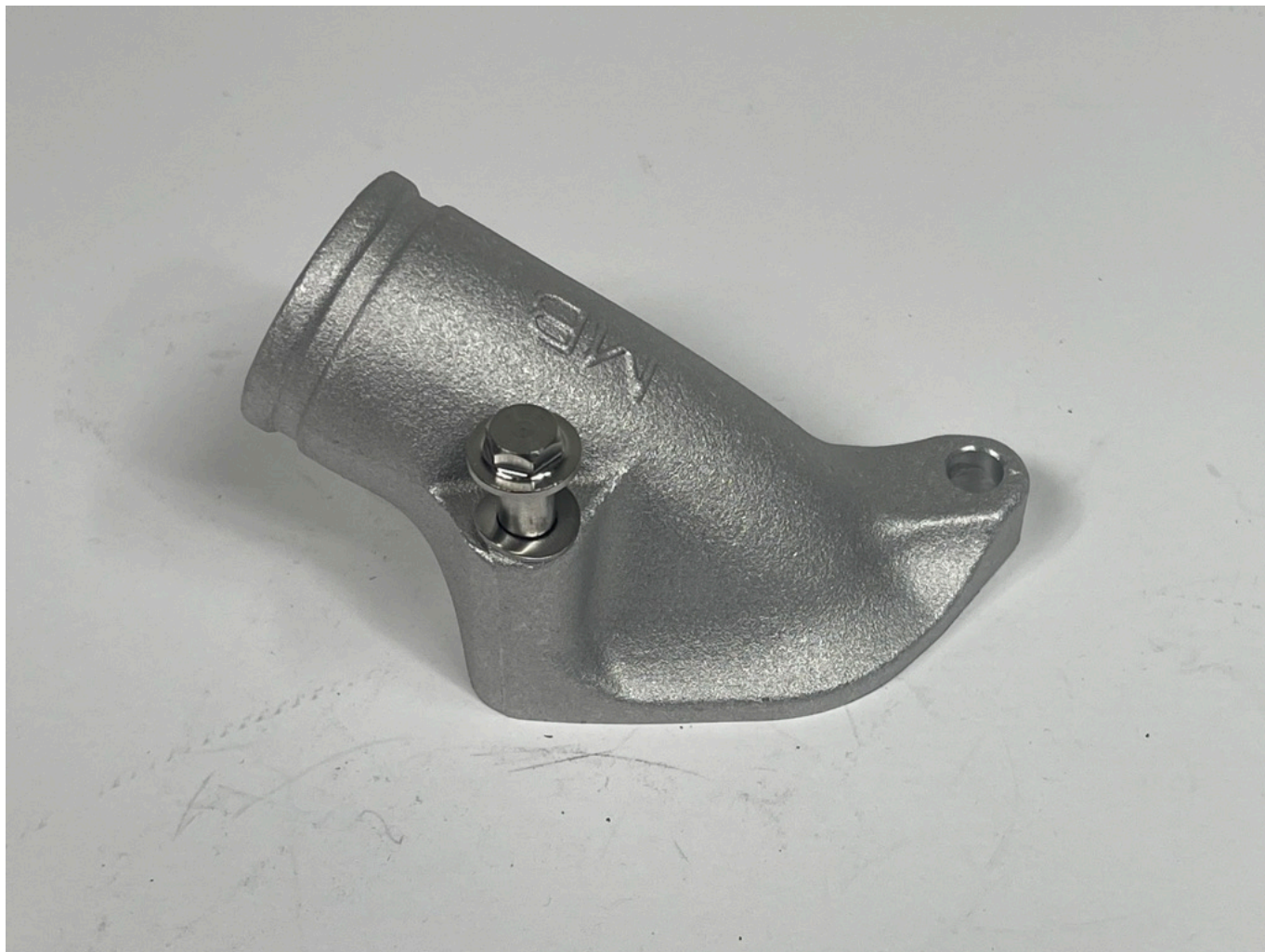
Die cast MB large block 30mm inlet, ideal for cutdowns, choppers and bikes with no side panels, better down draft flow
