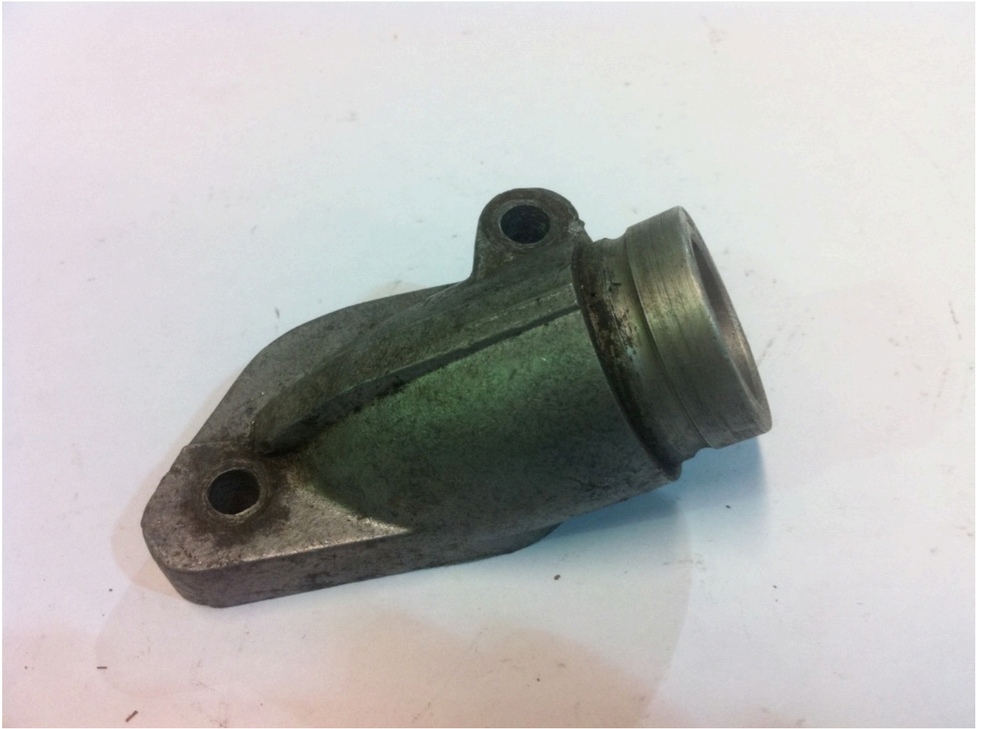
A modified CDC small block inlet machined to suit a rubber mounted carb
