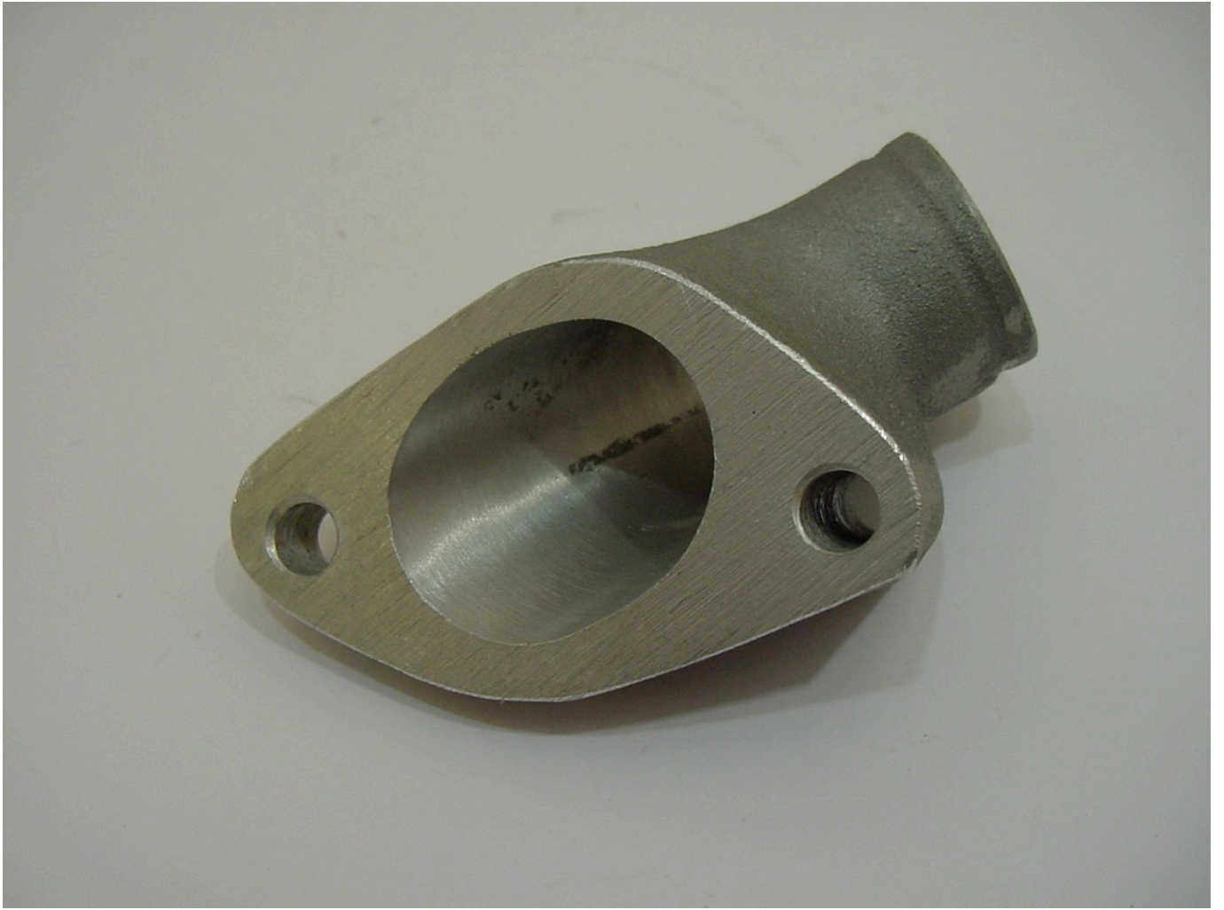
Flowed MB small block inlet for 25mm carbs
