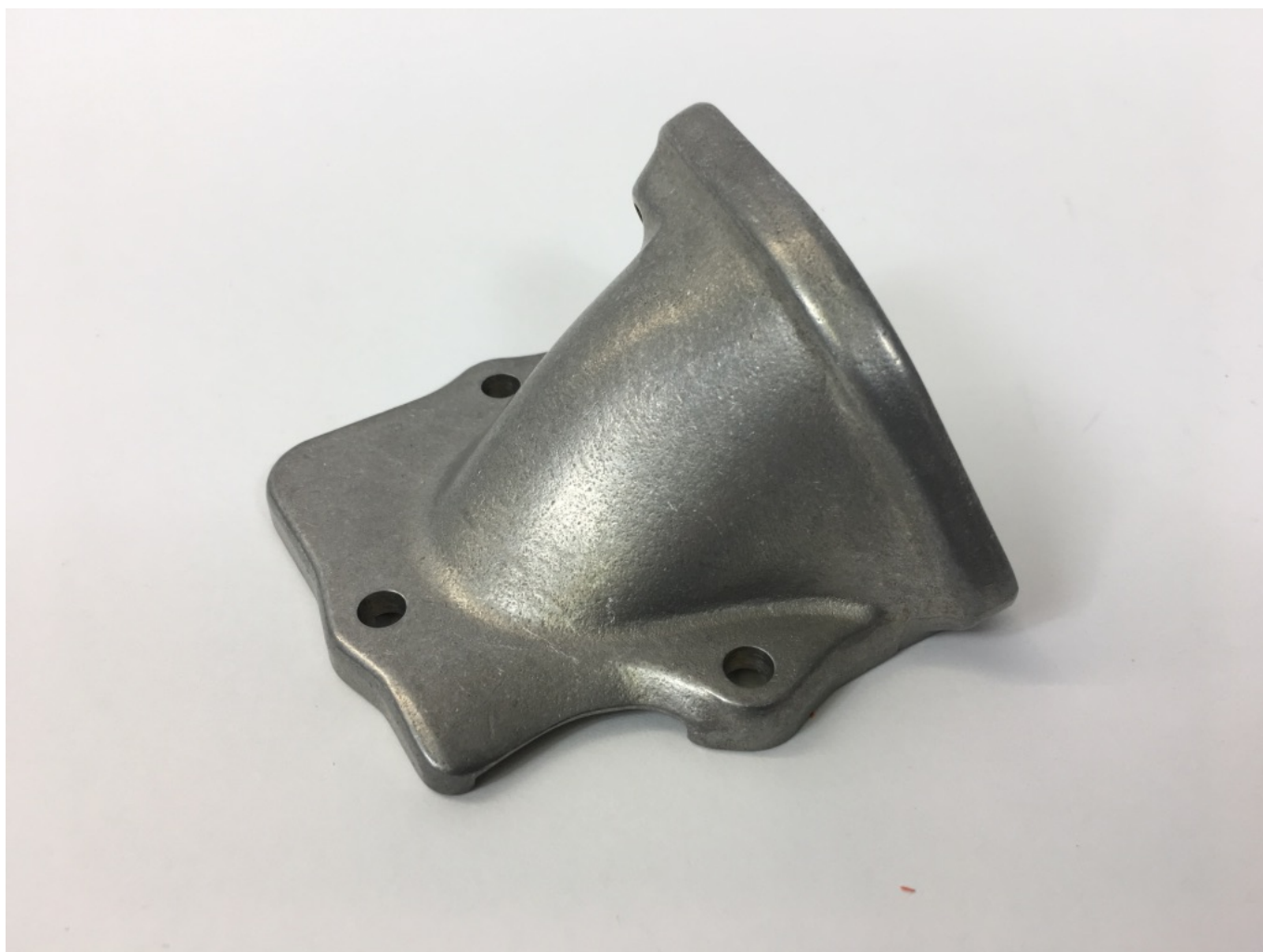
MB sand cast inlet to suit large block cylinders using 34,36mm Dellortos
