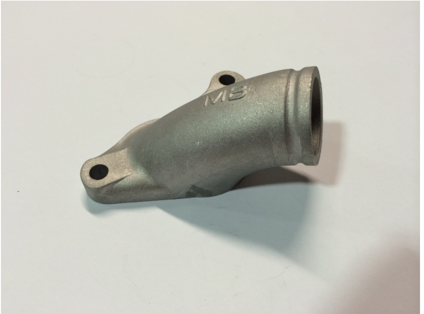
MB die cast large block Dellorto inlet, this version we used for cutdowns and bikes with panels off
