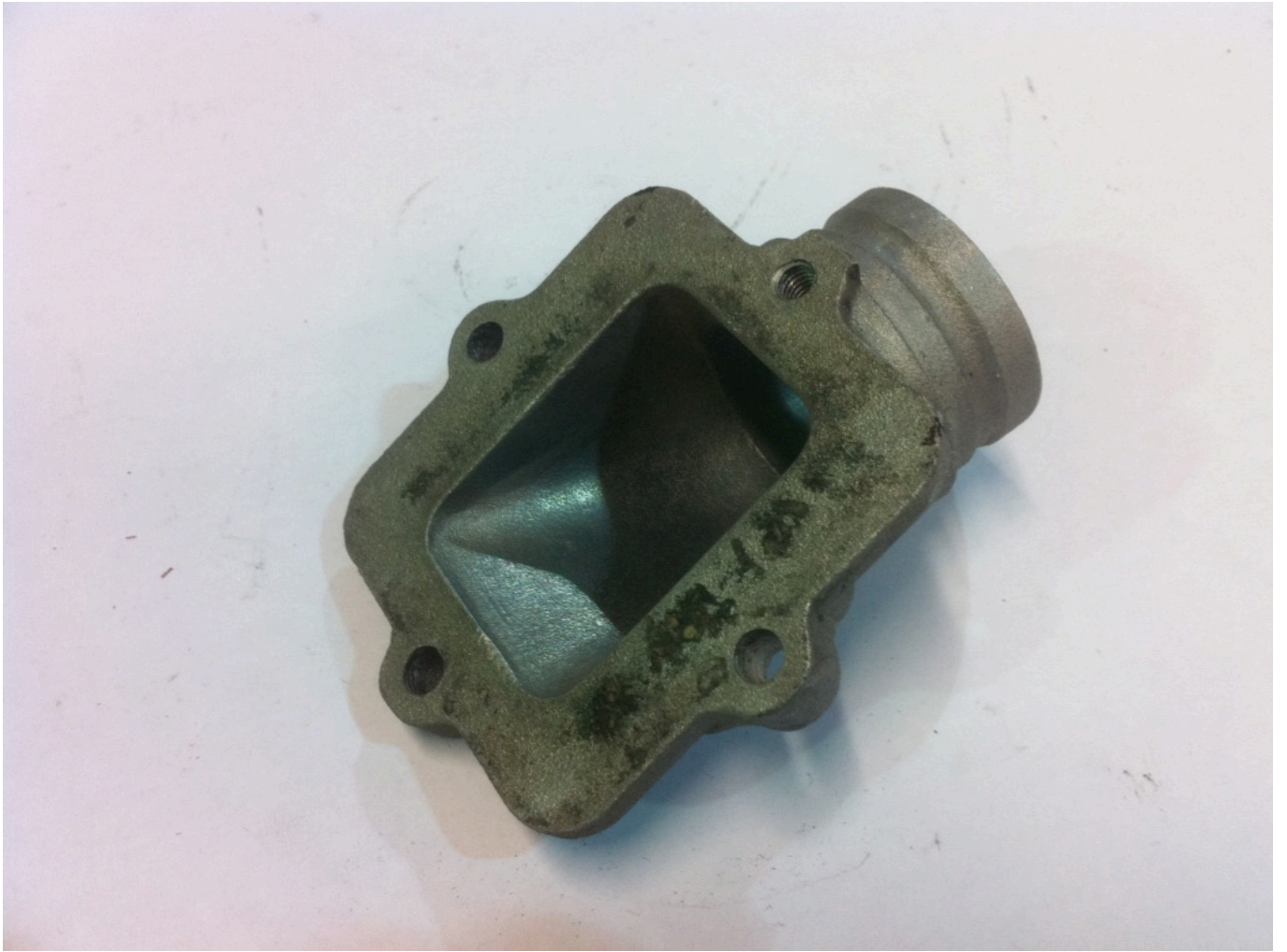
AF Rayspeed inlet, note no stuffer built in
