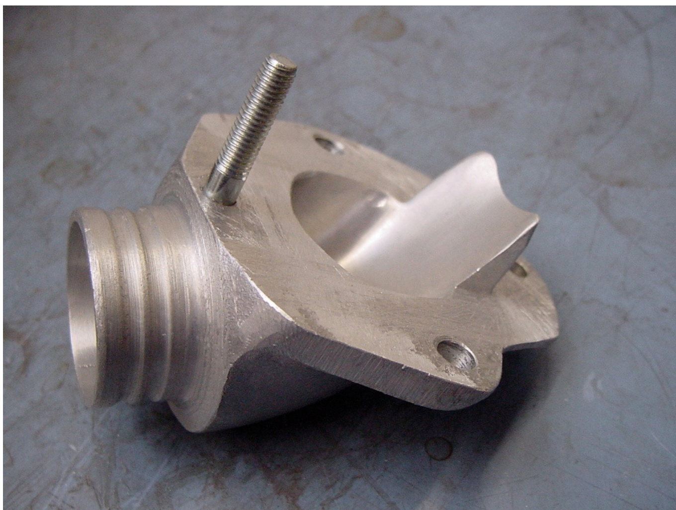
1980s MB Sand cast 6 petal reed assembly, 2 rubbers for different carbs
