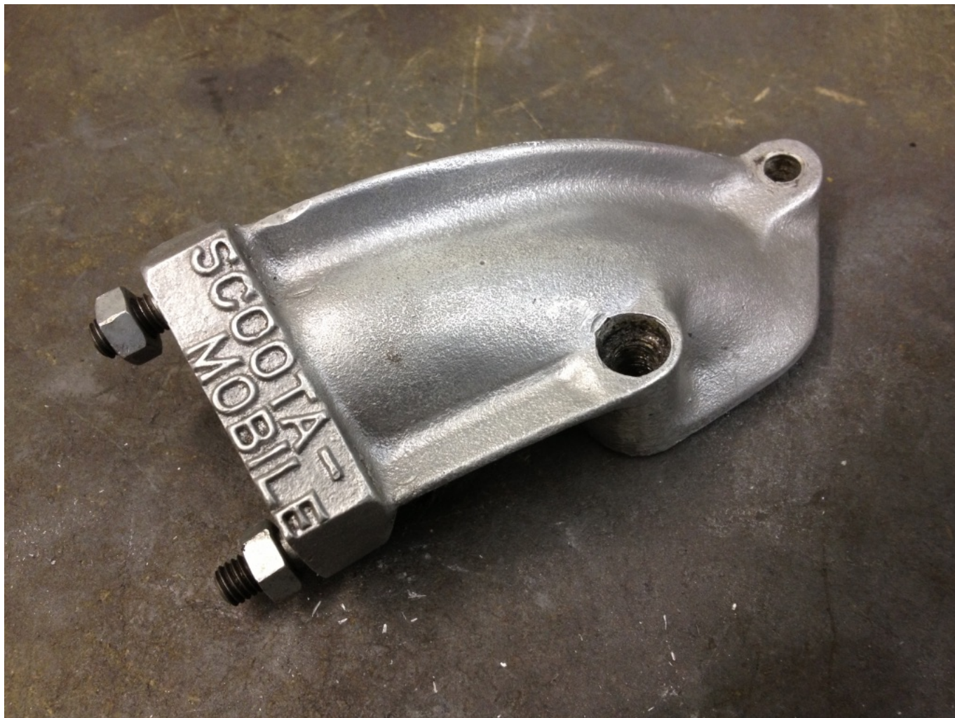
1960s Scoota Mobile Amal mark 1 sand cast inlet manifold
