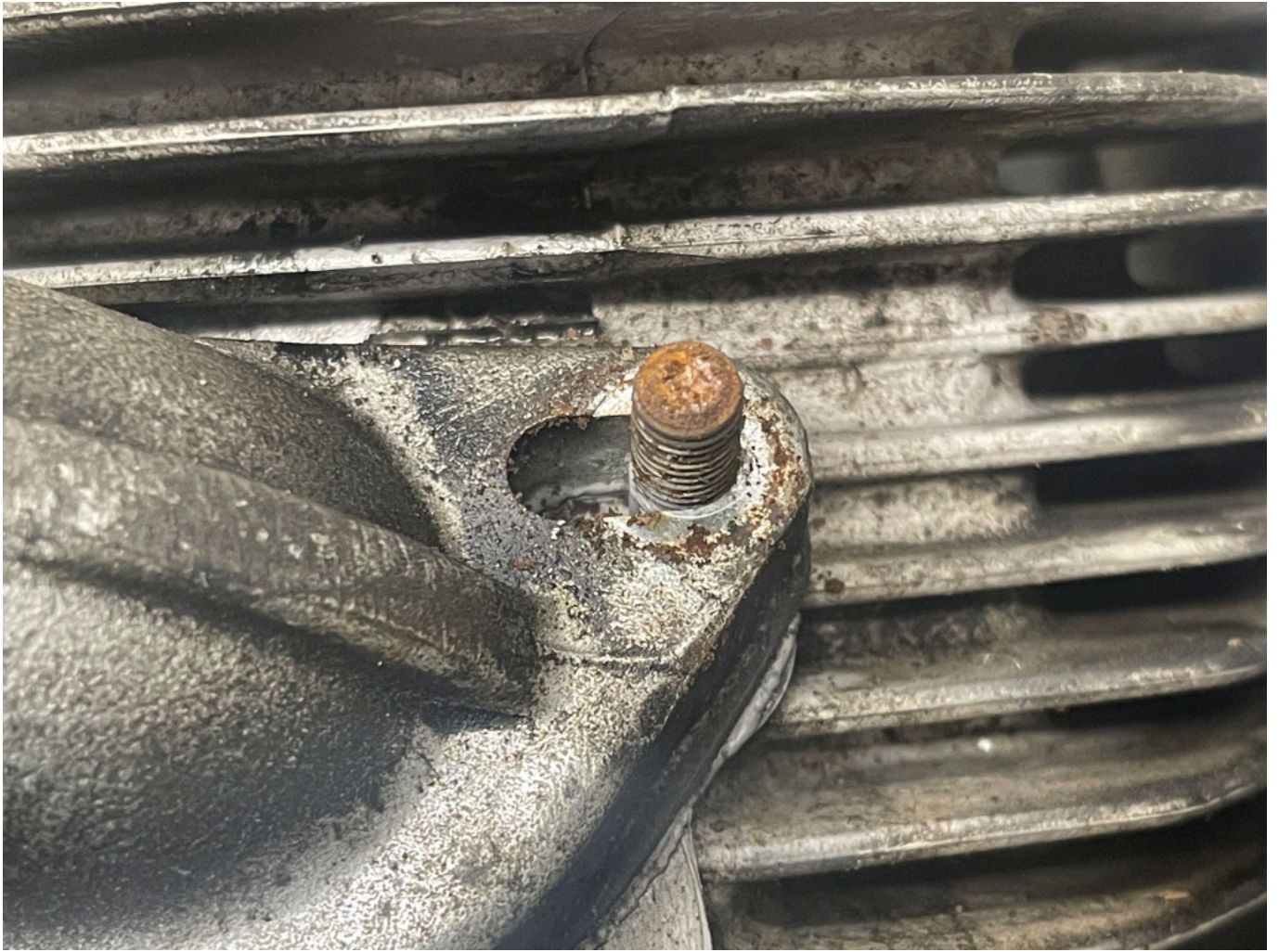
Mugello inlet manifold with a slot to suit small and large block but be careful with these
