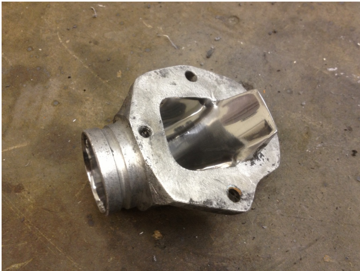
Early sand cast MB TS1 inlet, flowed, not one finger which fits into the reed assembly as a stuffer, fitted Amal and Mikuni
