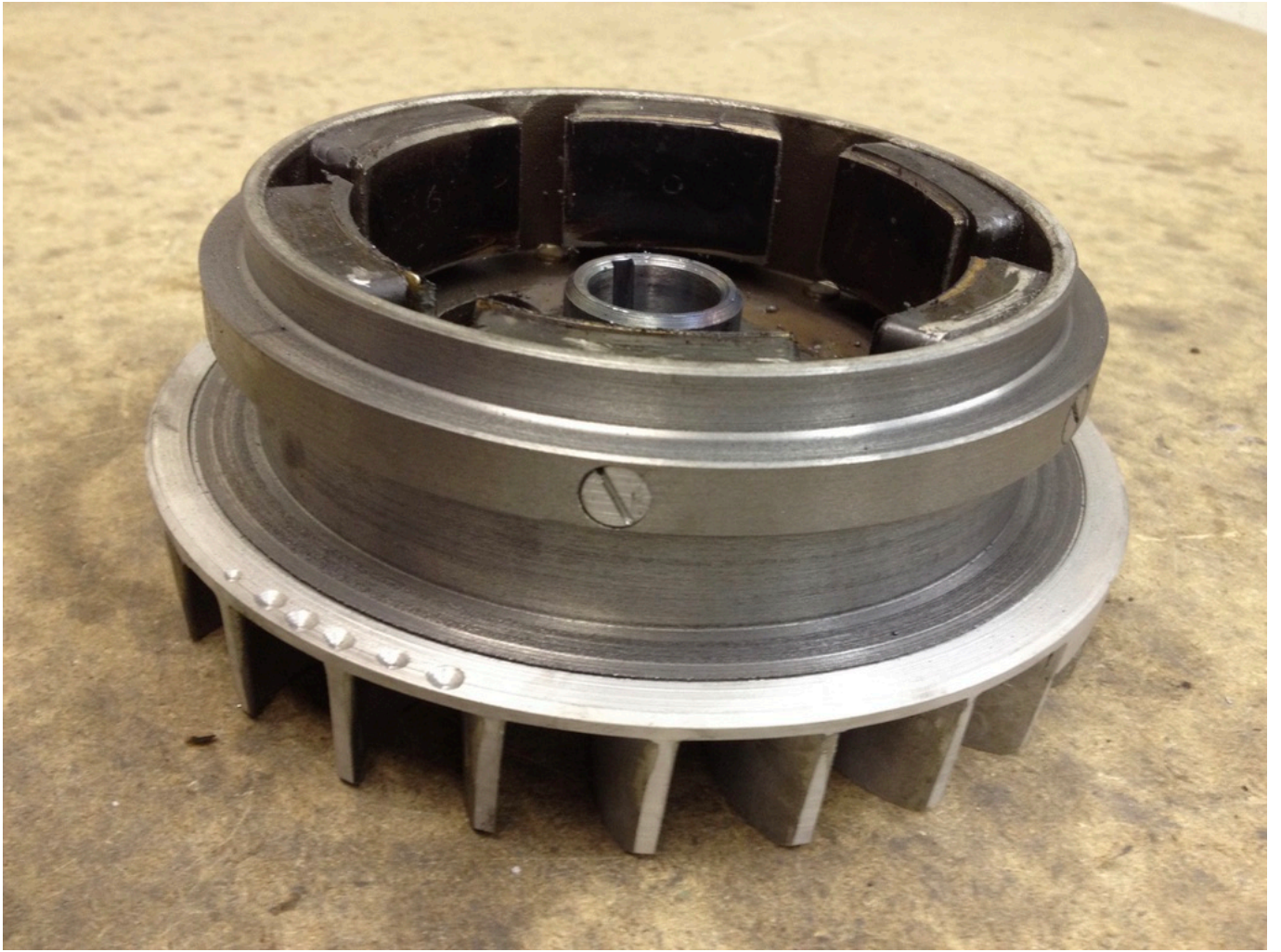
SIL flywheel, lightened by MB before Elemec brought out the mid flywheel
