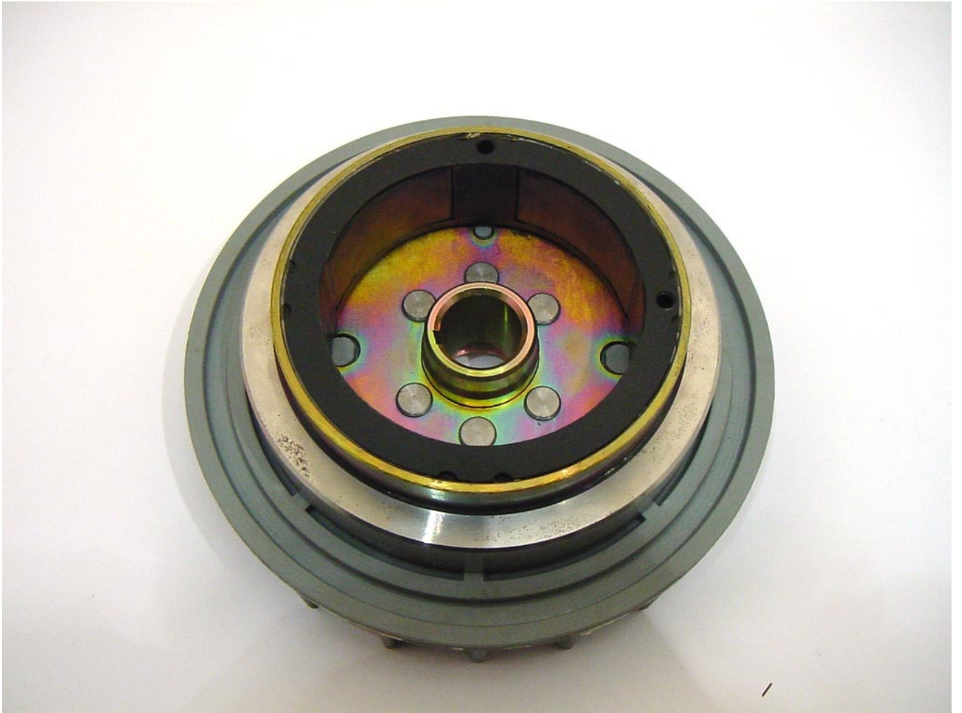
Varitronic flywheel Gp type insert the magnets
