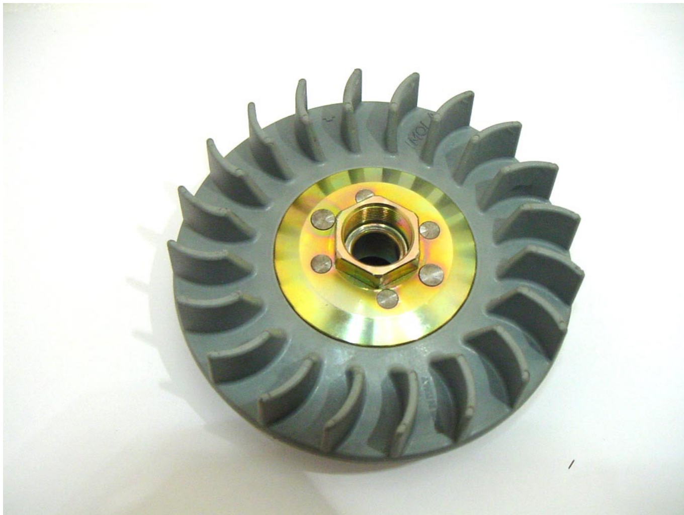
Varitronic outside showing plastic fins, this is an early type
