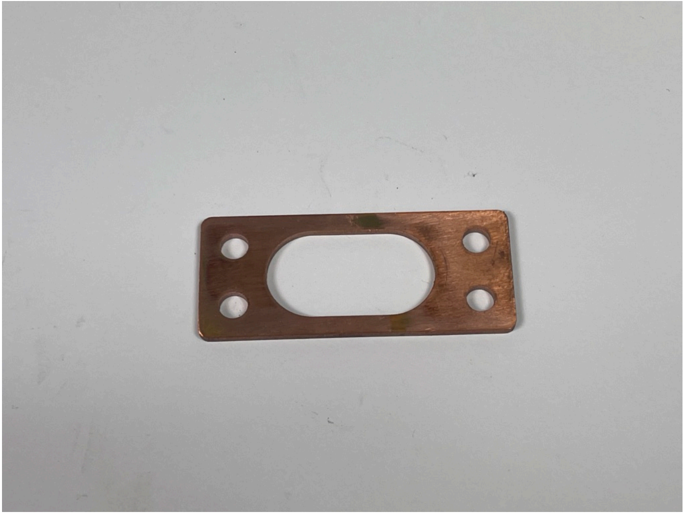
MB oval exhaust gasket in copper, note the gap positioning of the oval to the stud holes, these only fit one way
