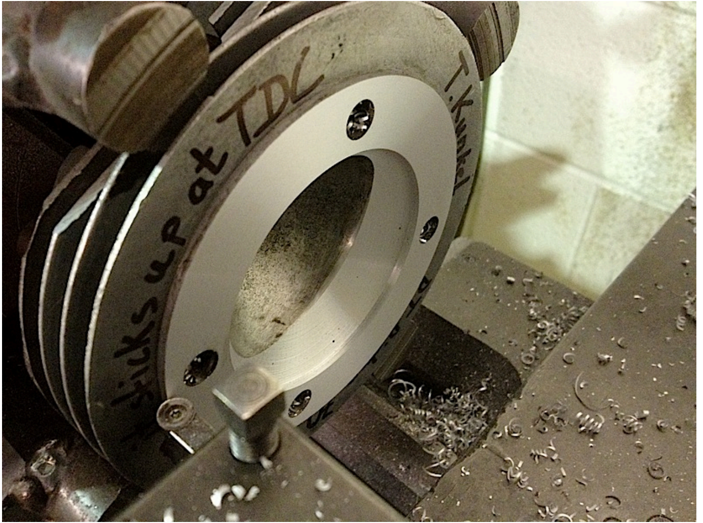
The face is cleaned off to get the recess correctly for the piston and 60mm stroke
