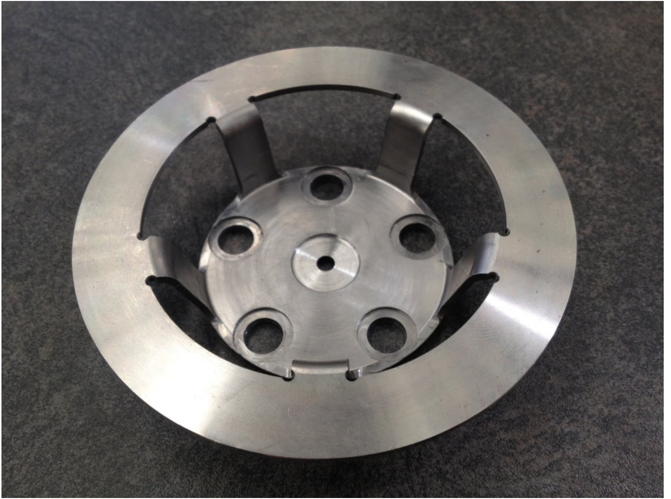
MB CNC pressure plate, note the recesses for the clutch springs
