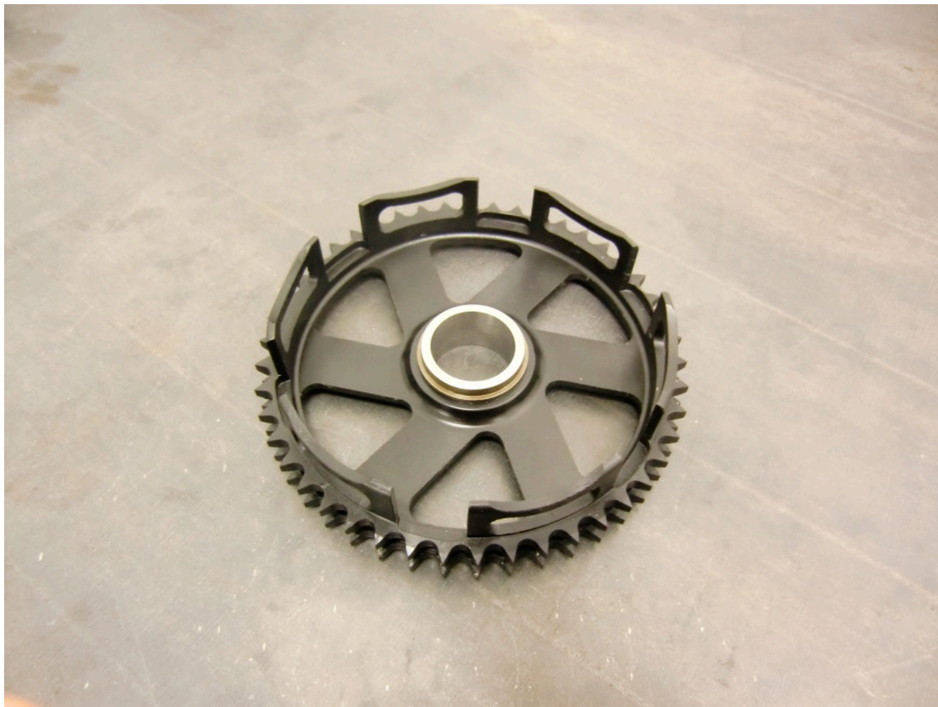
MB lightened 46/47 tooth crownwheels, some had a loose pressed in inner bearing some were one piece
