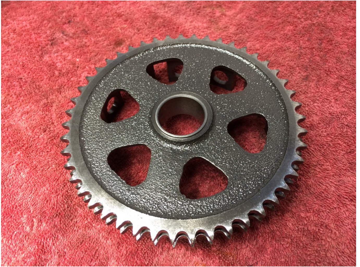
Rough casting for the crownwheel
