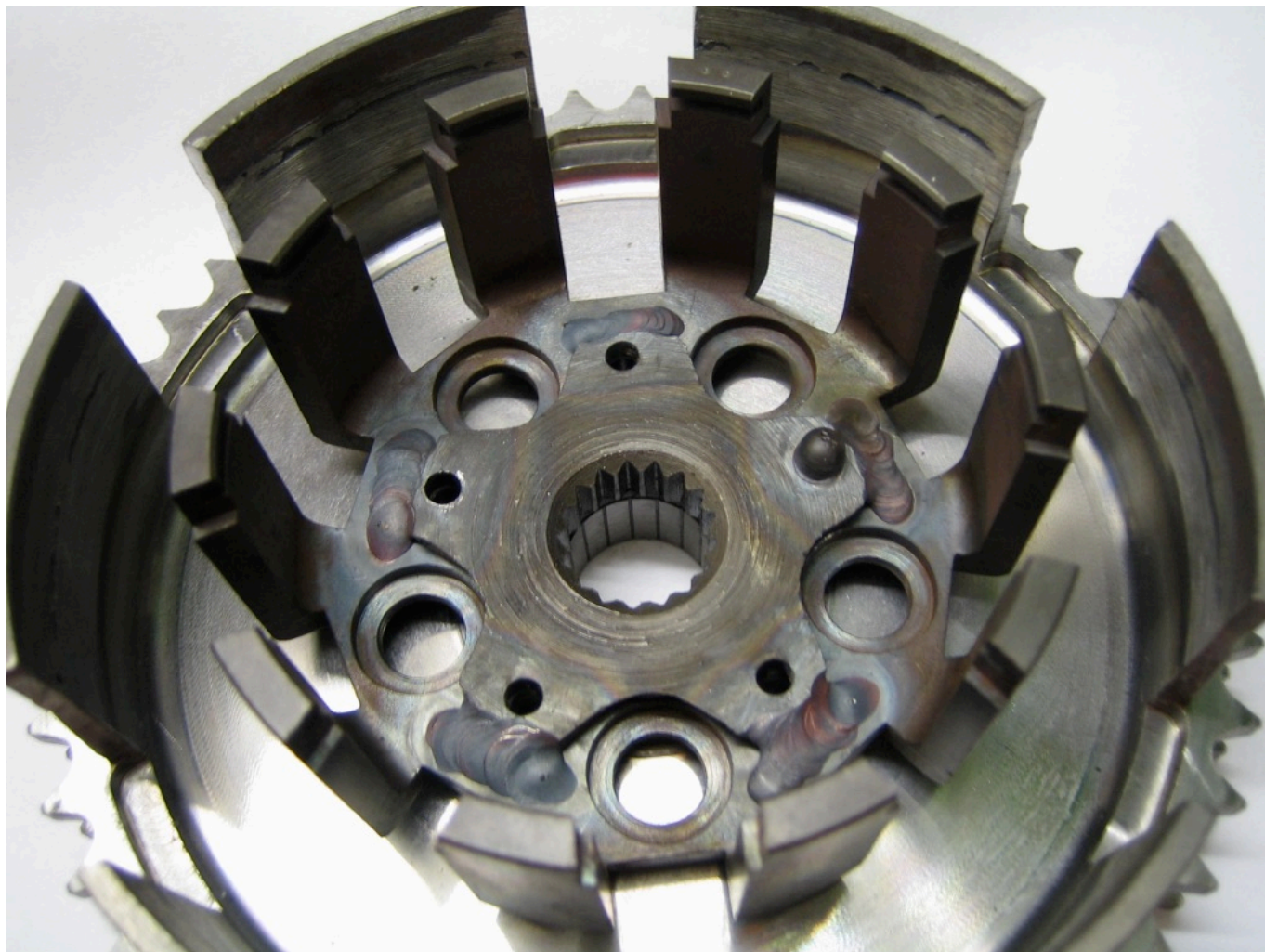
Early MB external clutch, which used a 10mm crankcase side packer
