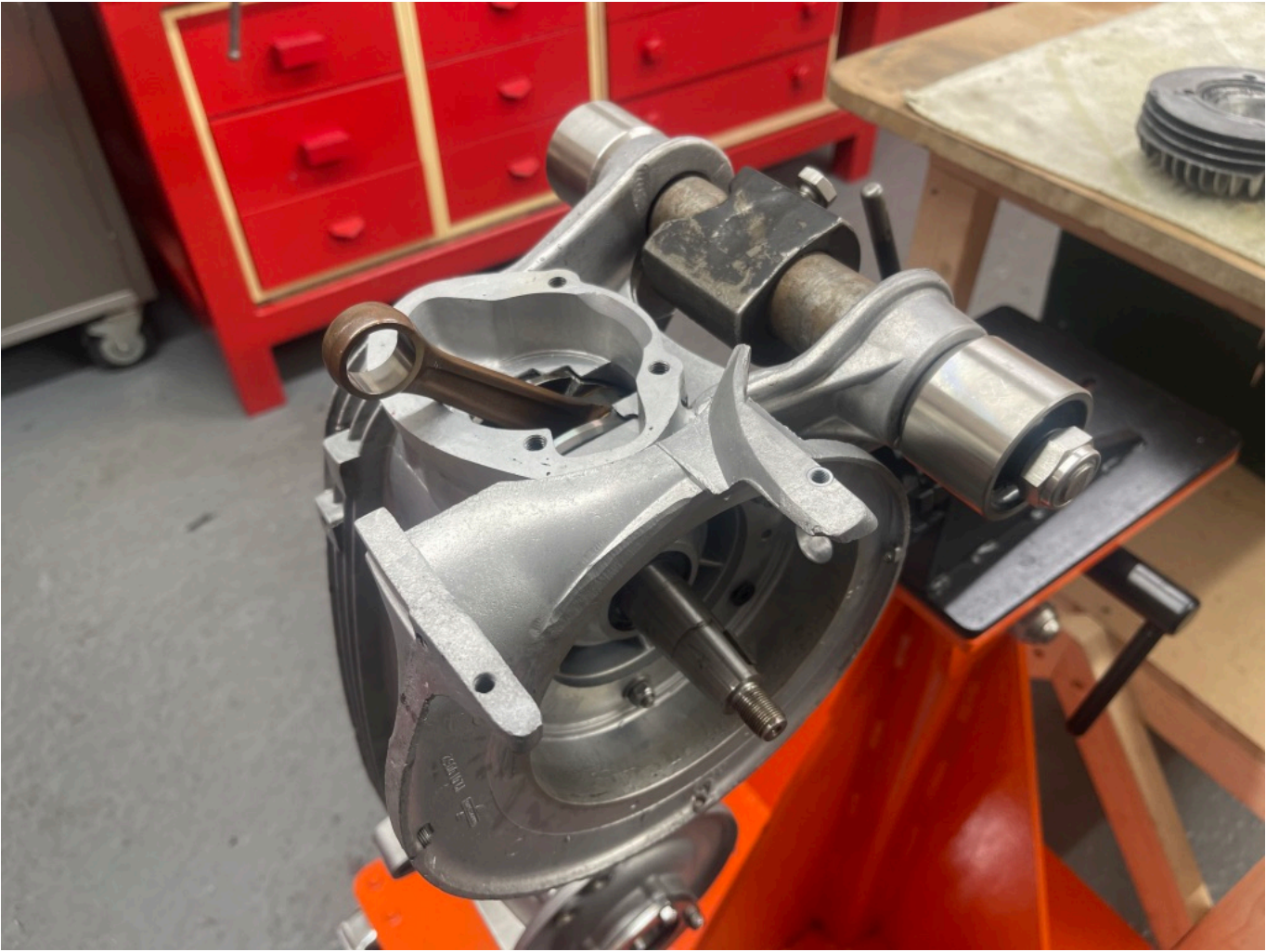
Crank fitted and turning free, ready for the rebuild
