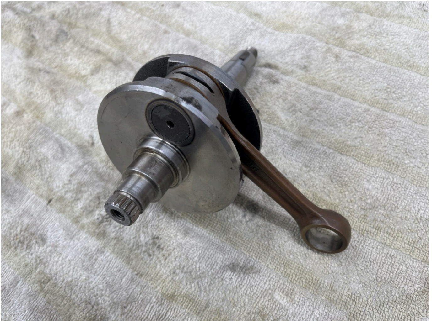
60mm x 115mm con rod MB conversion from the 90's
