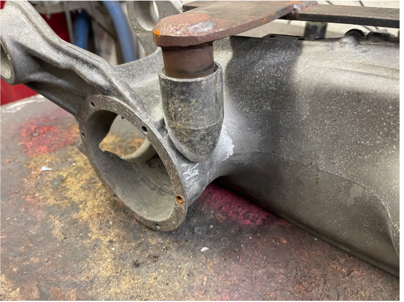
Donor engine lug fitted with our fixture
