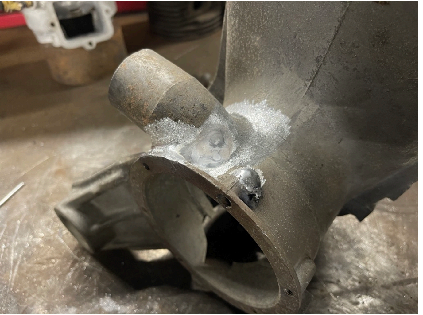
More welding to fill in any blow holes
