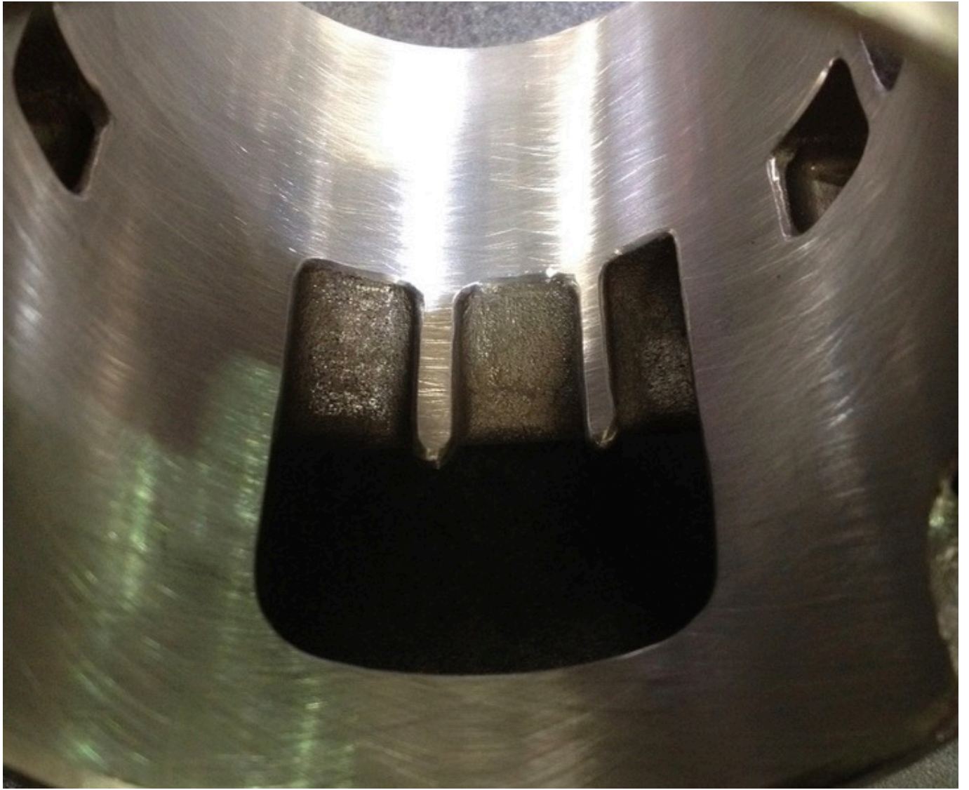
3 boost ports in the RB 250 cylinder
