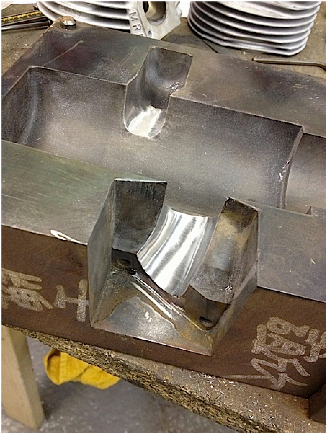
Both inlet and exhaust port was modified as was the transfer ports
