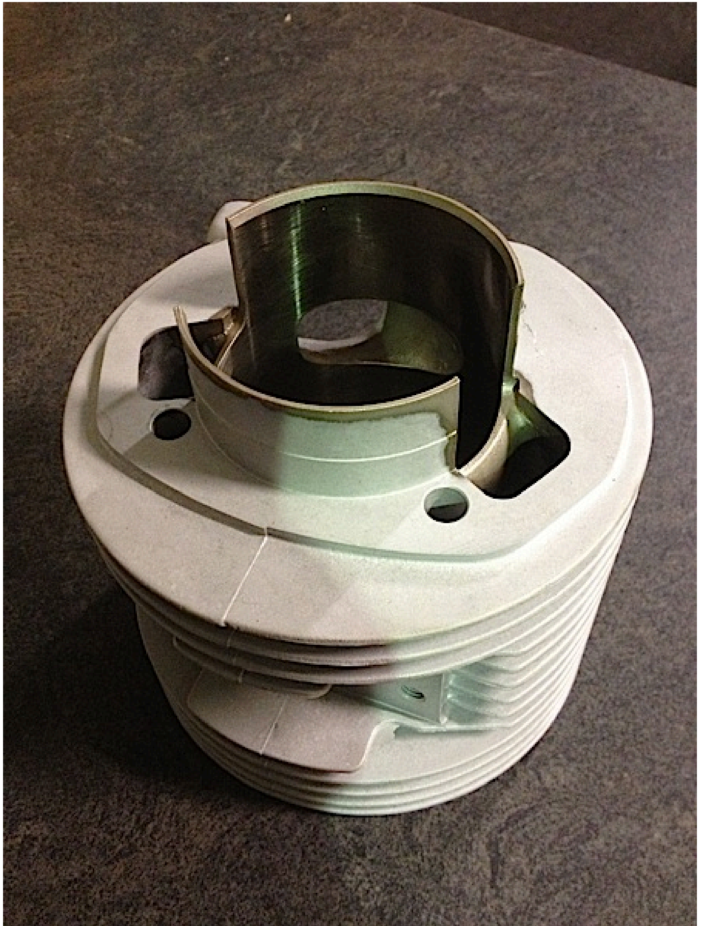
The MBgm cylinders have a rounded port compared to the MBD version with a square shaped port
