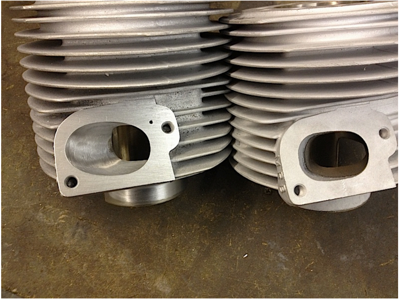
On the left a matched and flowed inlet port and standard on the right – note the thick top section with extra cooling fin
