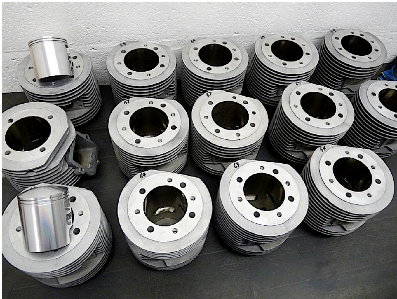
A pile of finished, plated RT cylinders ready for bagging and boxing
