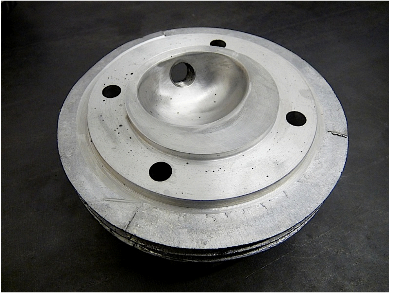
The MB drop head design to locate the head and stop the head gasket blowing, now copied by others
