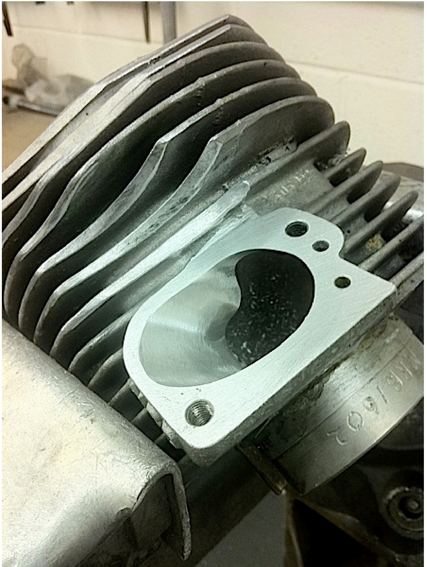
A MB RT 255 reed inlet port, matched and flowed to a reed block, MRB1602, note two holes in the face, this was originally done for a LTH Reed block which is slotted and these were locating pegs to centralise the block, note
