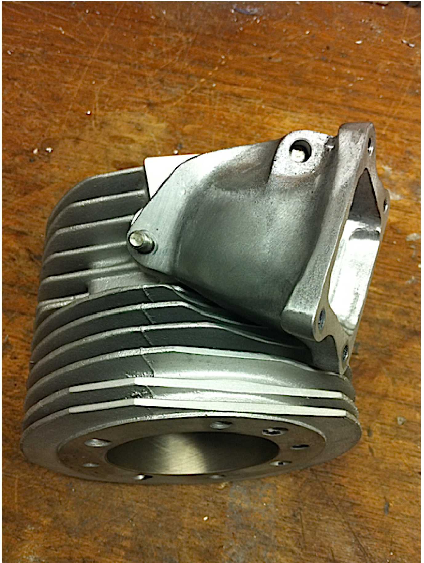
A modified MB RT cylinder with the Shorty Reed block fitted
