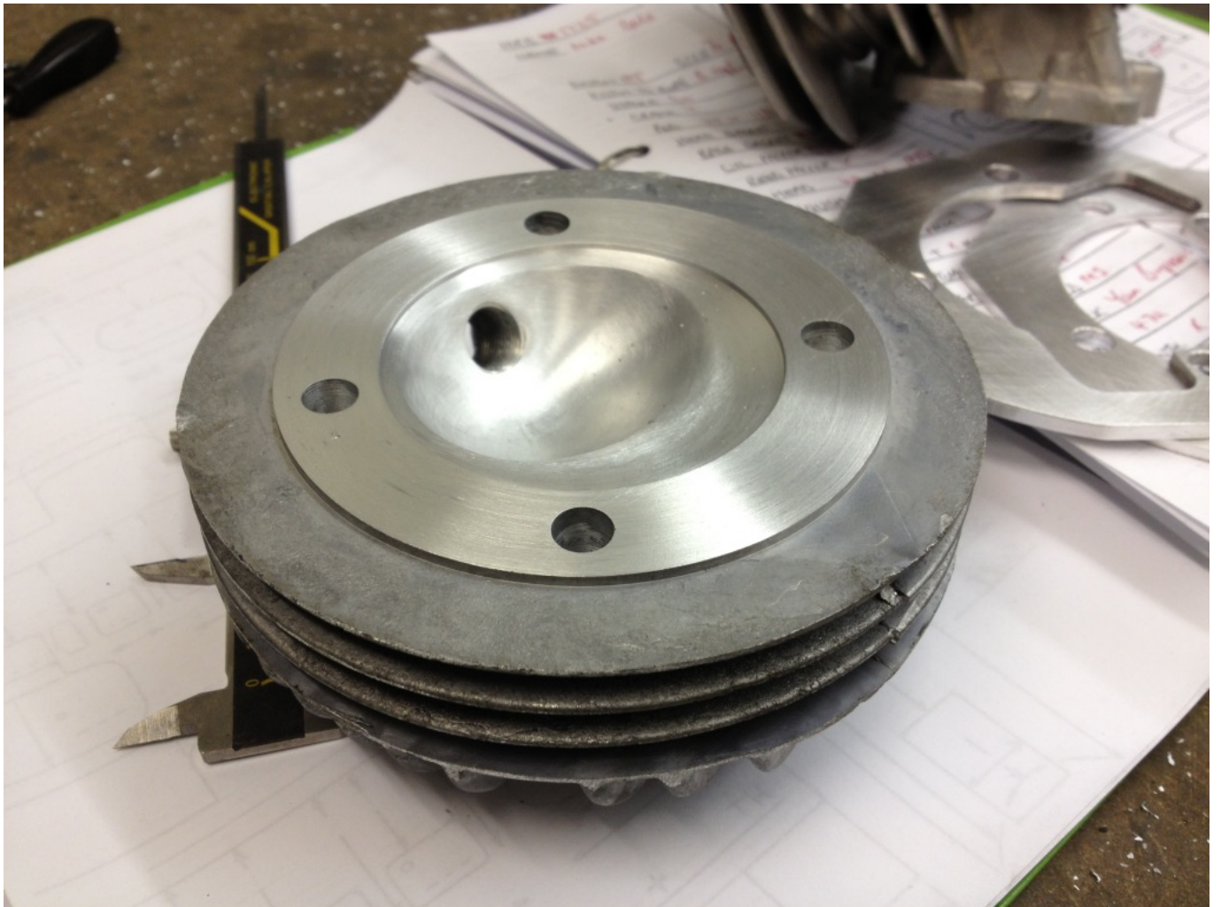
This is a remade 200 head modified for a Ts1 using a 60mm
