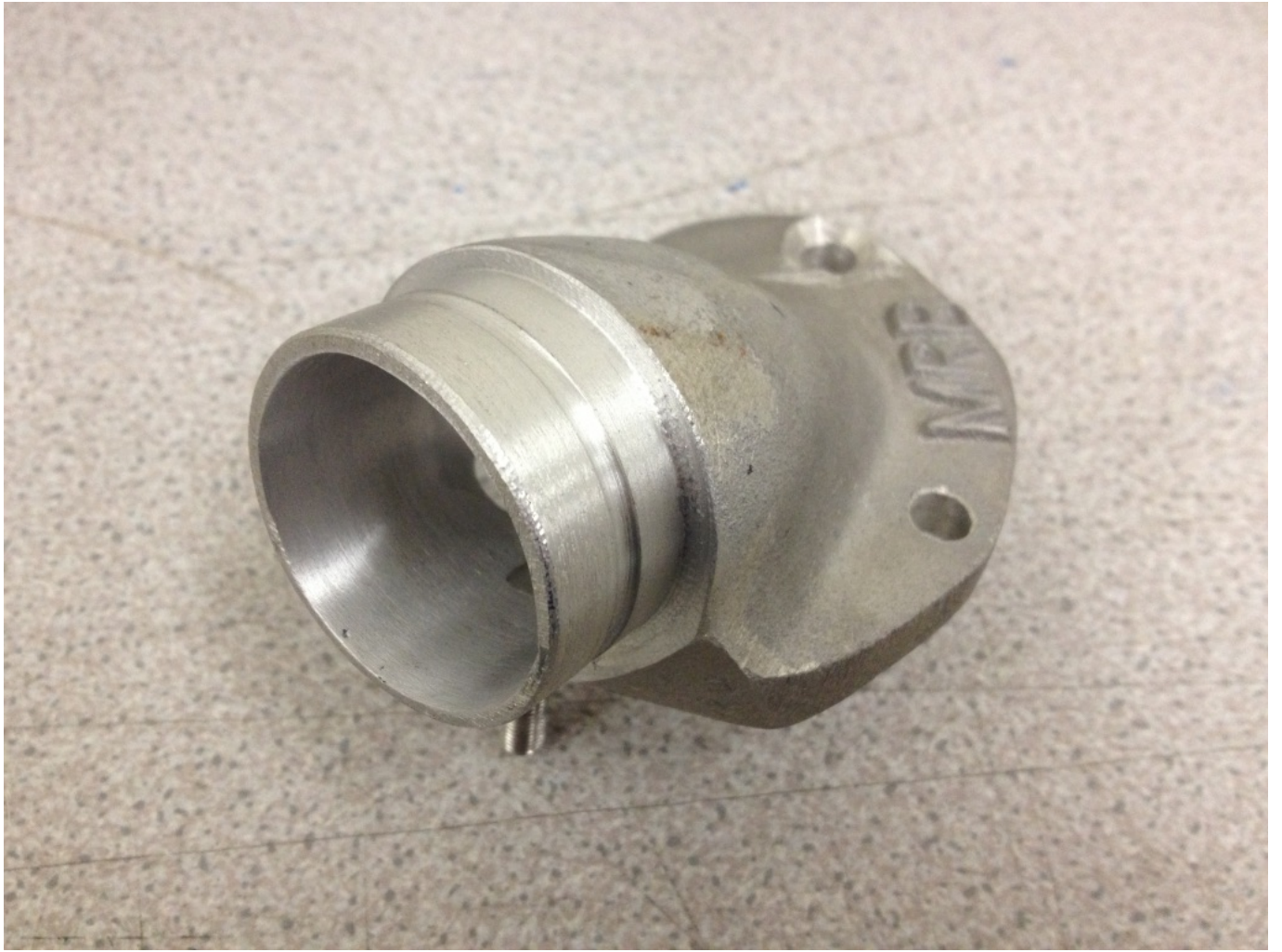
Early sand cast inlet flowed and machined to suit an Amal carb
