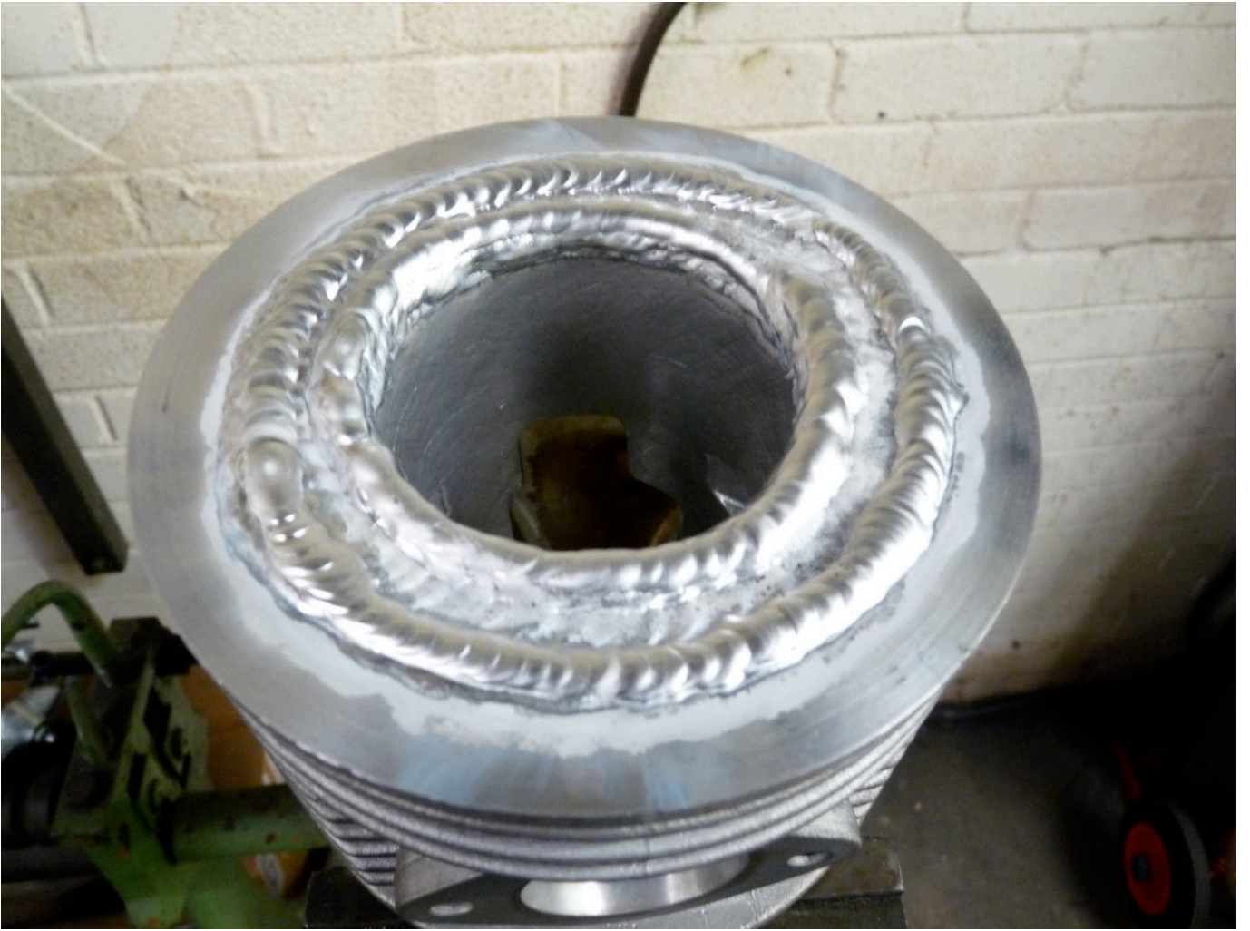
Once welded in needs machining
