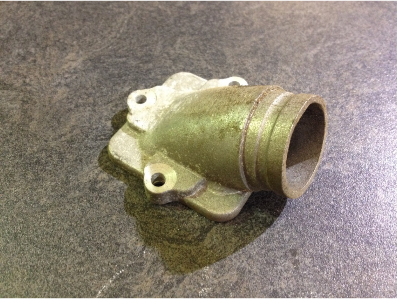
AF inlet manifold, which never changed but others did make manifolds
