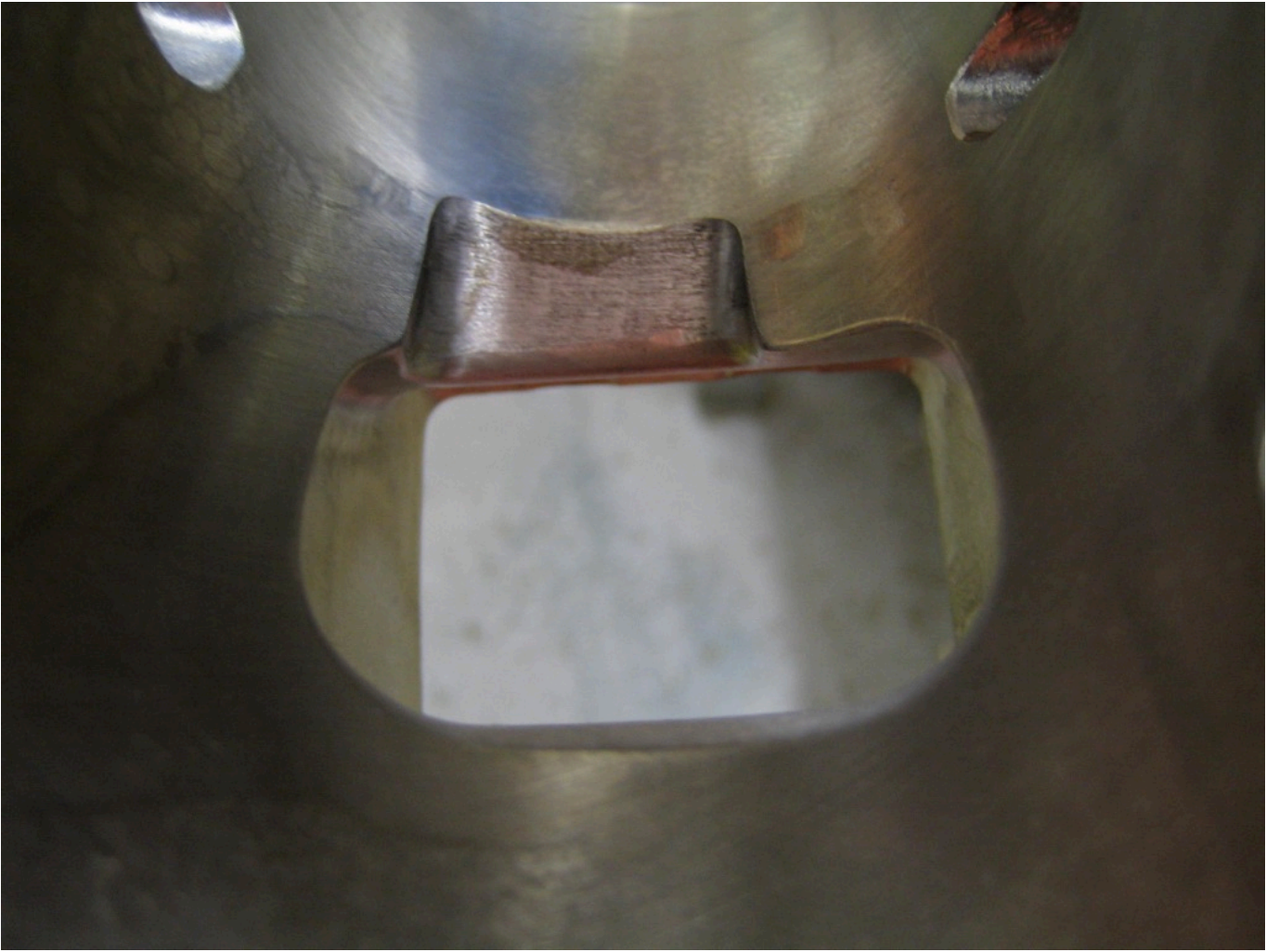
Standard type Ts1 inlet and boost port
