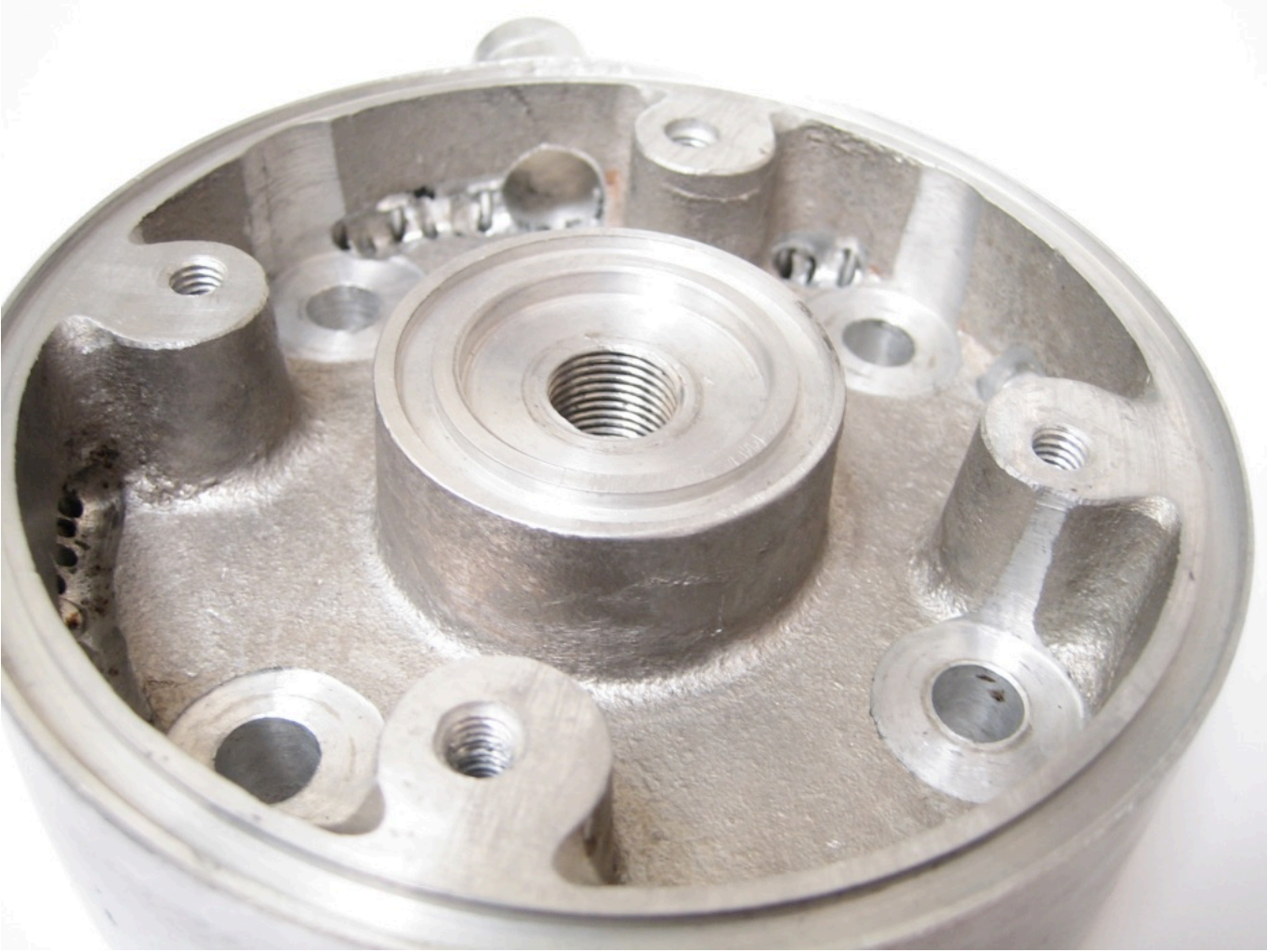
These are sand cast, heat treated, then machined to spec in house
