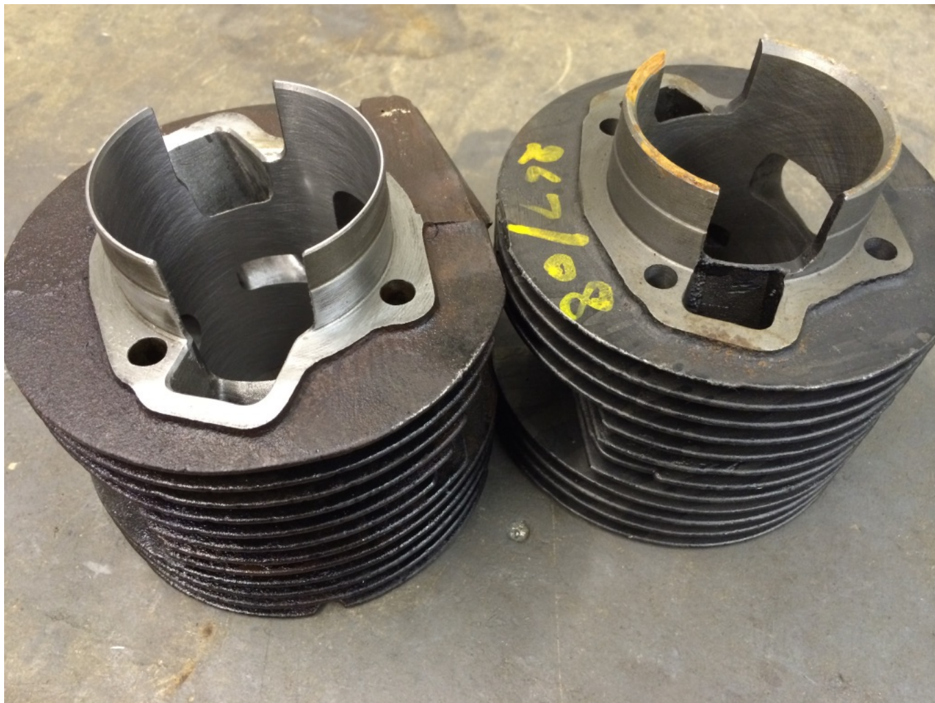
Tuned transfer ports on the left standard on the right
