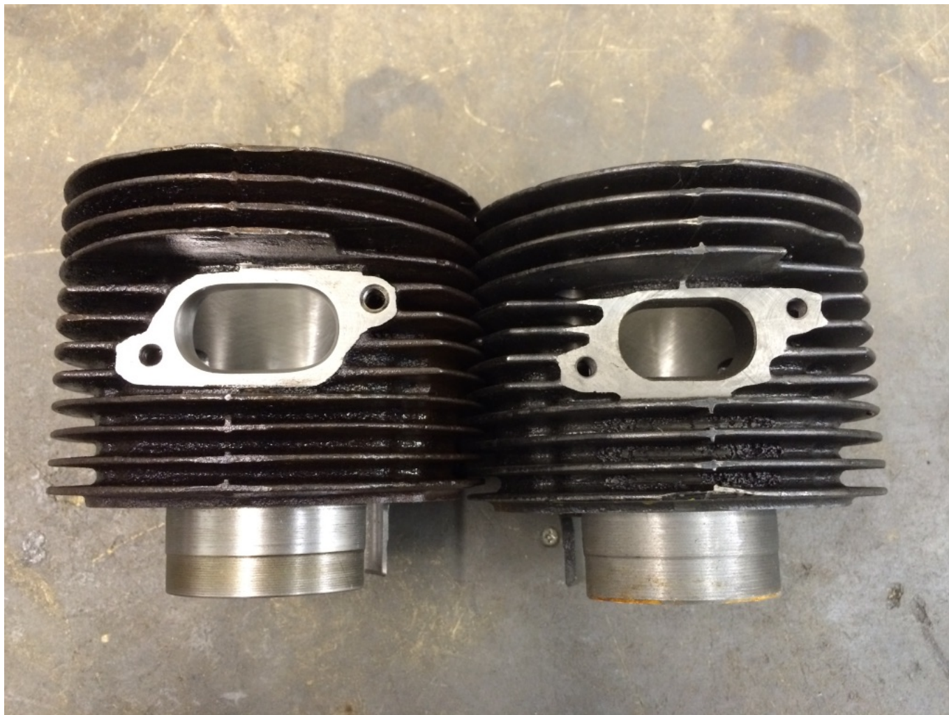
Tuned cylinder on the left standard SIL on the right
