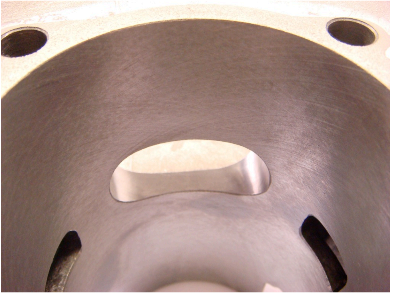
Tuned exhaust port from inside the bore
