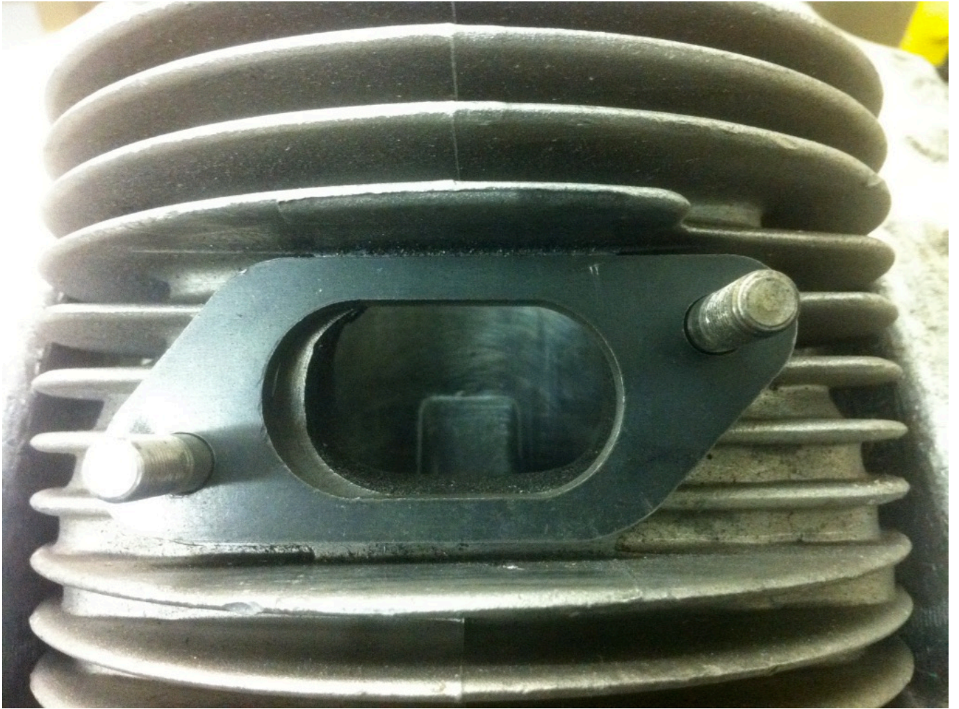
Another version mismatched to a correct exhaust flange
