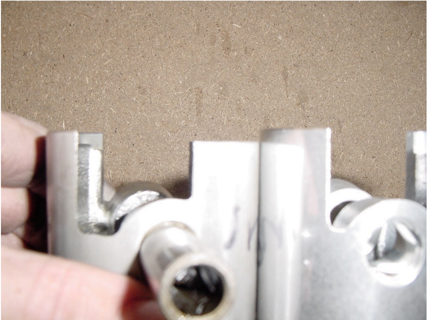
Shows the difference in inlet shirt lengths
