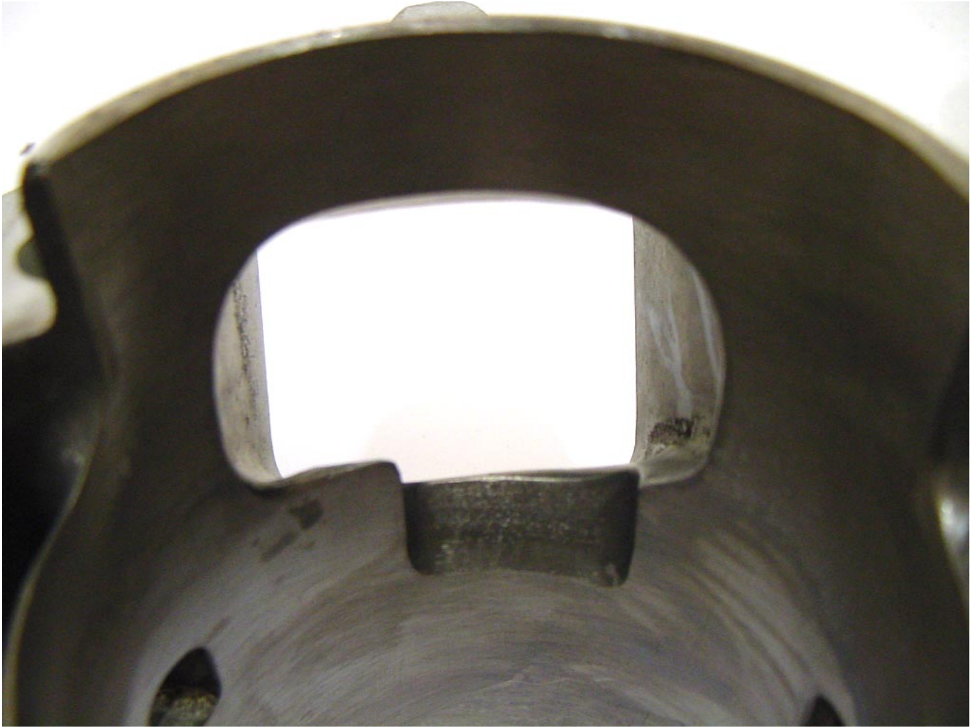
A Monza inlet port opened with reed boost port re tuned from original
