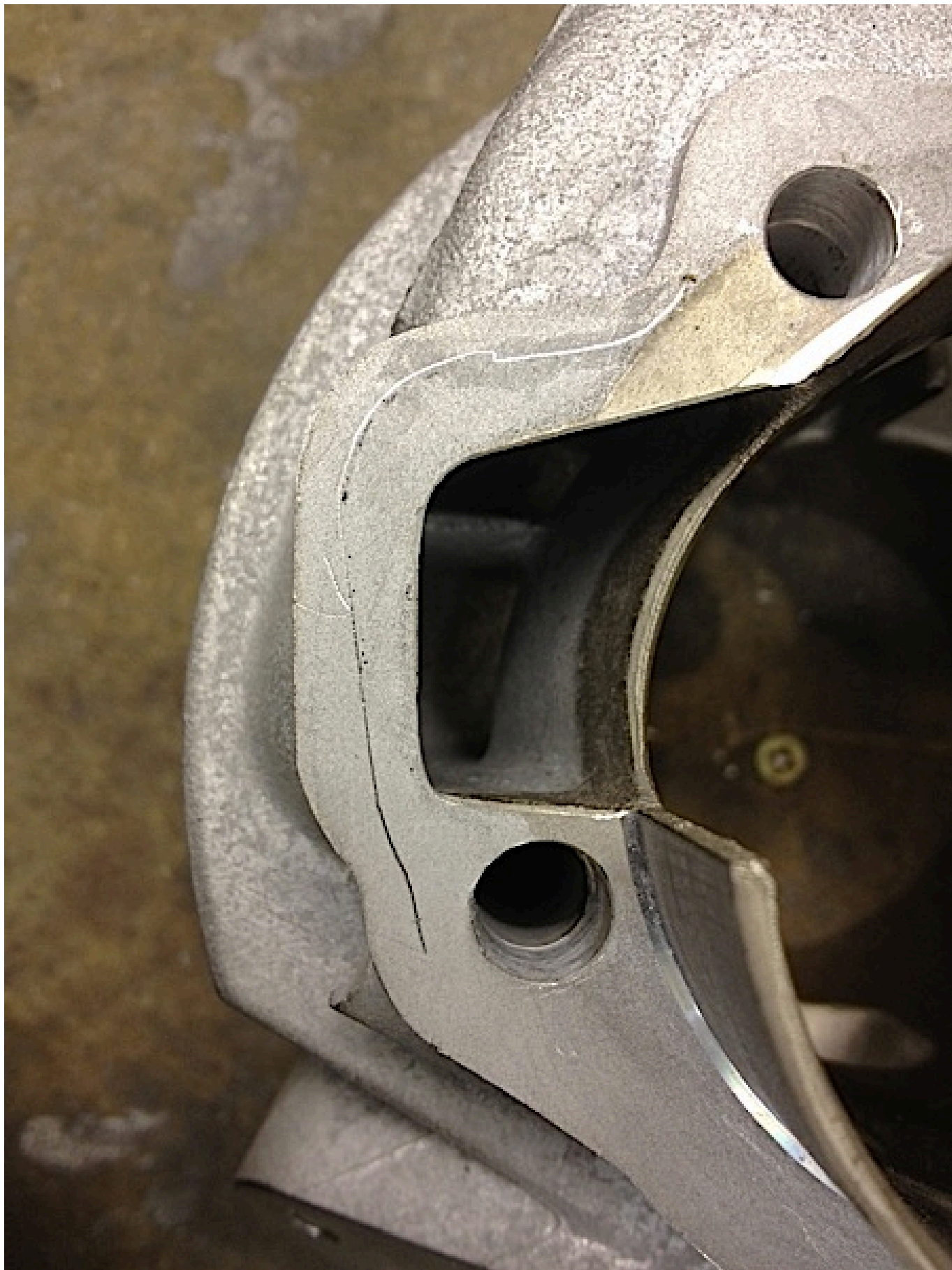
Shows where a standard Italian casing is and how much can be machined out
