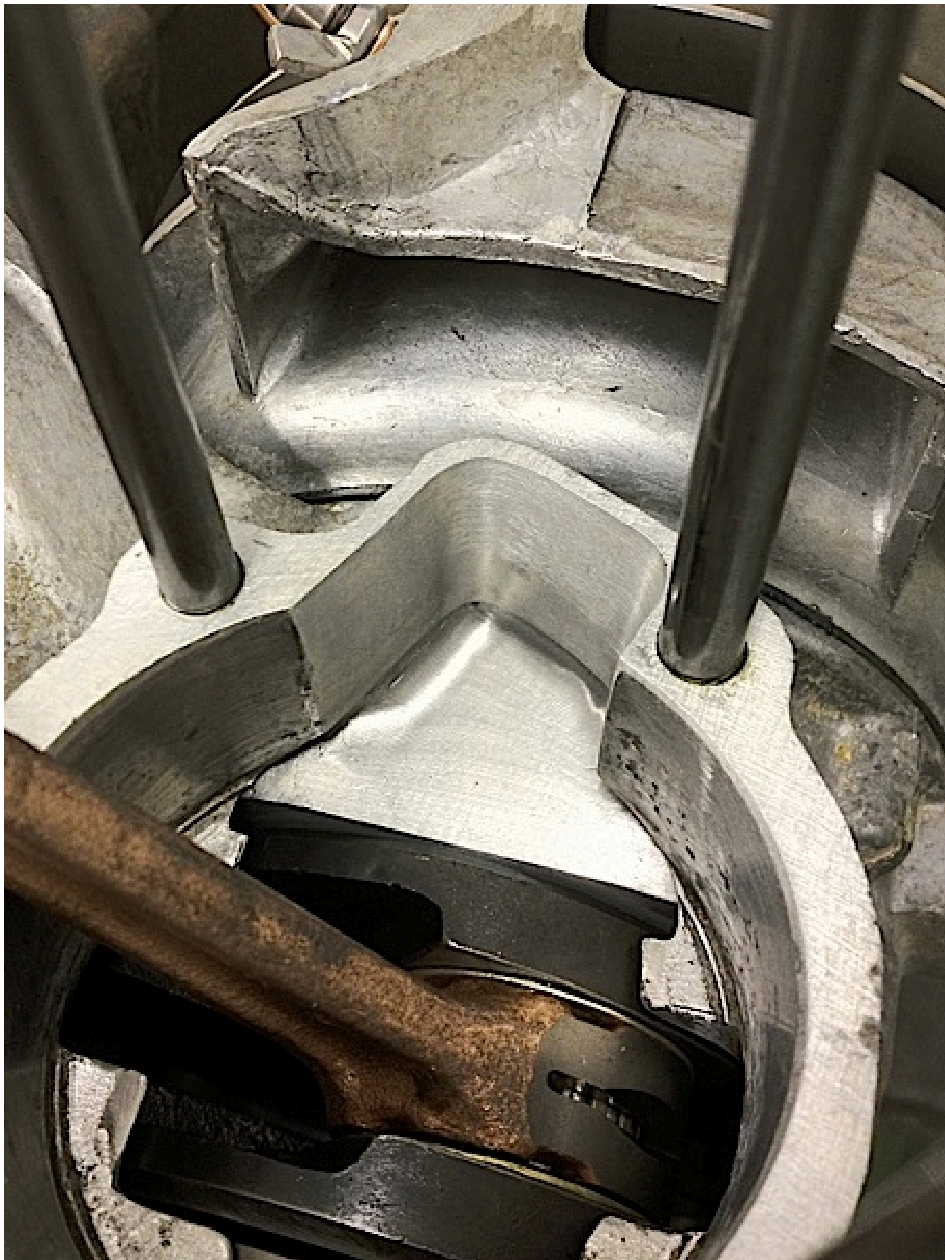
Transfers opened to the max in a bit of a dog of an old casing with a MB Yamaha 115 con rod conversion
