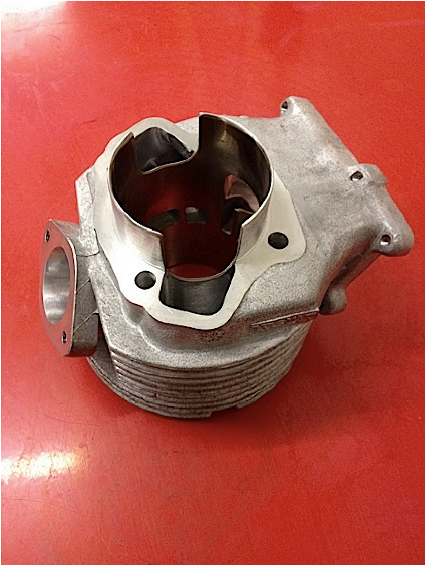
Machined base area and transfer matched and flowed, just needed the spigot altering in size
