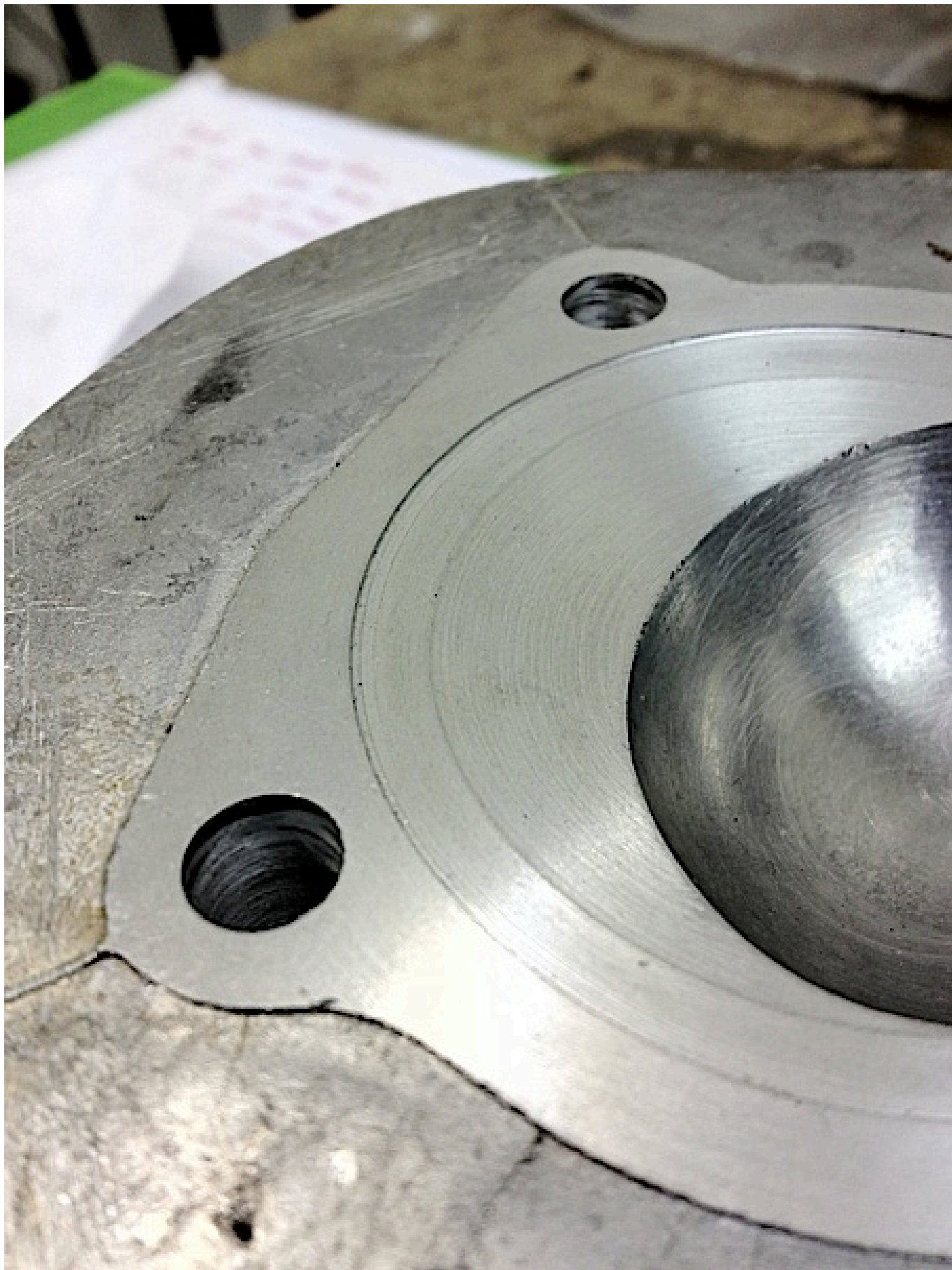
Strange standard head, recessed, and double cut
