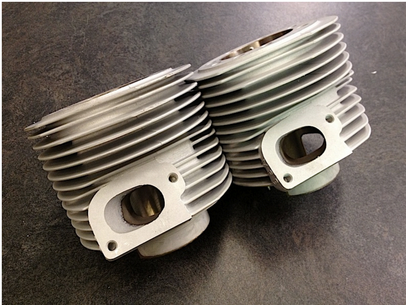
Left 1st batch prototype Right once the tooling was modified by Mark
