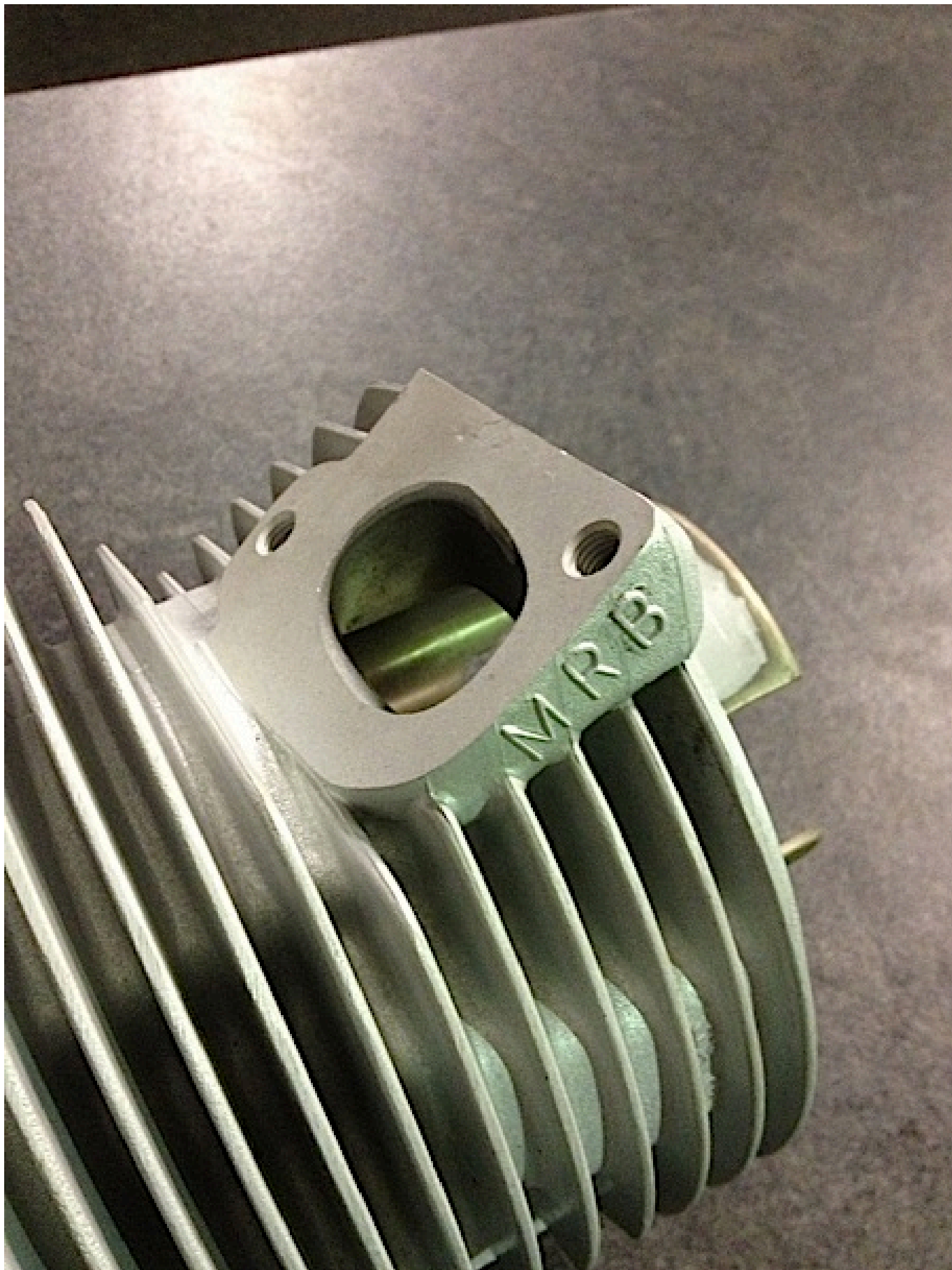
New MBgm cylinders are marked with MRB old ones are marked with MBD
