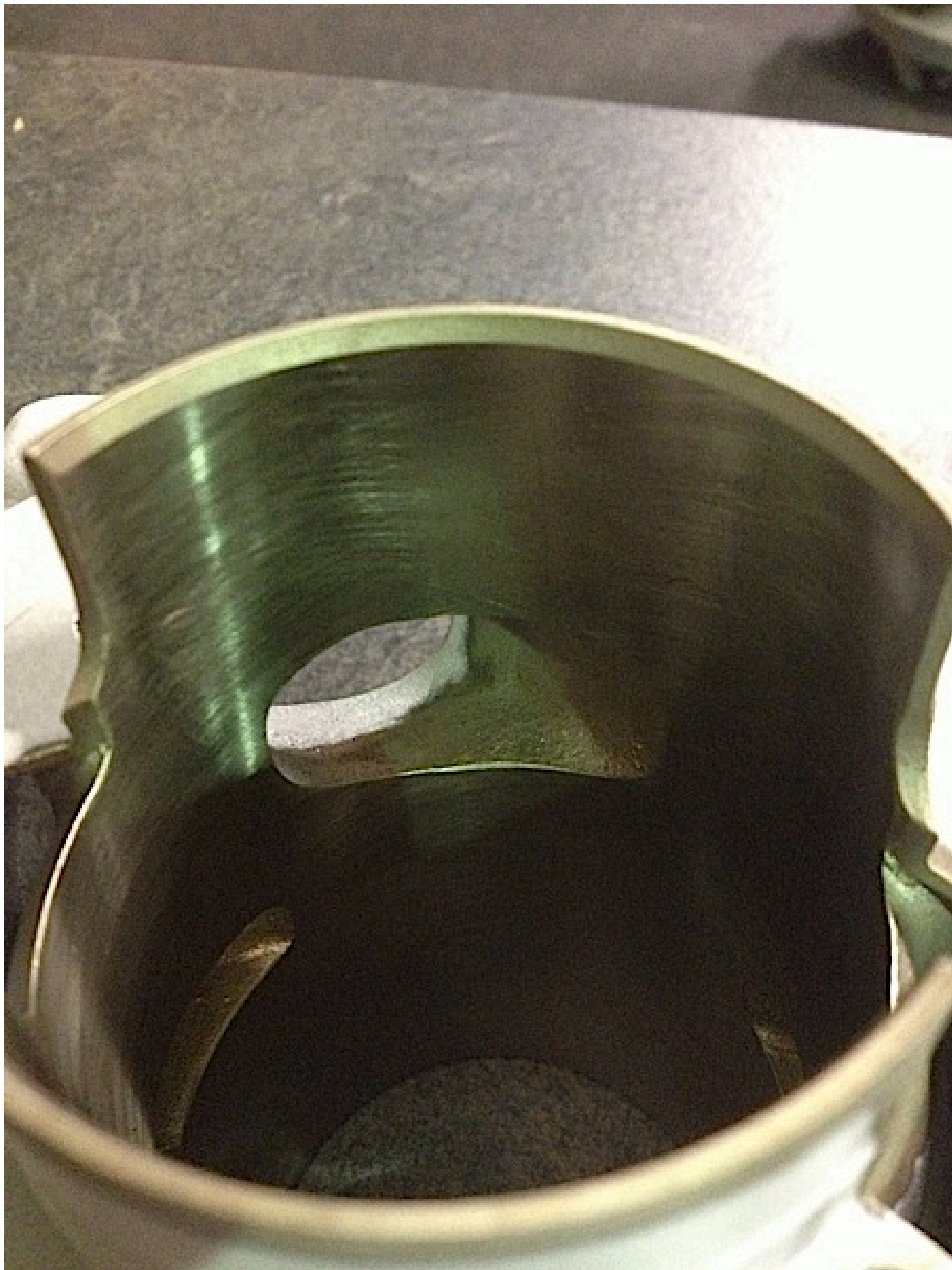
New rounded inlet port to improve piston life
