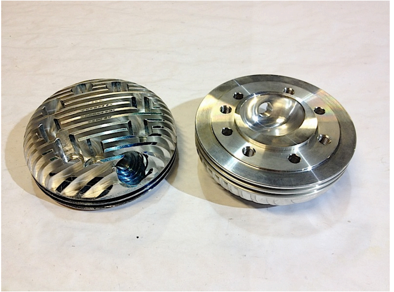
Prototype CNC heads with extra fins and extra cooling which fit with cowlings
