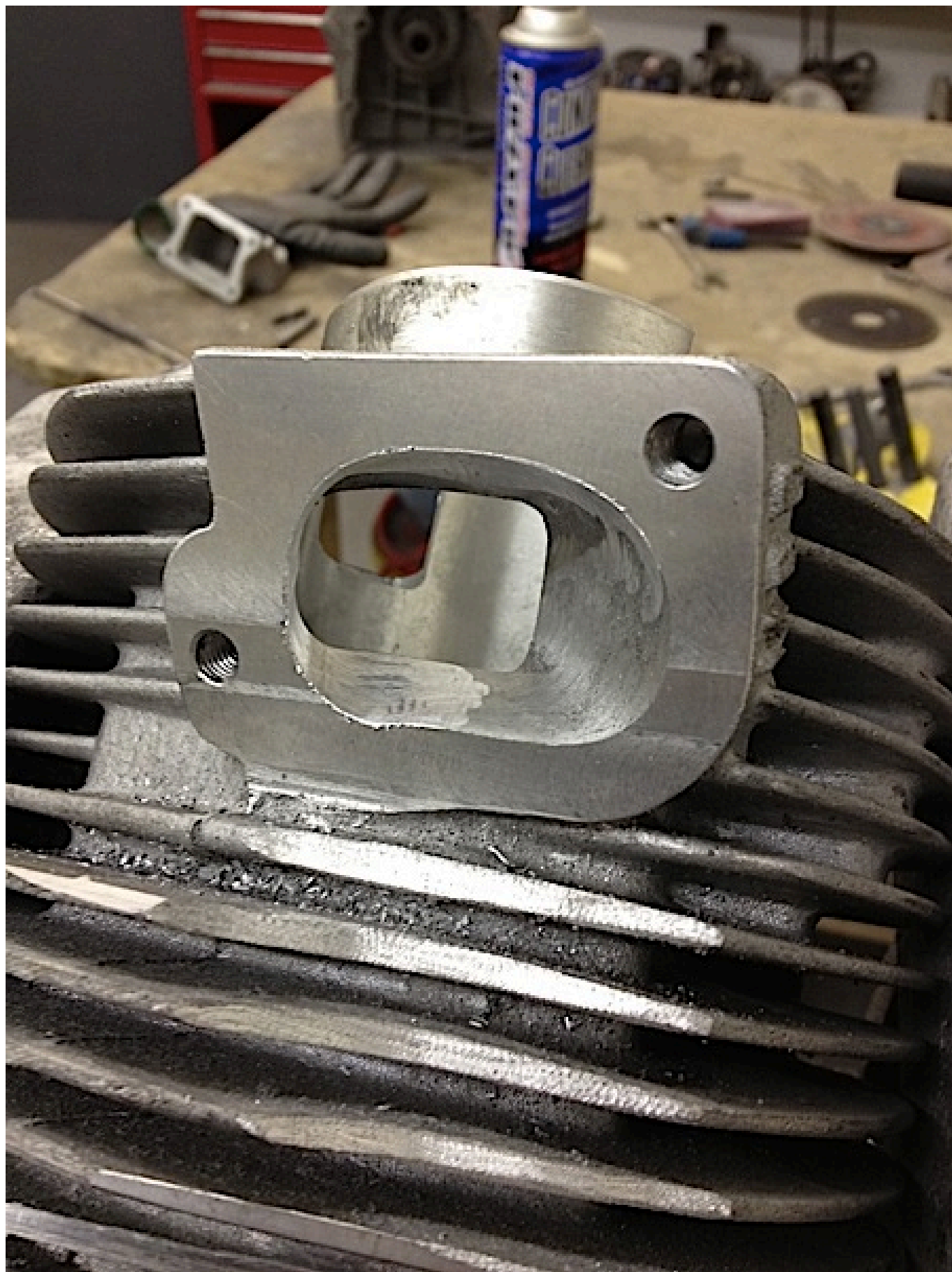
Mark out where the manifold is and cut the port to match
