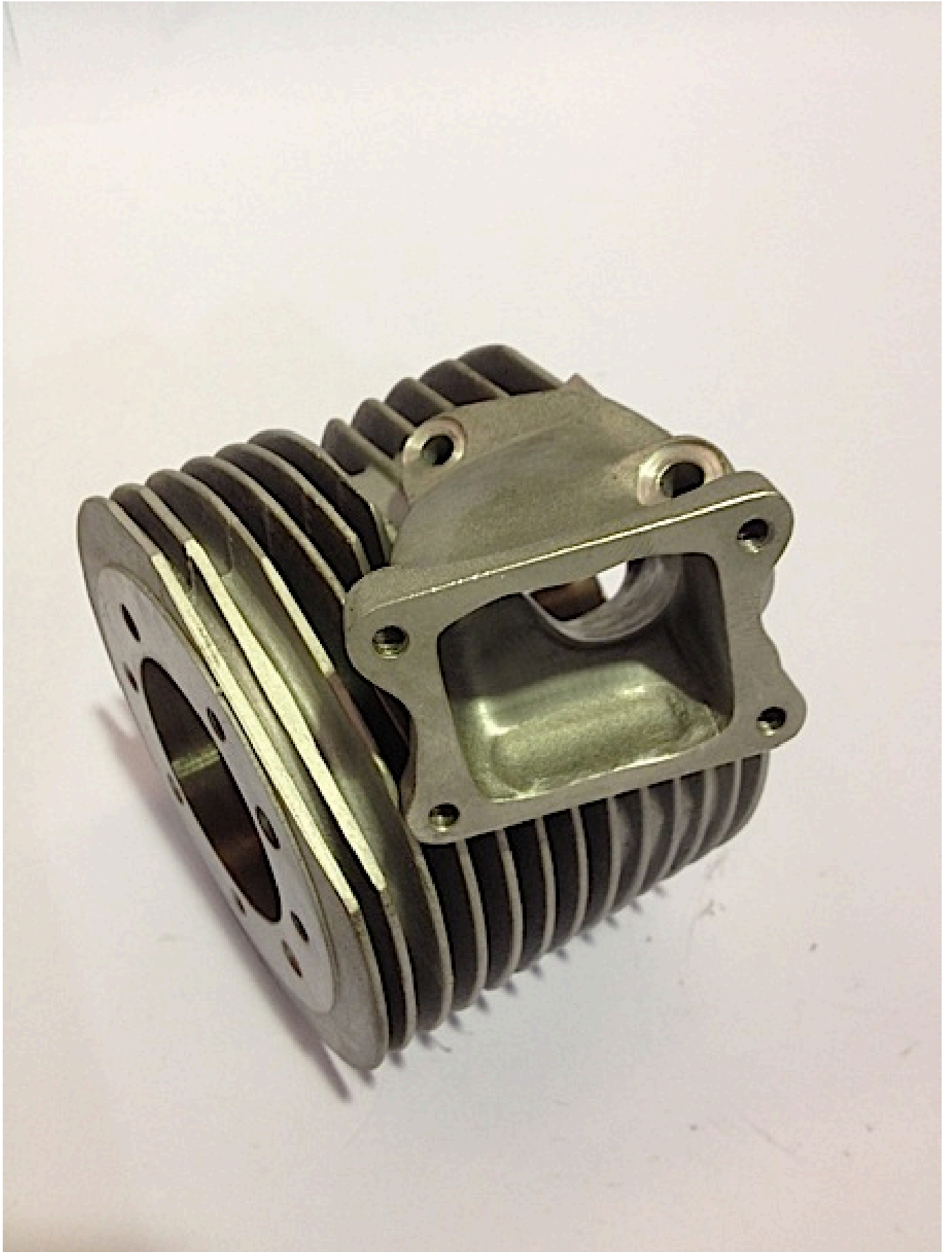
Finished Ceramic plated with Reed manifold flowed and matched
