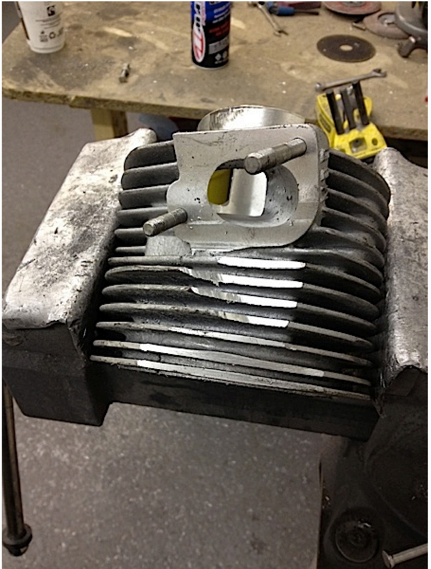
Top fins removed slowly to keep as much fin area as possible
