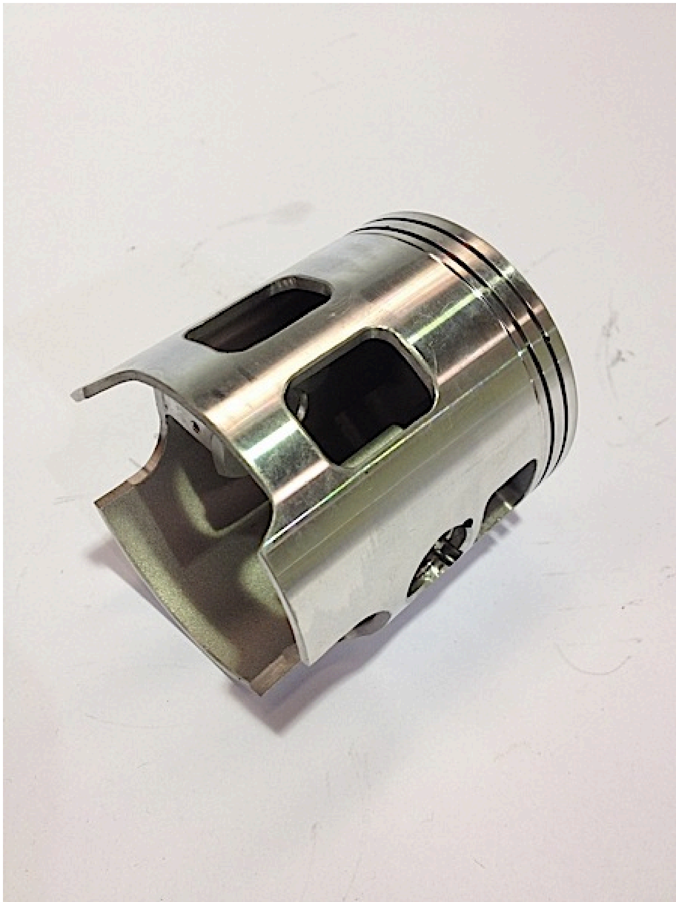
An MB RT piston port piston hand machined to suit reed 360 degrees inlet timing
