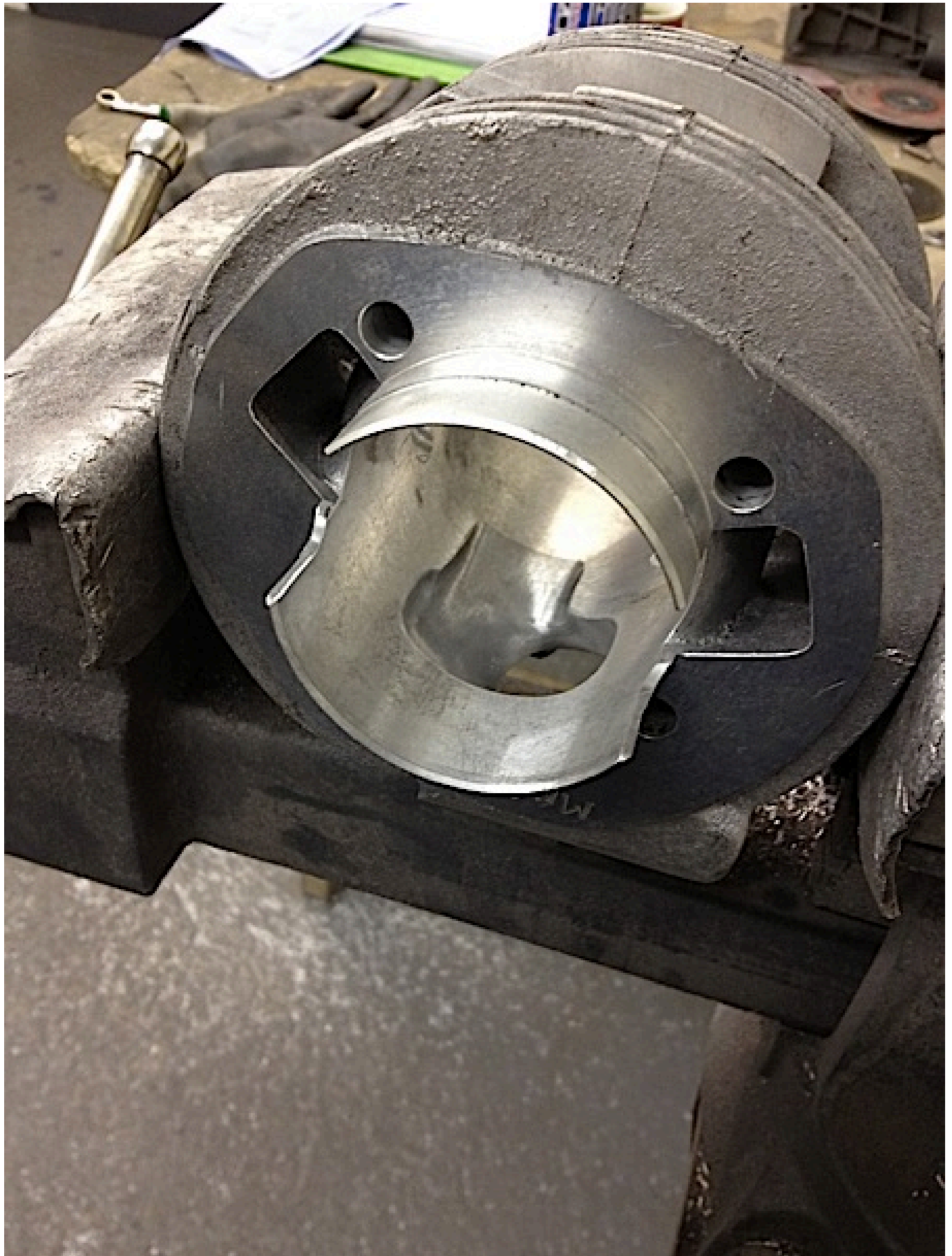
Boost port and new shape inlet port
