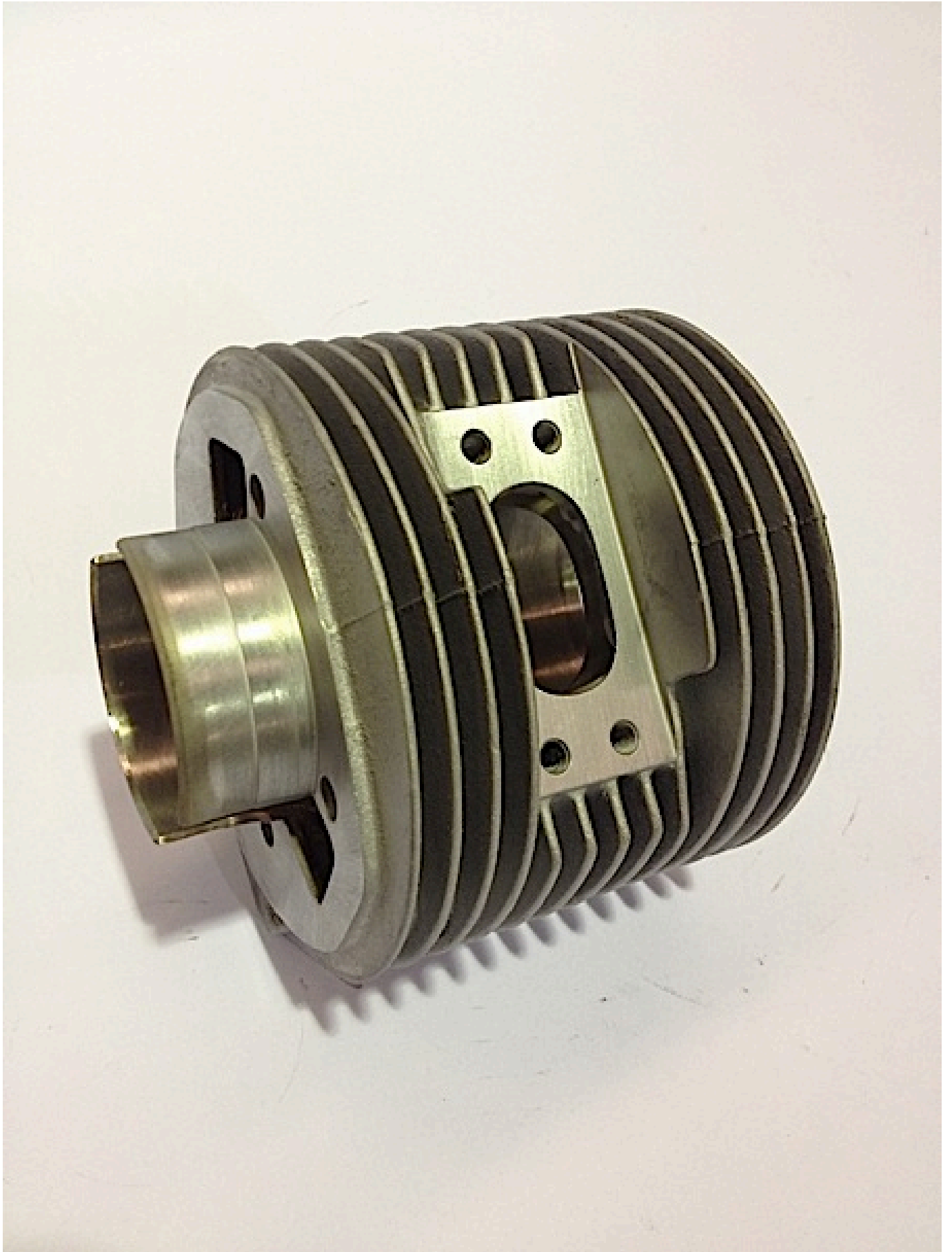
4 studded exhaust port only on an MB RT cylinder
