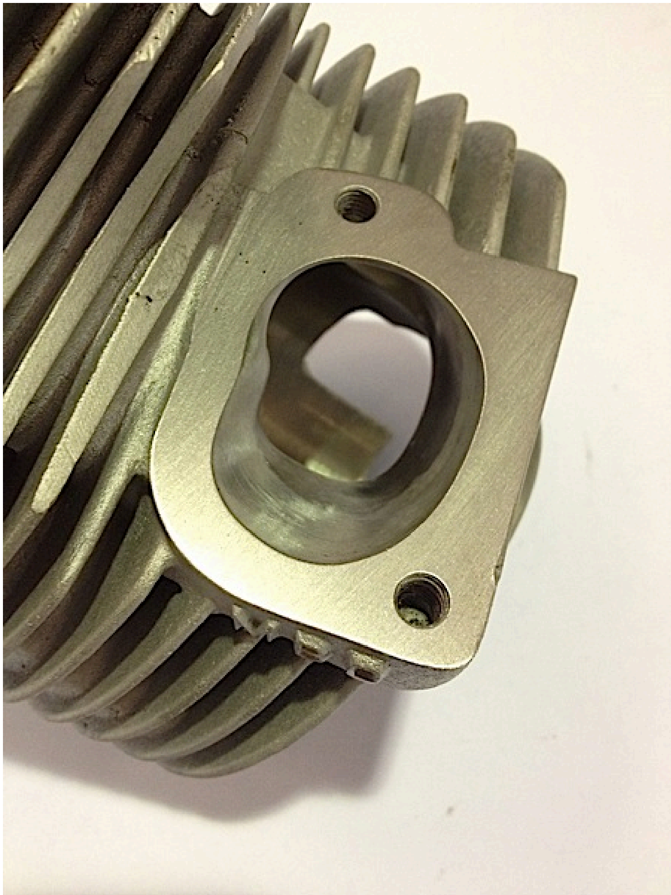
Inlet port after Ceramic plating, the plating always marks all the clean porting work and I re-flow it afterwards
