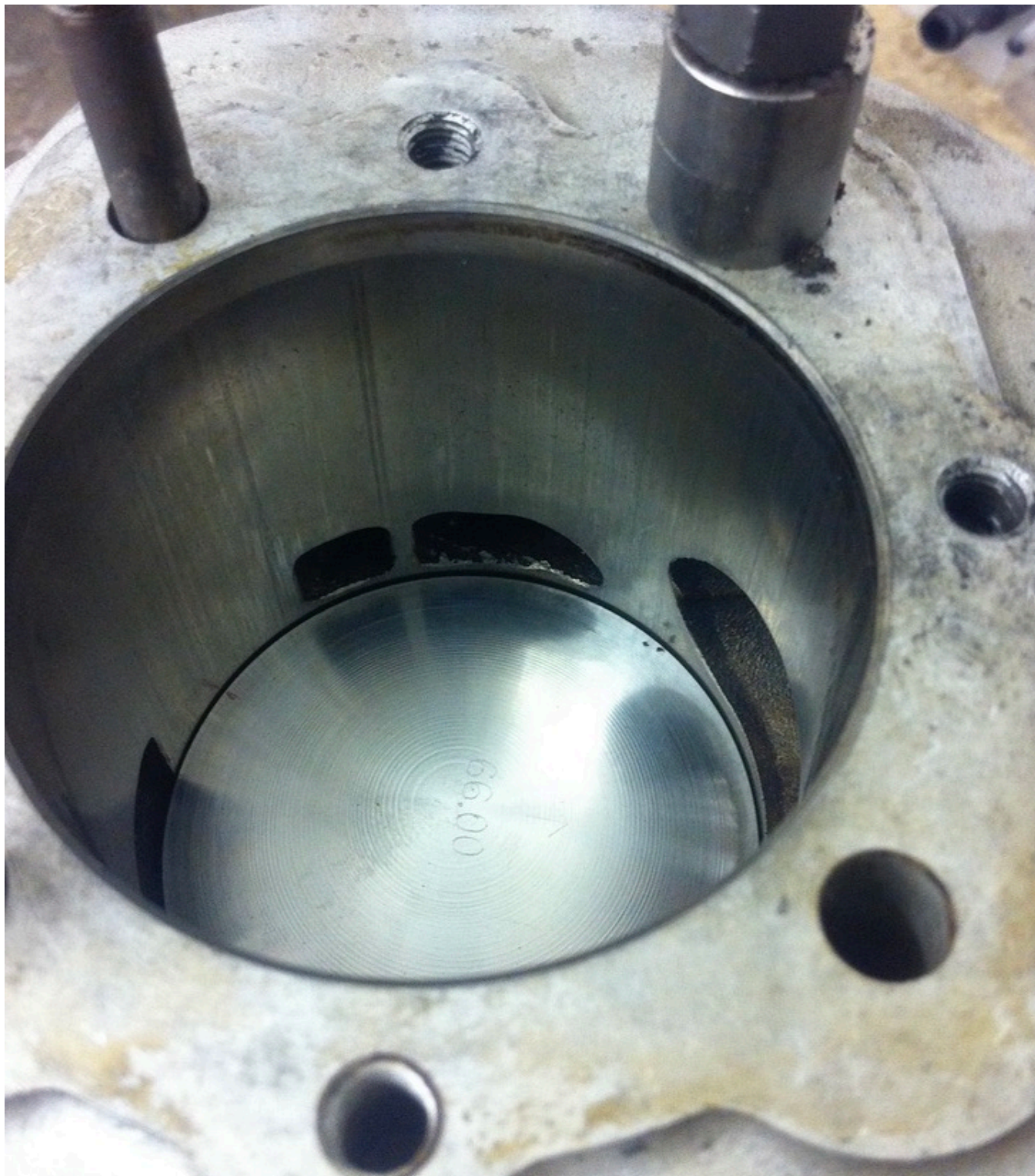
Later cylinders showing the split transfer feeds into the cylinder and the extra 7mm bolt holes to secure the head. Showing how poor the machining work is, note the exhaust port and transfers ports are not level at BDC
