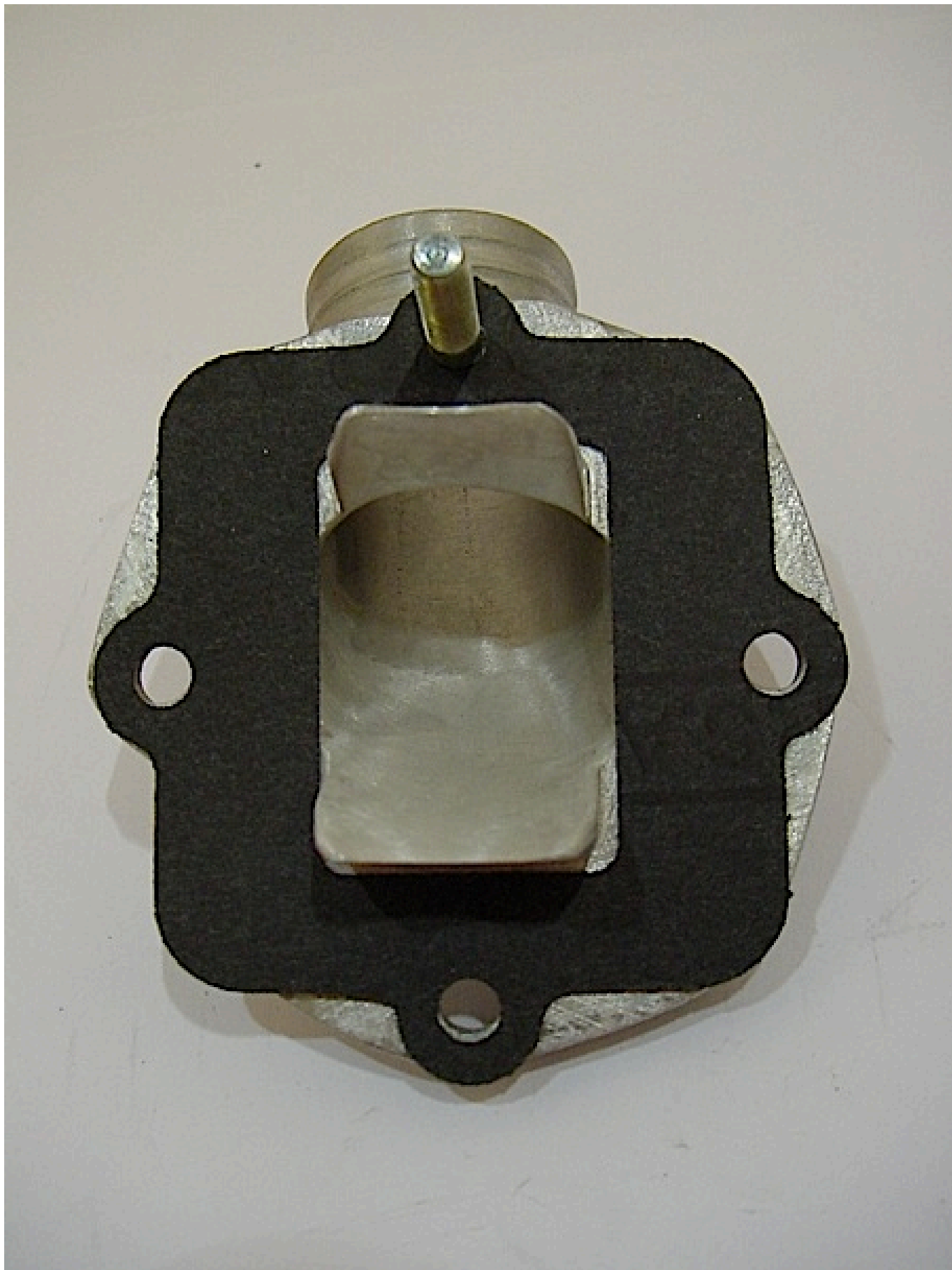
An MB inlet modified and thinned off around the area that fits into the small Honda Reed block of early Imola versions
