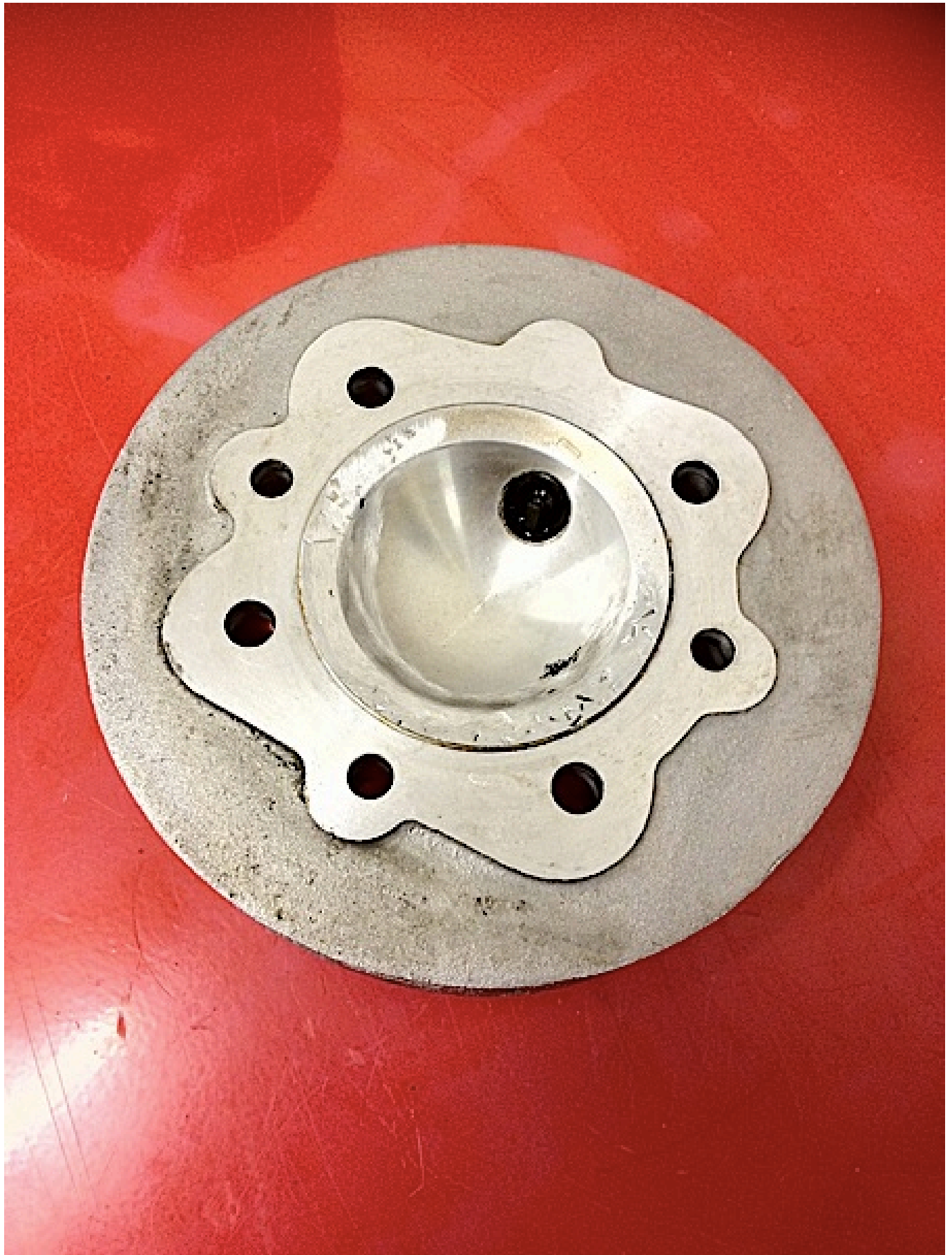
New type Imola head, cleaned up after a big end failure, note 3 extra bolt holes using 7mm studs and note the drop into the bore
