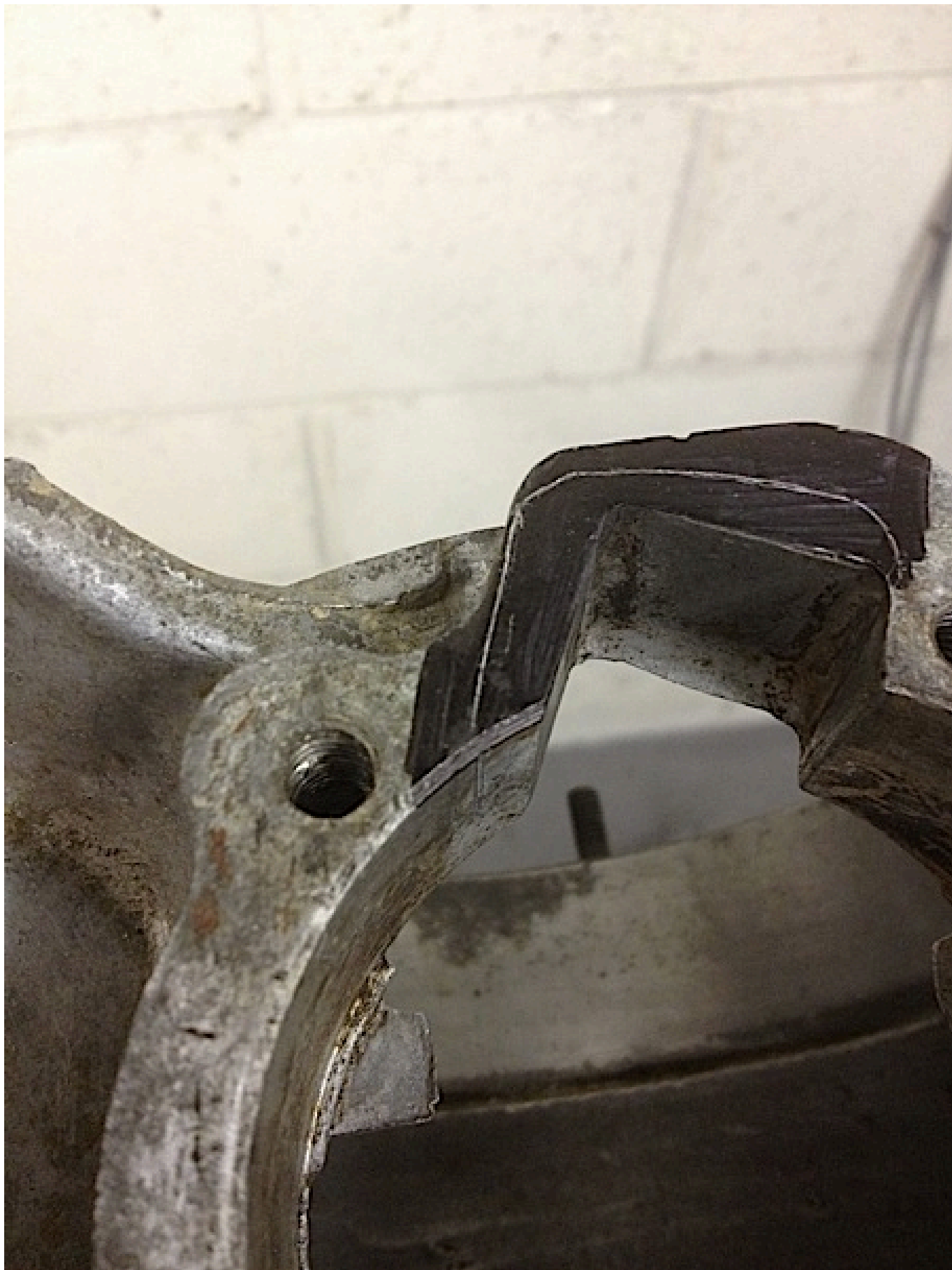
Some Imolas are so far out they can draw air through the casings as shown here
