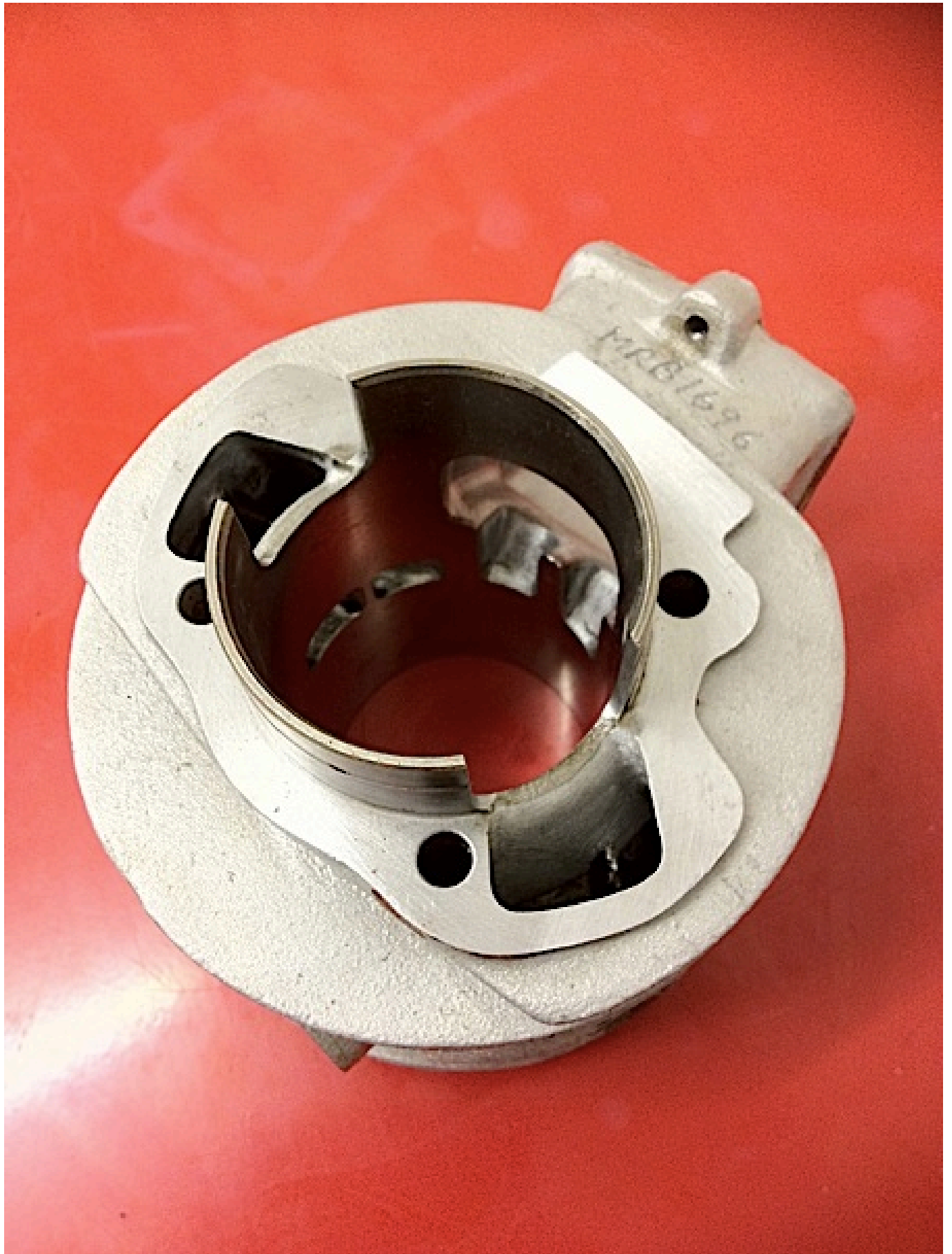
Later Imolas with two boost ports above the inlet
