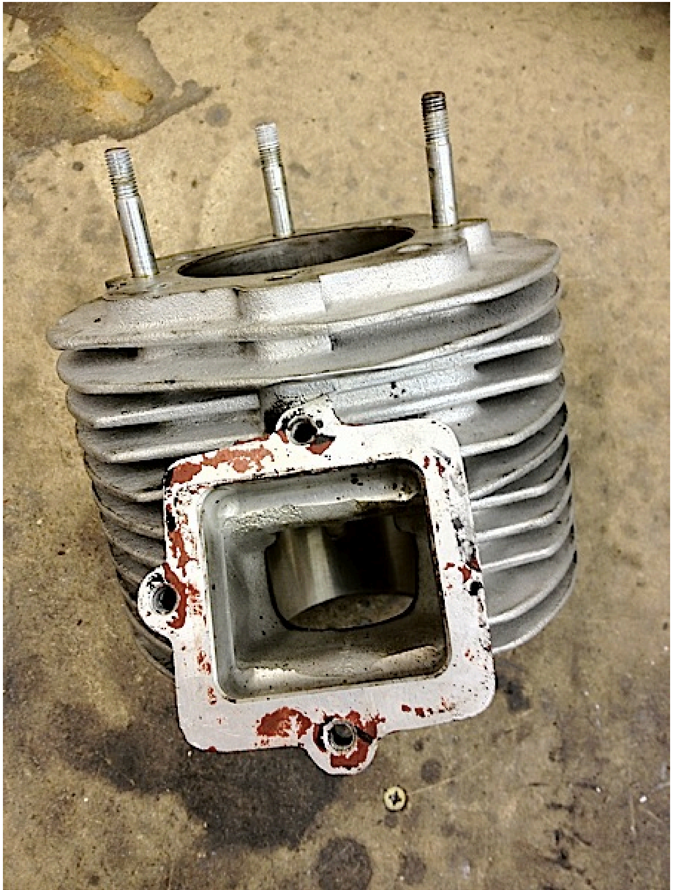
Later Imolas with 3 stud holes on the inlet manifold face with either 3 or 4 extra bolt holes for the head
