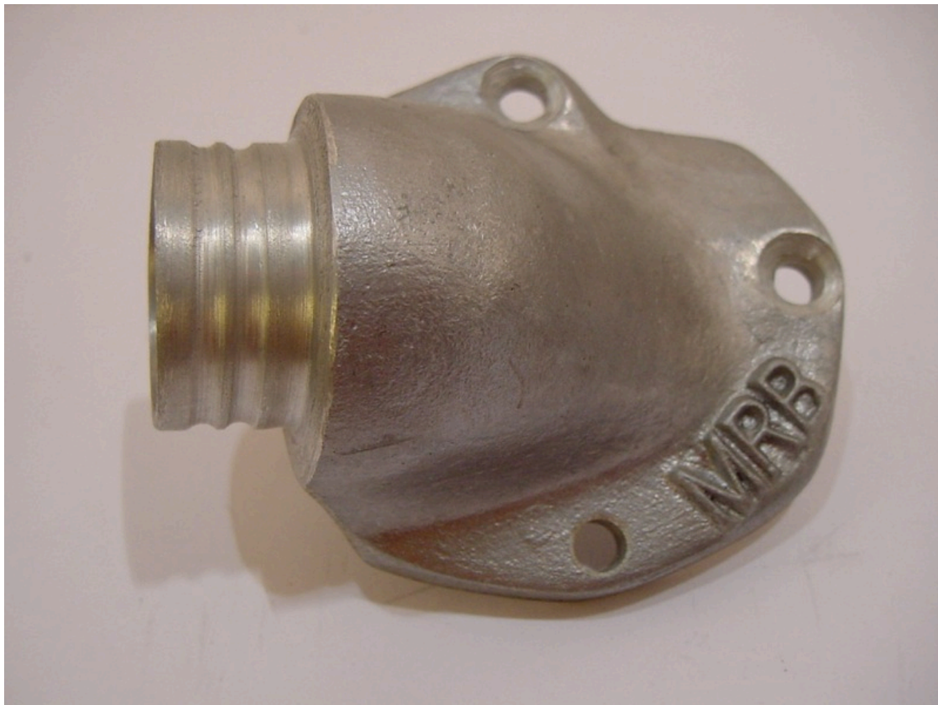
The MB 30mm TS1 inlet manifold machined to suit 30mm Dellorto and PWK mounting rubbers
