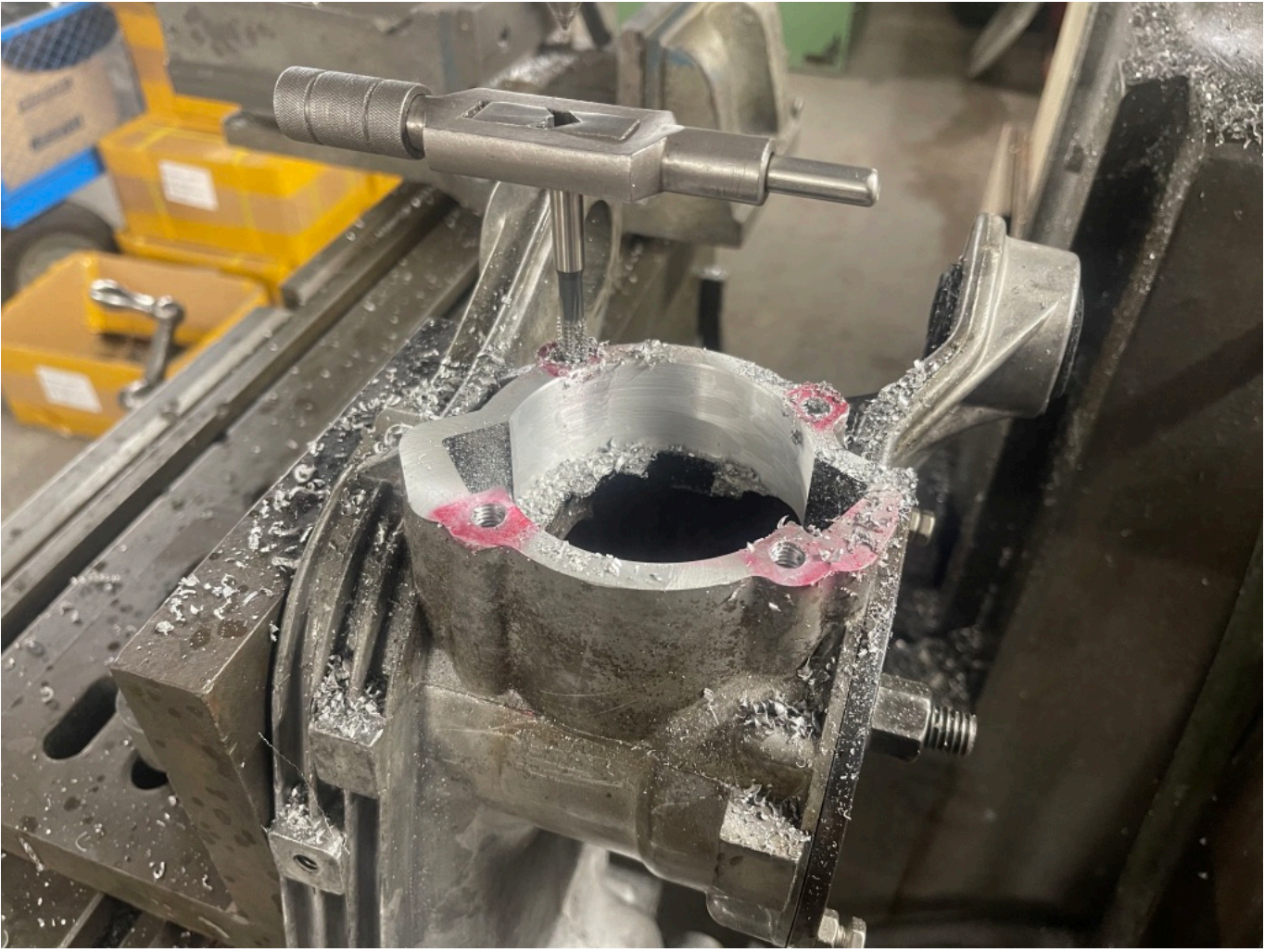
Set up, face off, bore out, drill and tap new Large block stud spacing
